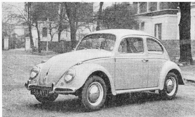
VOLKSWAGEN: The immensely popular Volkswagen, which has been manufactured basically unchanged for many, many years now. It is powered by an air-cooled, four-cylinder 1,192 c.c. engine.
