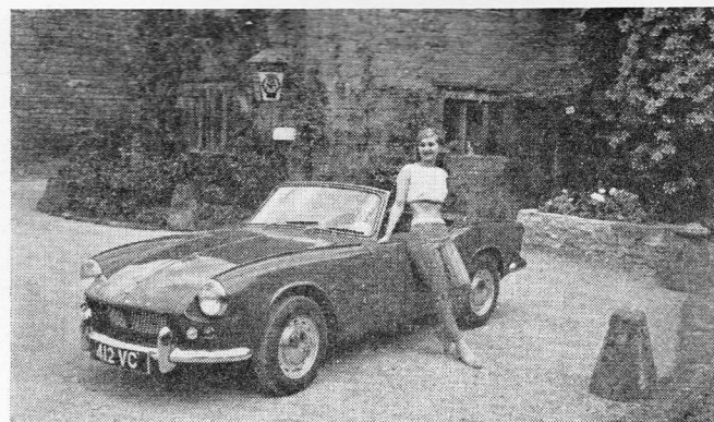
TRIUMPH: The new Triumph Spitfire sports car (above) is powered by a four-cylinder 1,147 c.c. engine developing 63 b.h.p. at 5,750 r.p.m. Independent suspension is featured. TRIUMPH: The TR4 sports car (below) has either a 2-litre or a 2.2-litre engine.
