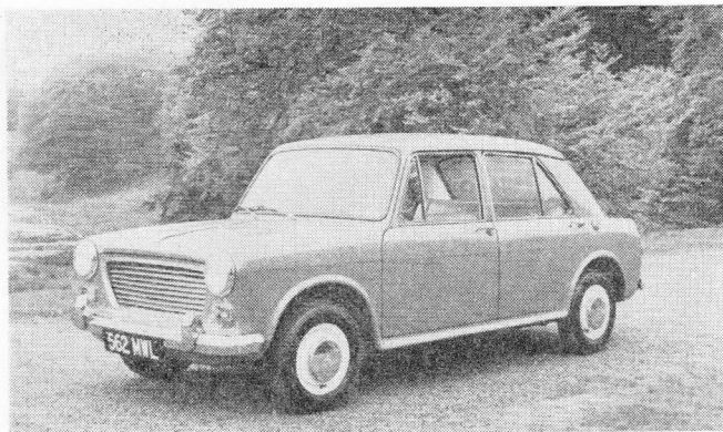
MORRIS: The 1962 Alec Issigonis wonder is the Morris 1100, featuring a transverse engine, front-wheel drive, independent suspension, the unique Hydrolastic suspension and disc brakes at the front.
