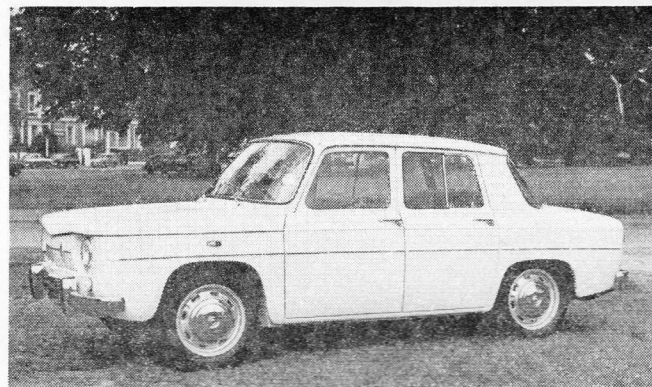
RENAULT: The four-seater Renault R8 (above) has disc brakes on all four wheels, a five-bearing 956 c.c. engine developing 48 b.h.p. and a sealed engine cooling system. RENAULT: The Renault Floride Caravelle (below) also has the five-bearing engine and disc brakes.
