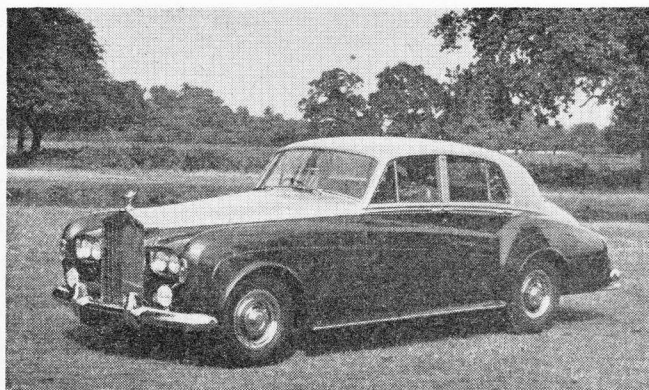
ROLLS-ROYCE: The Silver Cloud III four-door saloon now has improved performance and improved fuel consumption since the compression ratio of the V8 6,230 c.c. engine was raised from 8 : 1 to 9 : 1.
