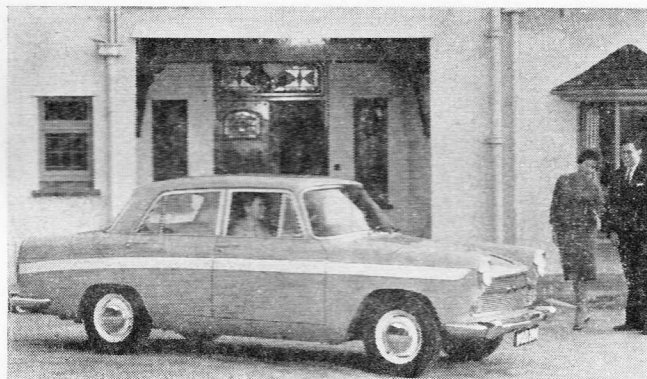
AUSTIN: The A60 Cambridge saloon (above) is powered by the B.M.C. B-type engine of 1,622 c.c. AUTO UNION: A revolutionary new system of automatic oil injection into the fuel at the carburetter is available as standard equipment on the f.w.d., three-cylinder 1000S coupé (below).
