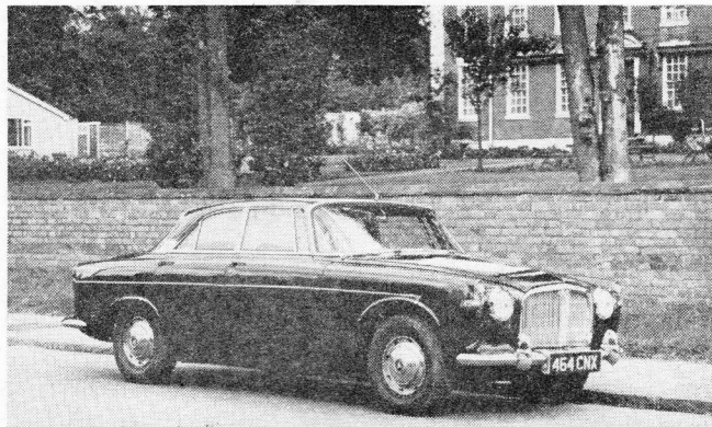
ROVER: The Rover Three-Litre Coupé was introduced to the range recently. The power output is 134 b.h.p. at 5,000 r.p.m. and the car is capable of speeds well in excess of 100 m.p.h.
