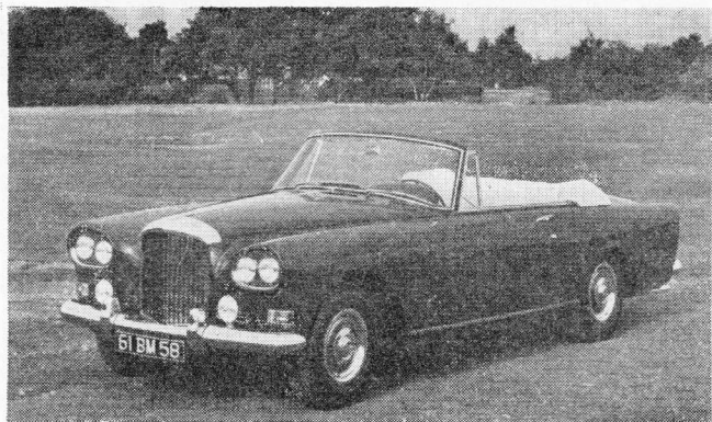
BENTLEY: The S3 Continental drophead coupé with coachwork by Park Ward. The engine of this finely appointed sports car is the V8 6,230 c.c. unit. Note the new twin headlamps.
