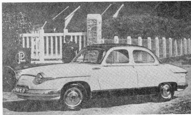
PANHARD: The Panhard PL17 features air-cooling, a two-cylinder 850 c.c. engine, front-wheel drive and represents remarkable performance and economy.
