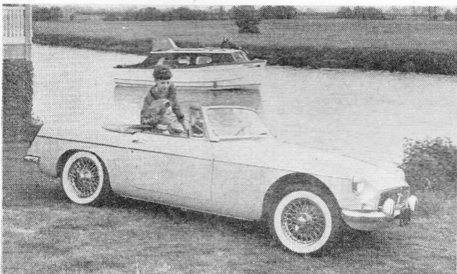
M.G.: The M.G.B. is developed from the very successful dollar-earning M.G.A. It has a four-cylinder, 1,798 c.c. engine, winding windows, an occasional rear seat and front disc brakes.
