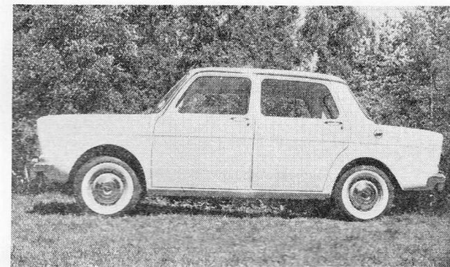
SIMCA: This rear-engined 944 c.c. car (above) has independent suspension all round. The Simca 1000 has a top speed in the region of 75 m.p.h. SINGER: The Singer Vogue (below) is another Rootes car of well above average quality and workmanship.
