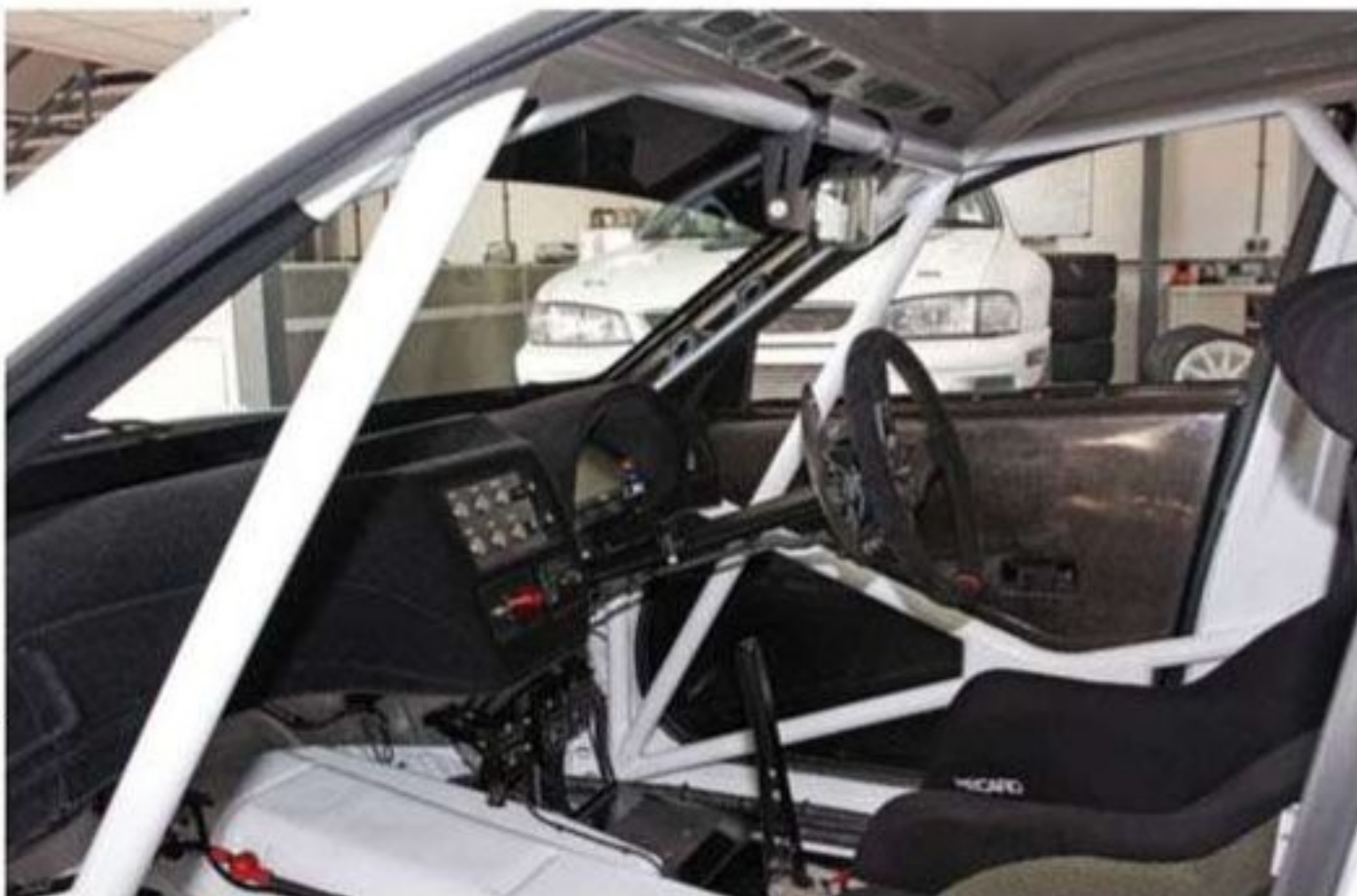
The roll cage - created by Custom Fabrications - provides most of the car's strength and stiffness
