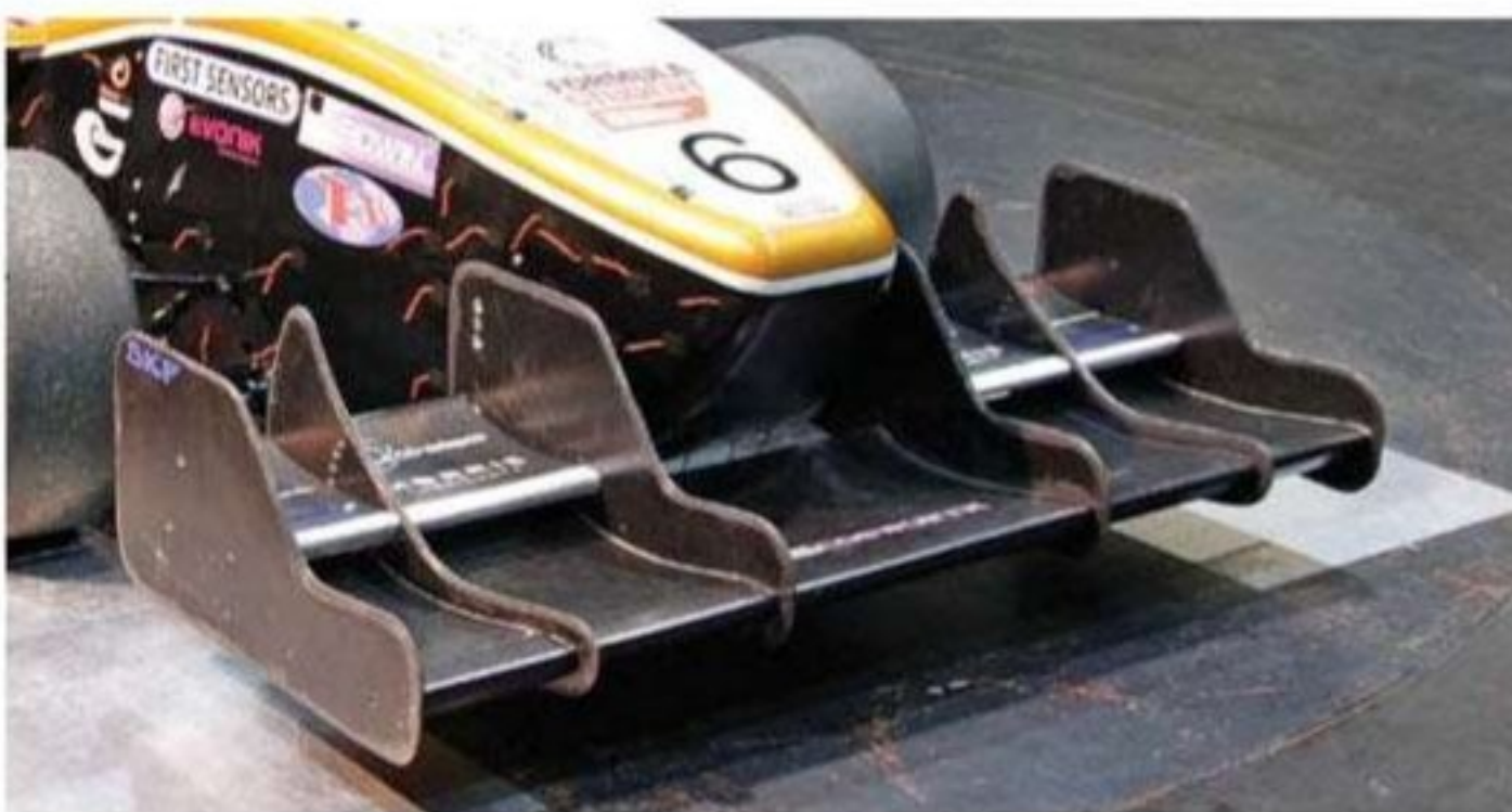
Minimum inner and outer front flap angle
