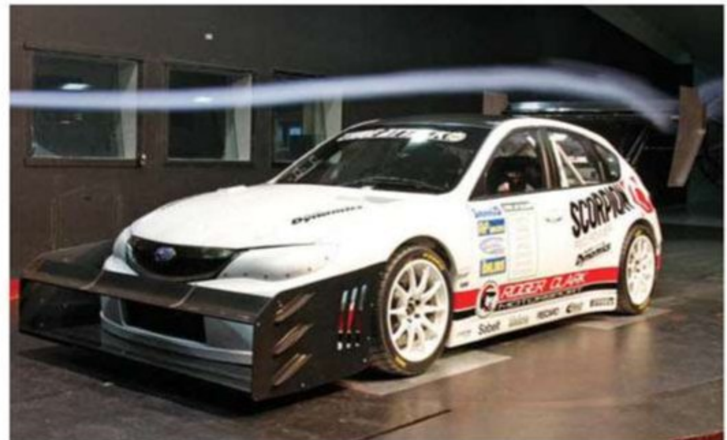
Wind tunnel testing revealed all, including the rear wing's induced downwash
