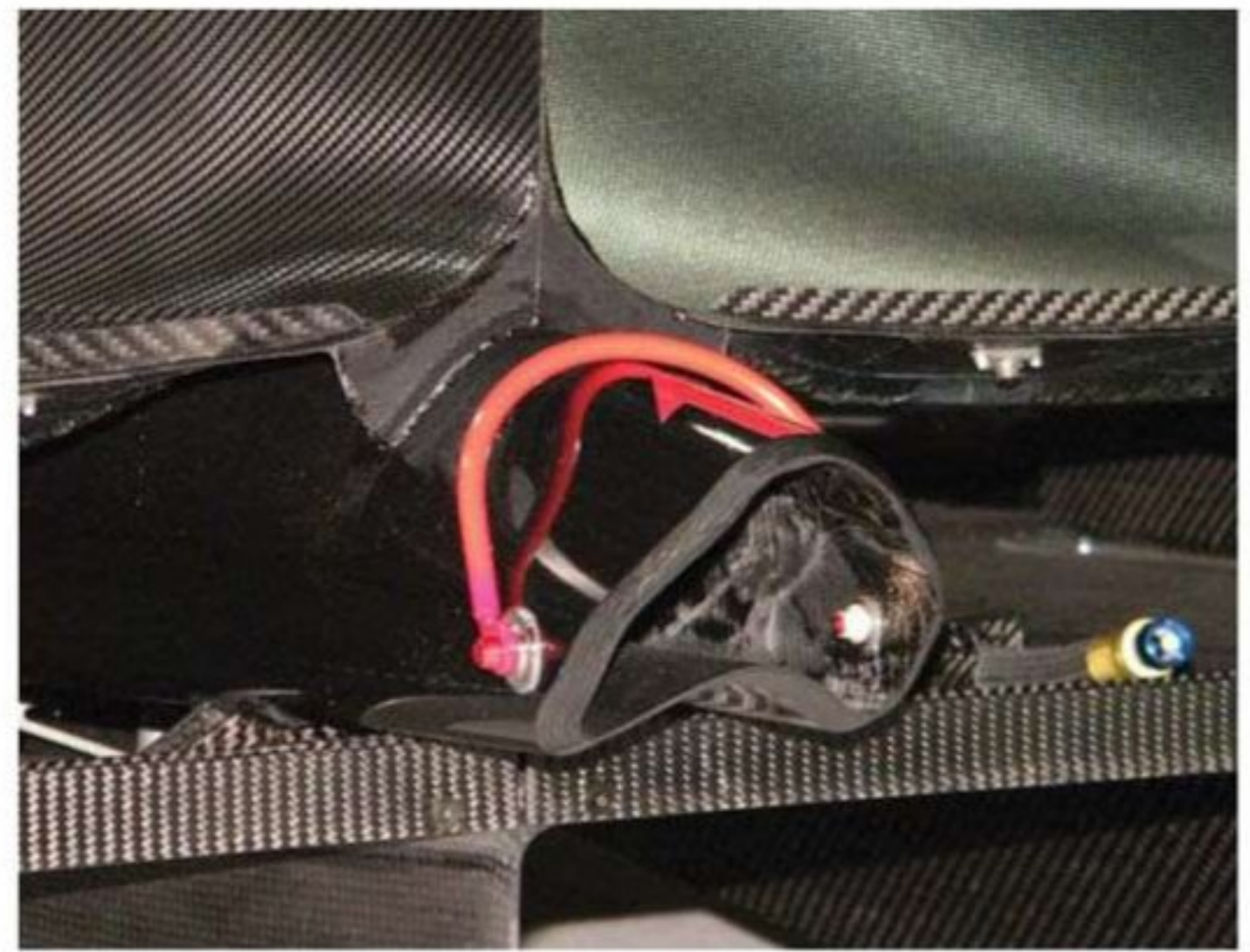
Larger crash structures are required in the new regulations, and in the case of the new R18, this extends beyond the end of the rear bodywork
