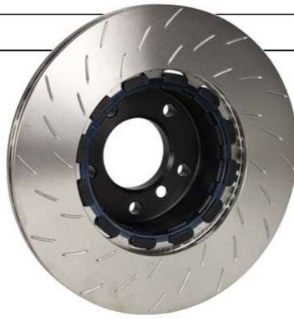
V3 disc retention technology from PFC, which requires no torque wrenches
