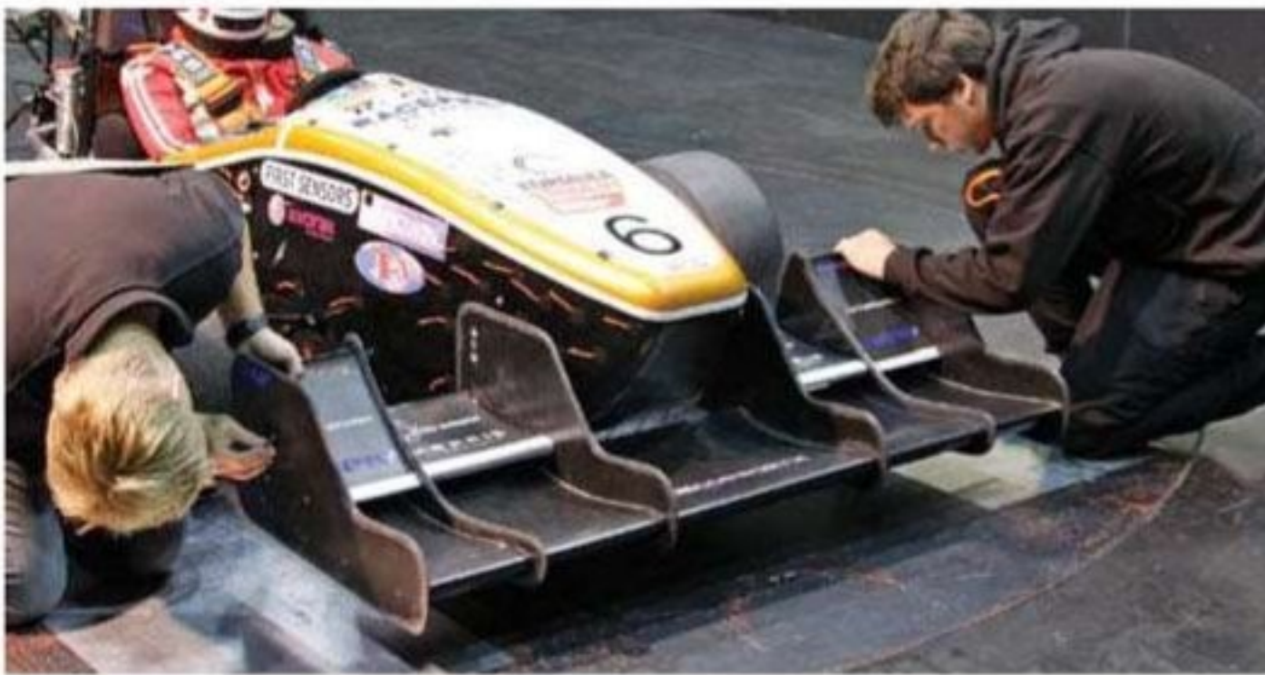
Minimum inner and maximum outer front flap angle
