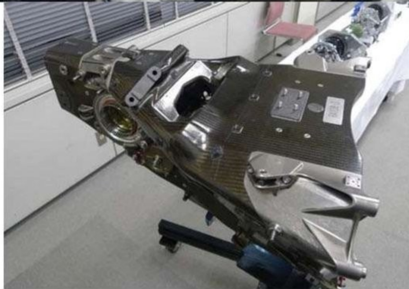
Top: the original seamless shifting concept from 2008
