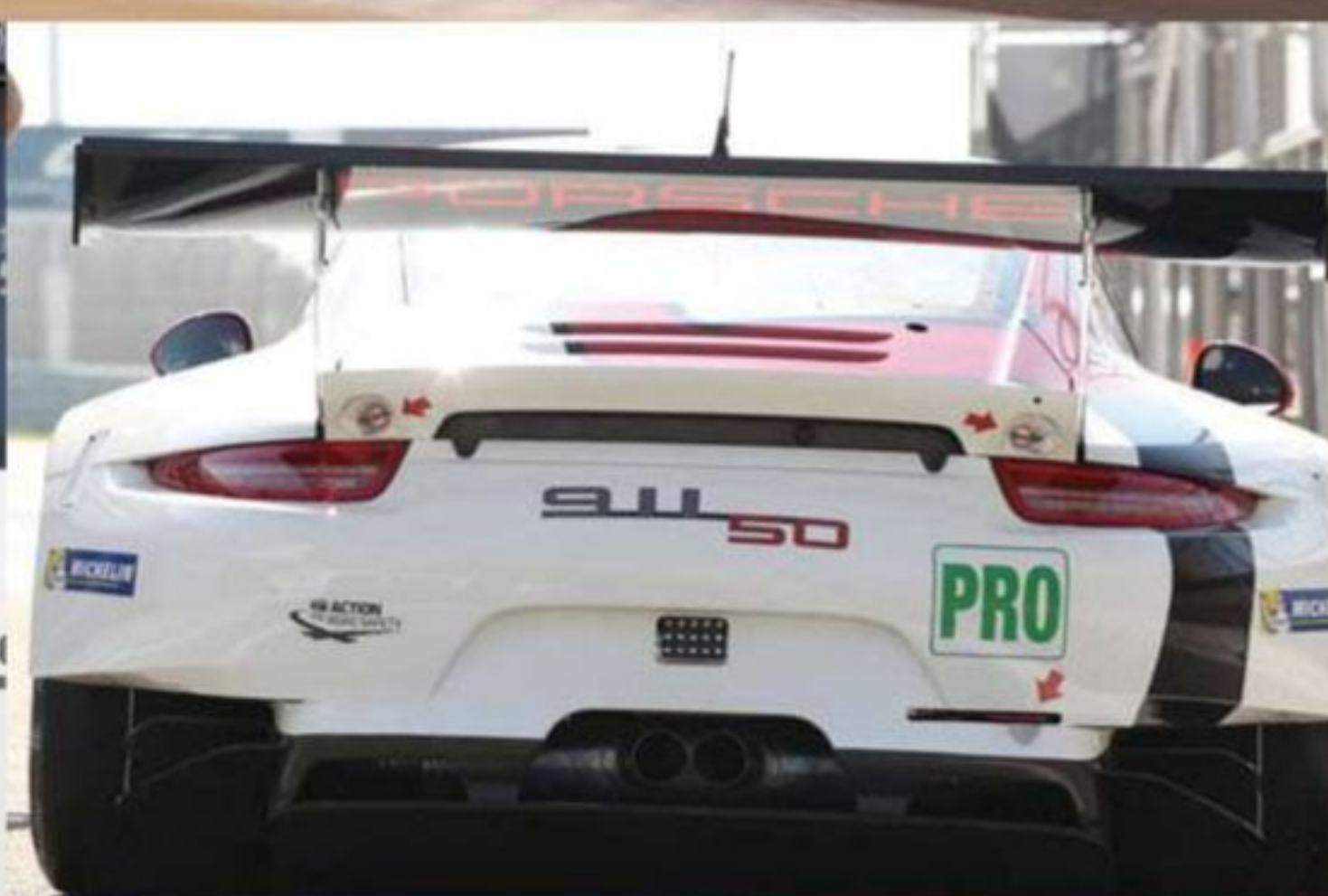
Wider rear wing and wider rear rims were crucial to managing the rear tyre wear on the 991. Waivers were needed for both
