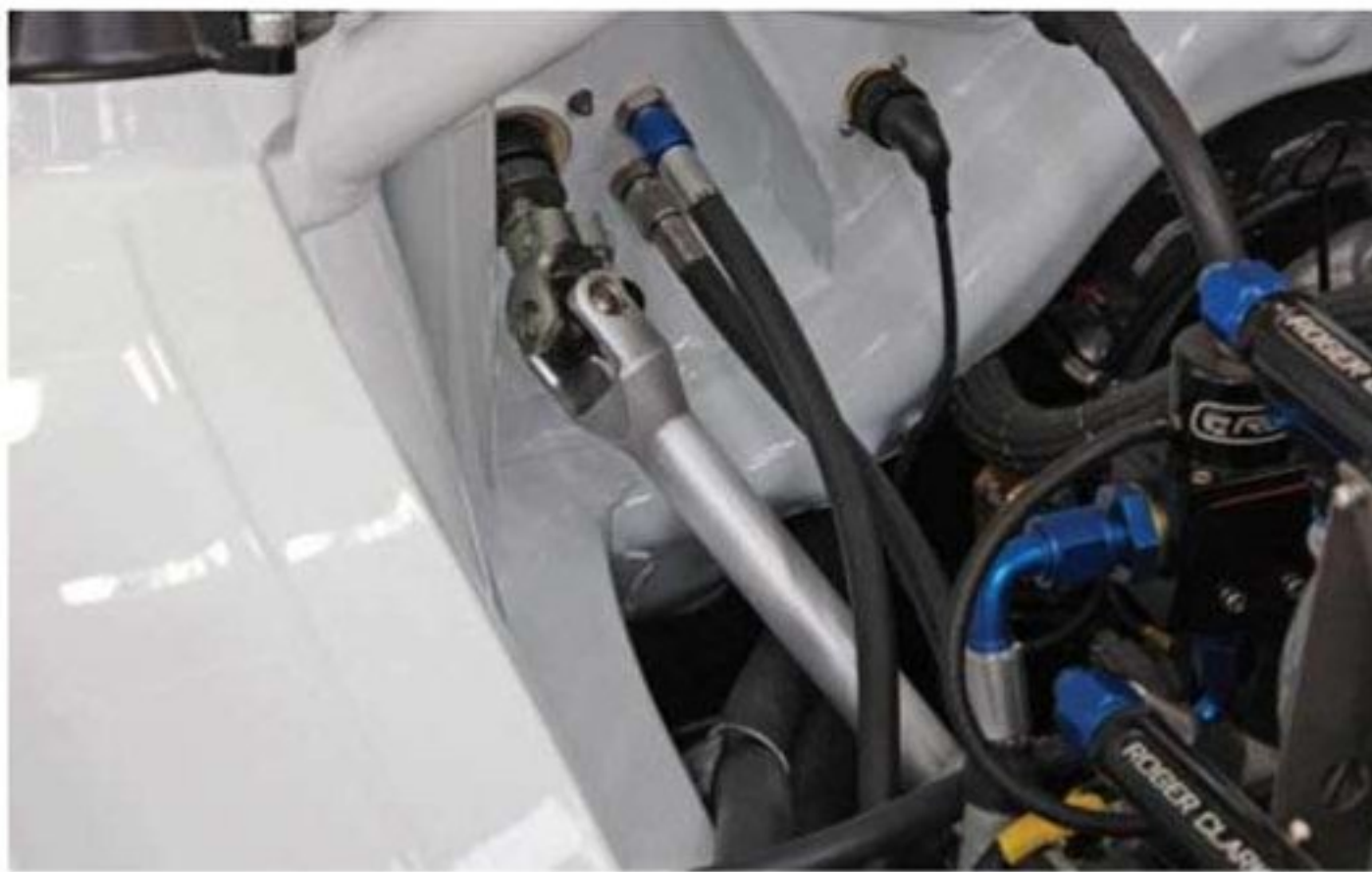
The visible steering column on the right-hand side demonstrates that the turbo has been moved to the left
