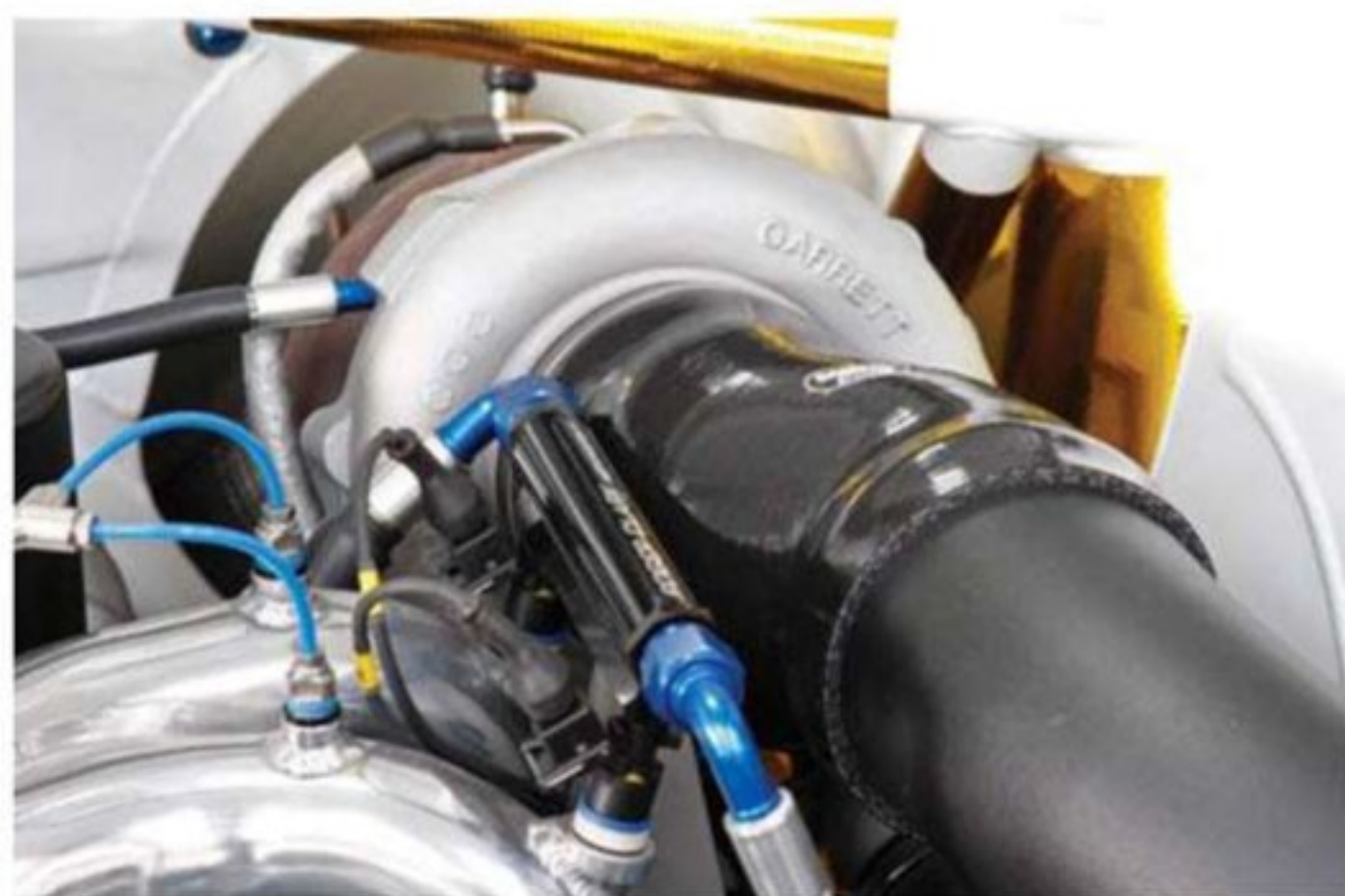
Garrett GT4094 hybrid twin scroll turbo, big for a 2-litre engine - normally
