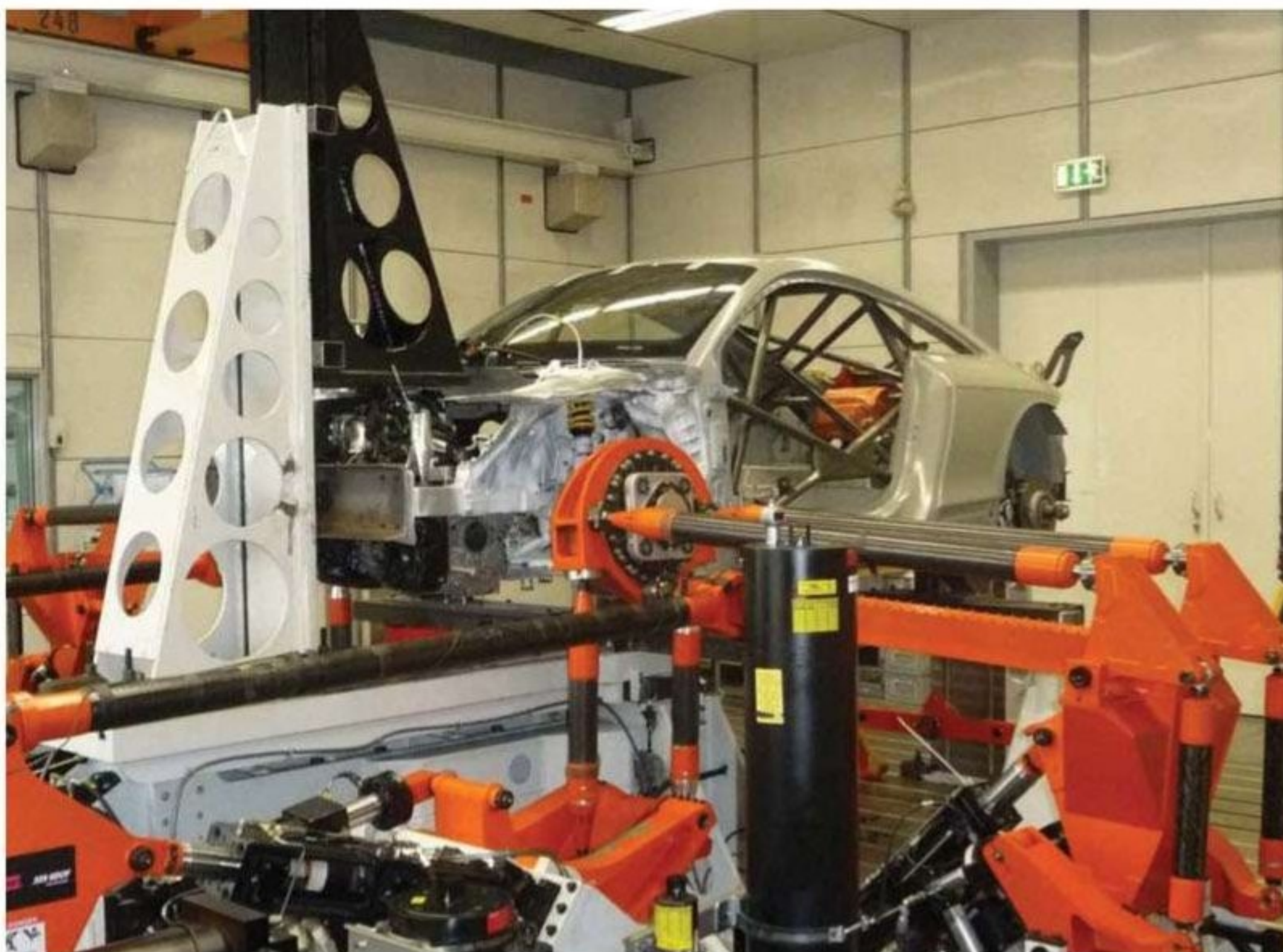
The front axle on the test rig. The input data came from measurements derived from Nürburgring and Oschersleben
