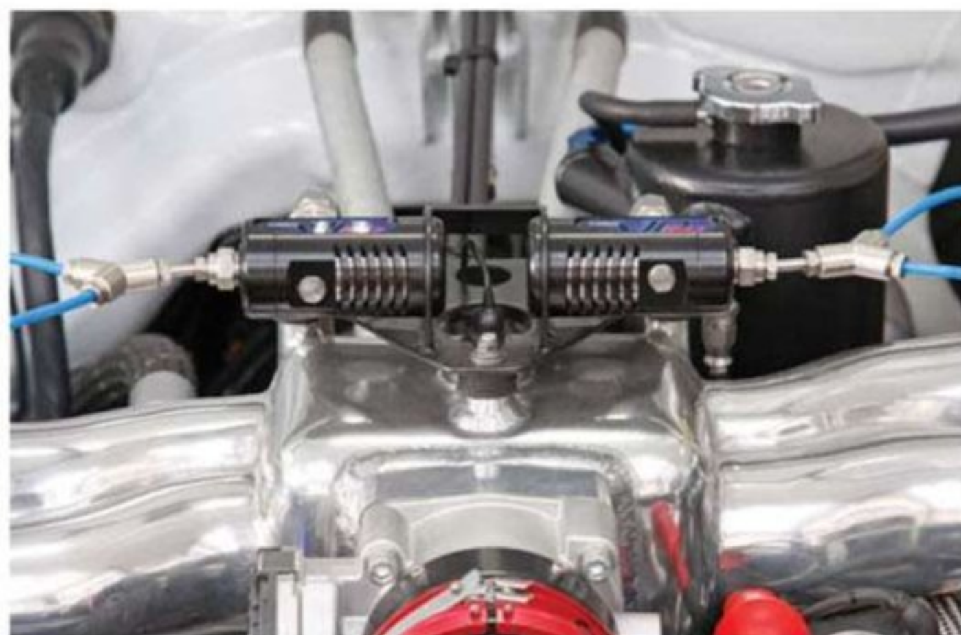
The progressively controlled nitrous oxide injection system helps match the big turbo to the 2-litre engine
