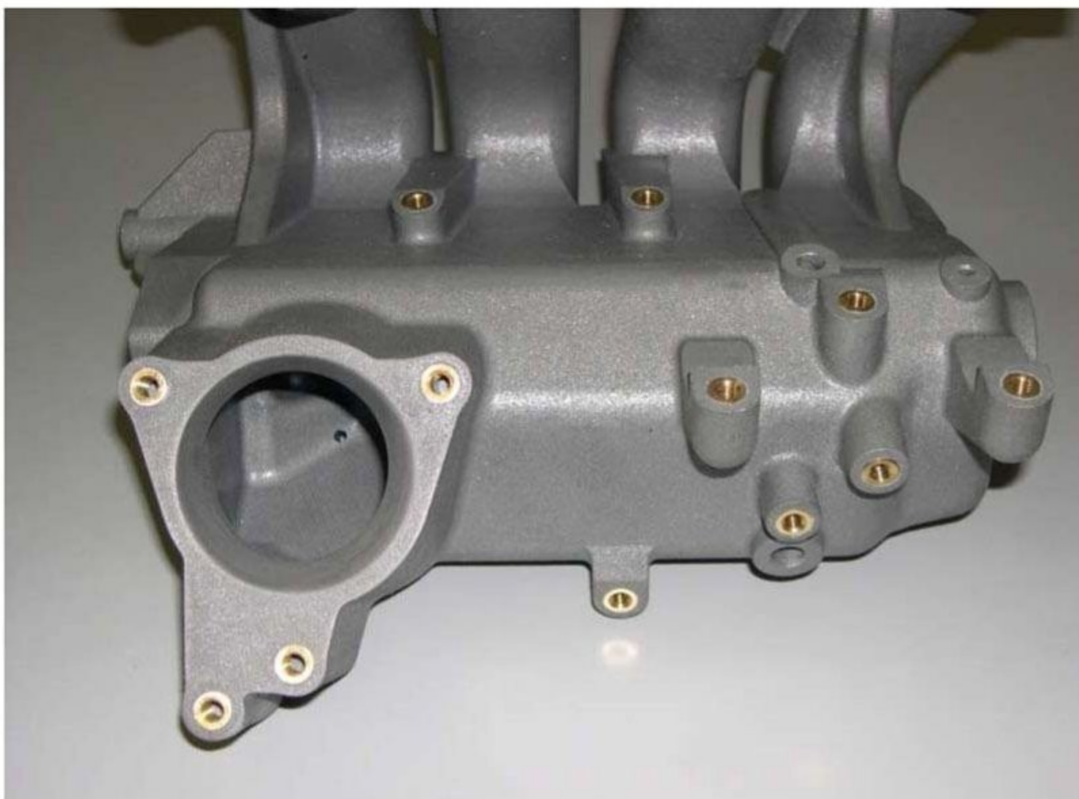
Close-up view of the 3D printed intake manifold, featuring threaded bushings
