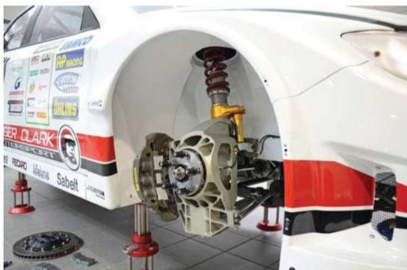
RCM billet alloy uprights and Ohlins TTX46 struts
