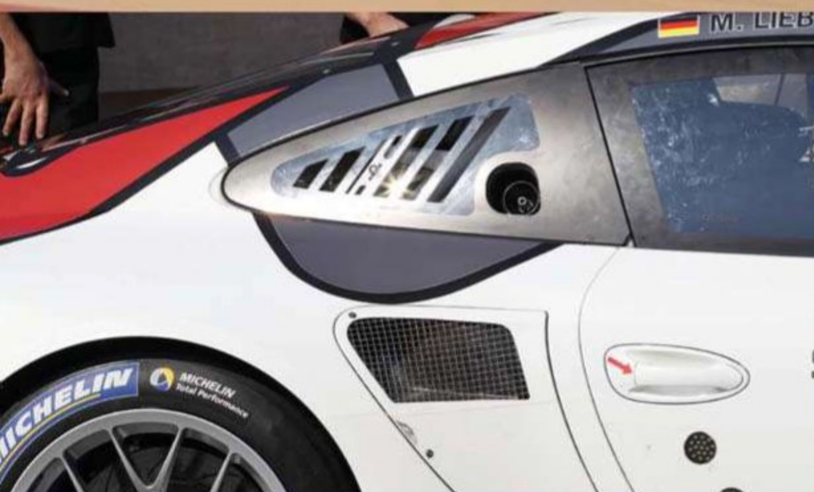
New air intakes for the engine may have slightly increased power, but not enough for engineers to start boasting
