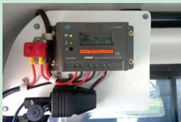
Left: Solar Regulator fitted to a solar system in a canopy. Note the Load Circuit is feeding directly to the cig socket.
