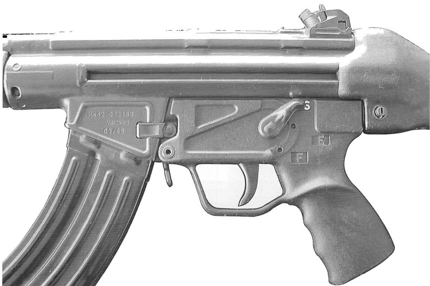
450. Left side closeup of HK32 serial no 012169, manufactured in September, 1969. H&K collection, courtesy Dieter Rall
