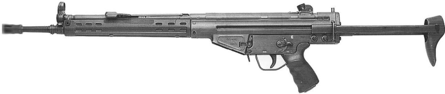
558. Left side view of the Turkish G3A4, manufactured by MKE, with retractable stock extended.
