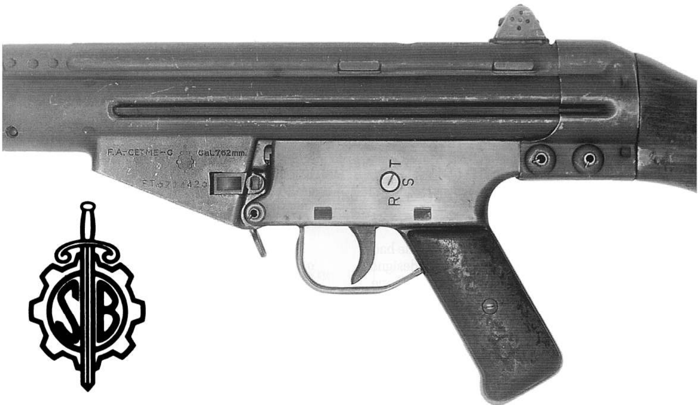
603. Left side closeup of the interim "Model 1958-64-C", marked "F.A.-CETME-C Cal. 7,62mm", serial no E.T. *71442*, manufactured by Empresa Nacional Santa Bárbara, with selector still on the right side. Note the first appearance of the four-way flip-over rear sight, which has been relocated to the rear of the receiver.
