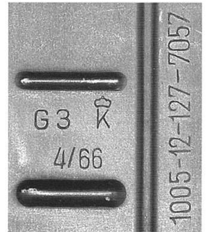
698 (right). A closeup of the aluminum magazine in fig 697, showing markings indicating manufacture by Kongsberg arsenal in Norway in April, 1966, but marked with an NSN with country code 12 (Germany).
