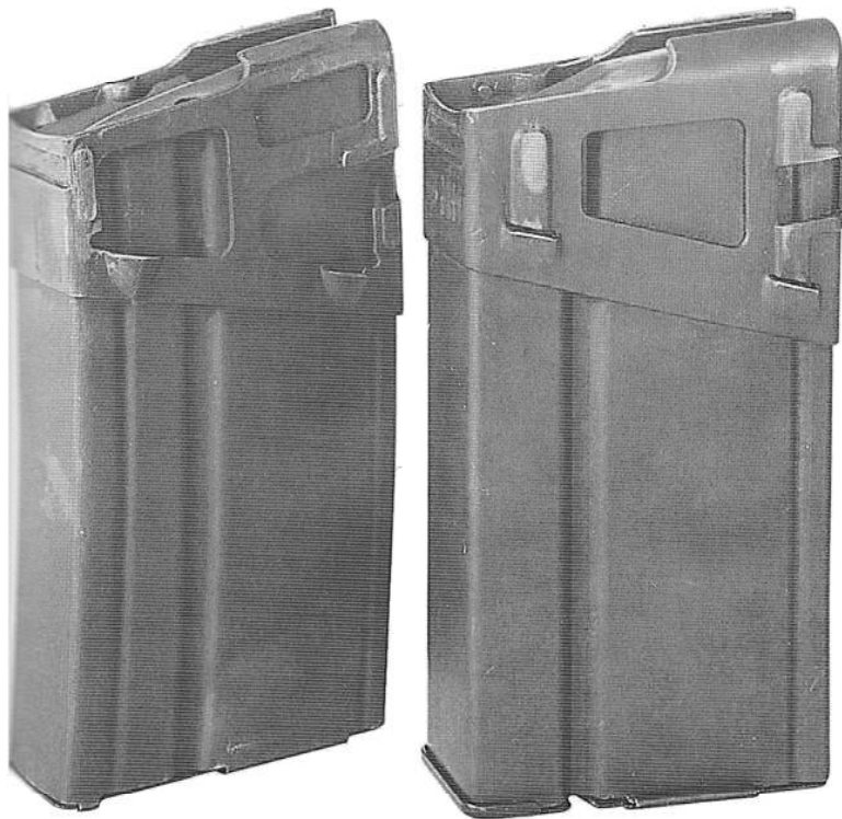
696. A comparison of two styles of steel 20-round magazines for the G3 rifle.
