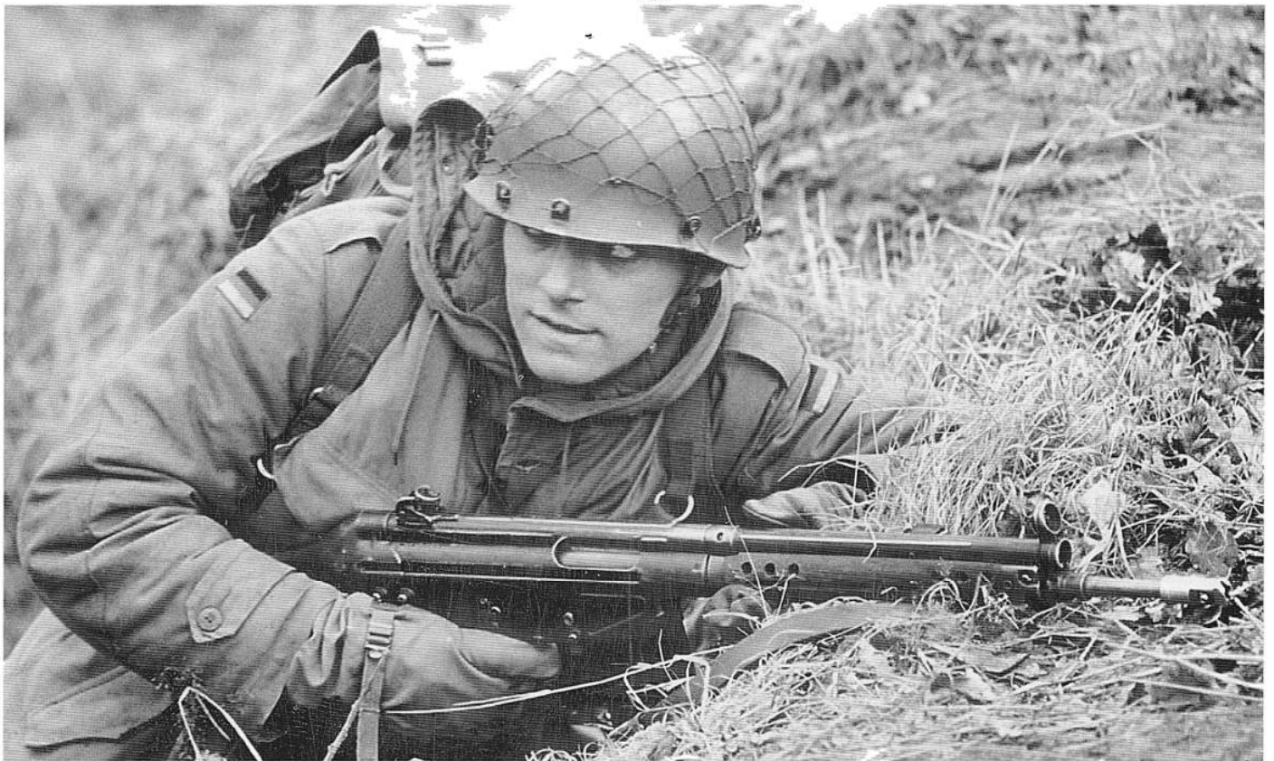
692. A German soldier on exercises. His G3 rifle, with wood handguard, is fitted with the version of the blank firing adapter (BFA) shown in fig 693.
