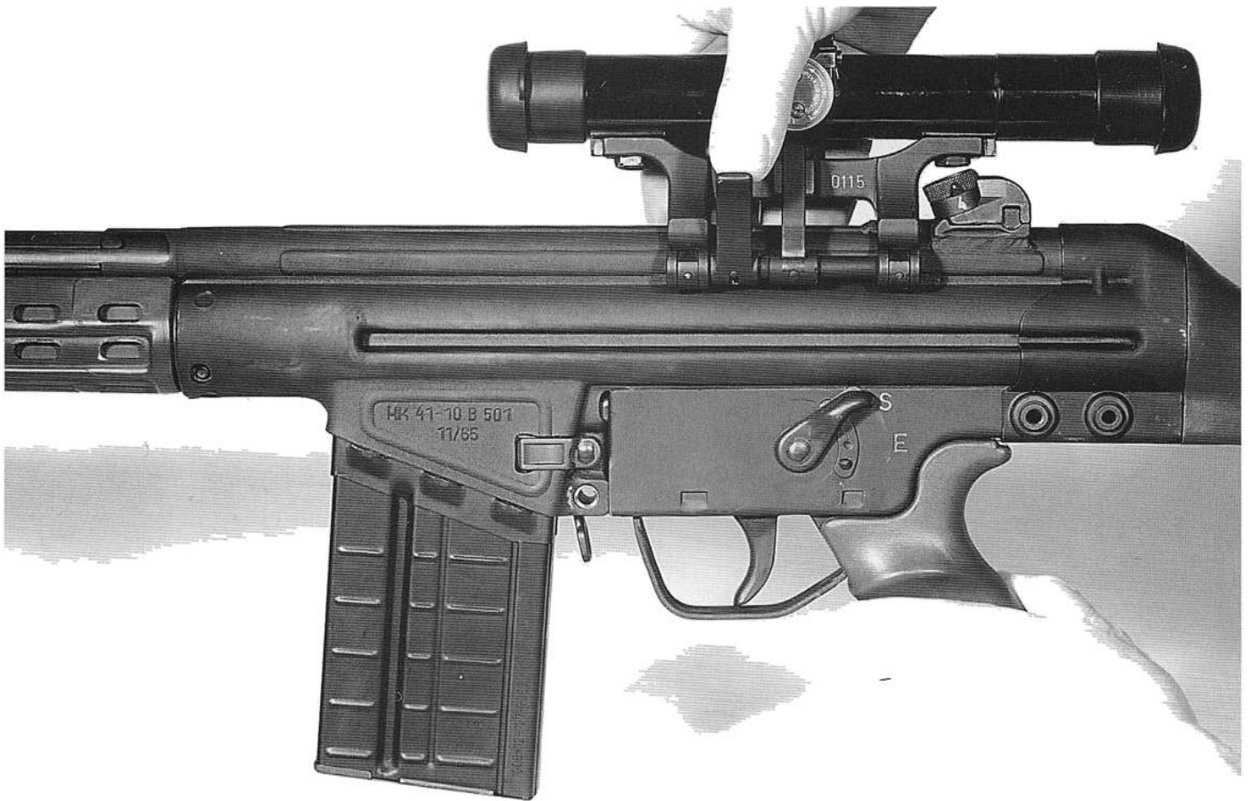
717. Left side closeup of an HK41 marked "HK41 - 10 B 501", dated November, 1965, showing the method of locking the final version of the mount for the Hensoldt G3ZF.
