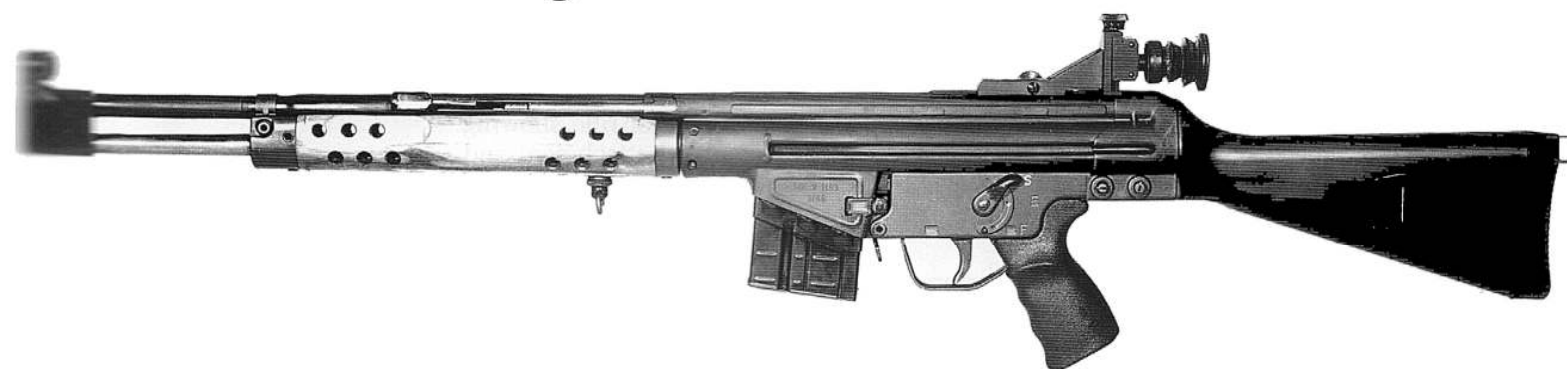
467. Left side view of the Biathlon version of the standard 7.62mm NATO calibre G3 serial no V 1193, produced in March, 1966.
