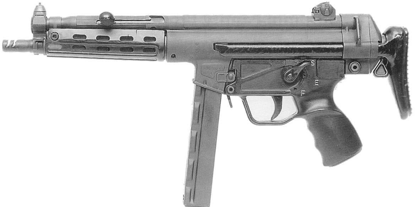
453. Left side view of a slightly later version of the MP64, manufactured in November, 1964. Compare with the above: note the addition of an integral muzzle brake, and the redesigned sights. The rear sight has
