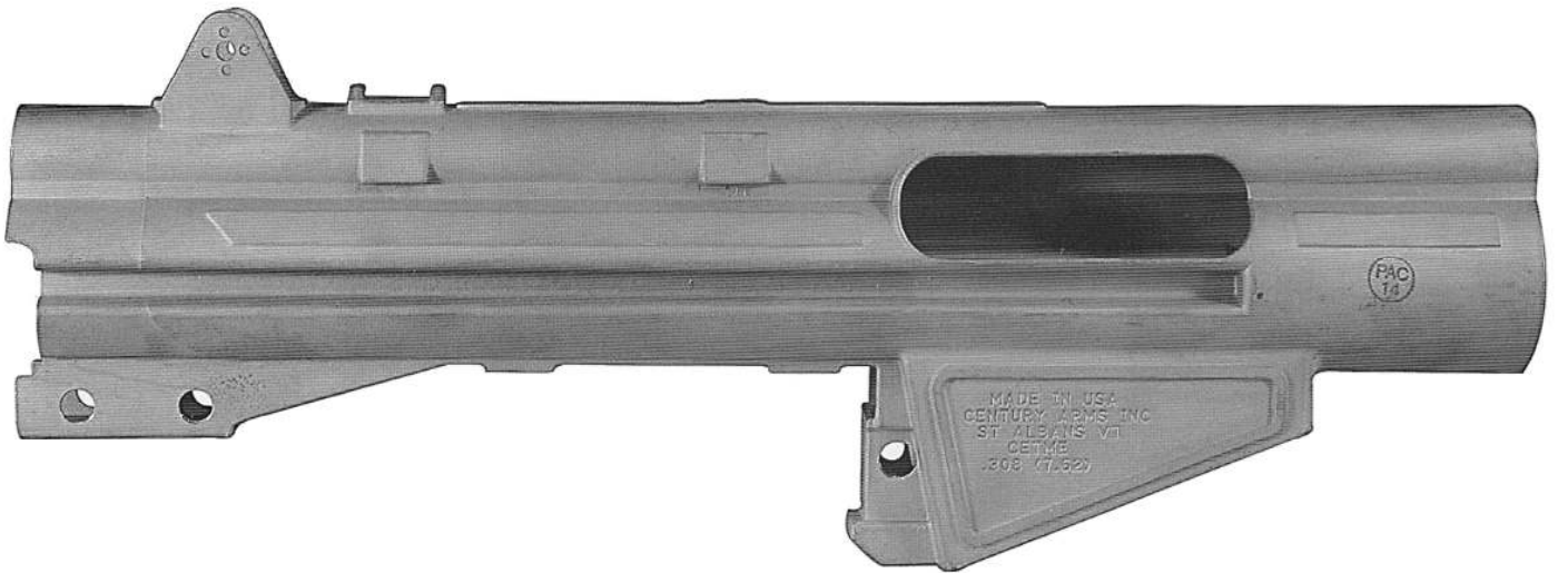
667. Right side view of the Century Arms investment-cast CETME receiver, bearing markings indicating Century's old St Albans, Vermont address.
