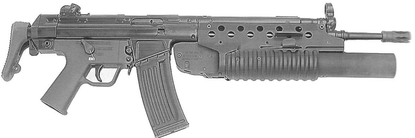
562. Right side view of an HK33E/A3 with stock retracted, fitted with a T-40 40mm grenade launcher.
