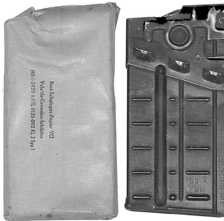
697. The 20-round aluminum magazine, standard-issue in the Bundeswehr for the G3 rifle.
