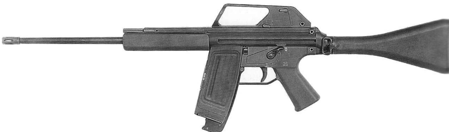
461. Left side view of a late prototype of the HK36 4.6x36mm assault rifle. Its unusual features are discussed in the text. courtesy the late Dr Edward C Ezell
