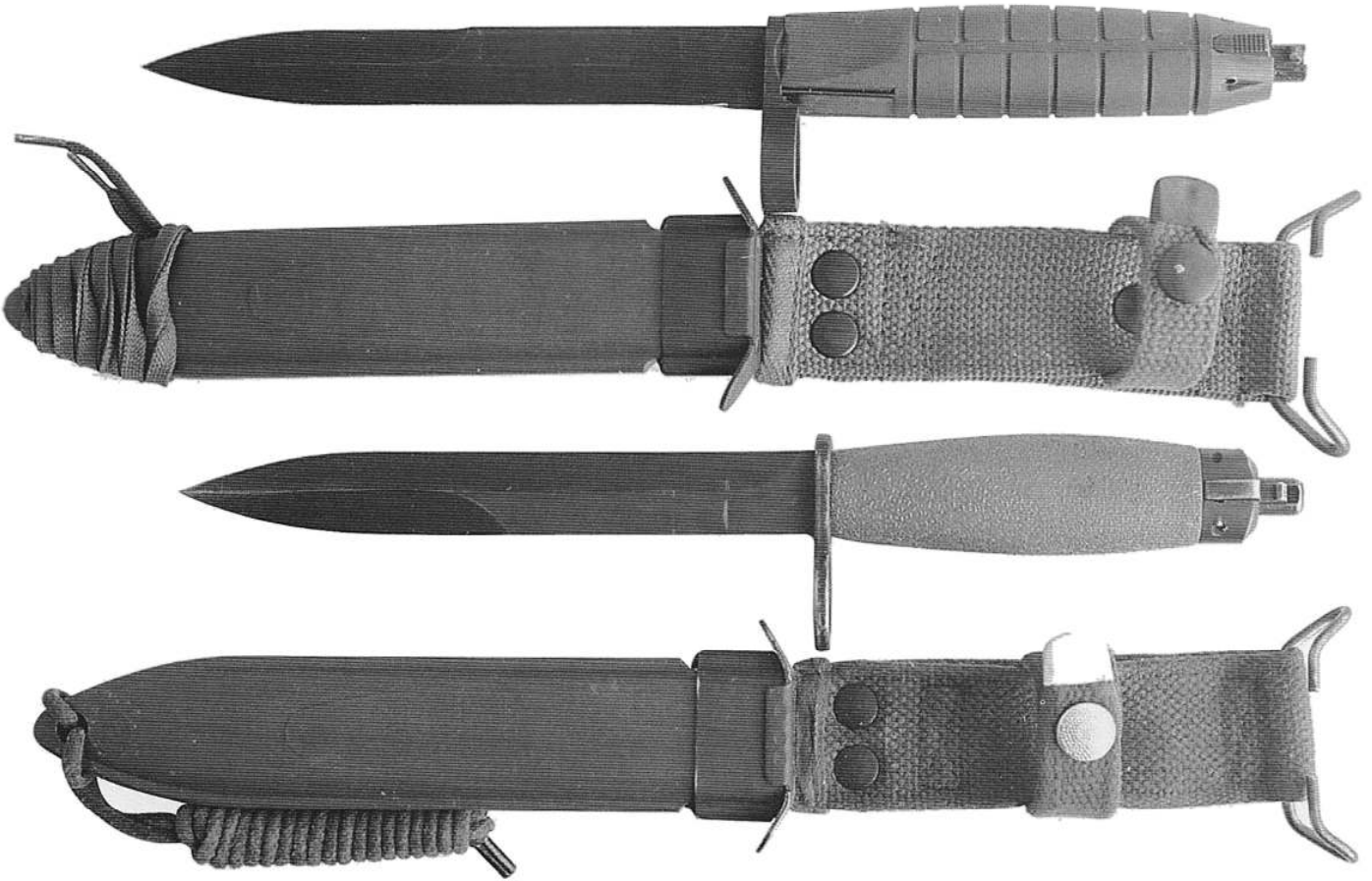
519. Two variations of AG3 bayonets and their scabbards. Above: new style, with grooved grip. Below: old style, with US-type blade and crossguard. Both scabbards resemble the common US pattern. courtesy Vidar Andresen
