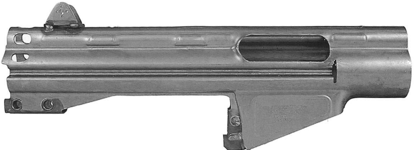
666. Right side view of the stamped receiver produced by Century Arms for use on its CETME clones. Markings read “CETME SPORTER .308 CAL./CENTURY ARMS
