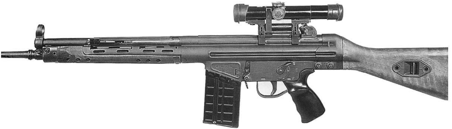
716. Left side view of an early G3ZF, marked "S G3 HK 0115" and dated July, 1963, fitted with a Hensoldt Telescope Sight 4 x 24 (ZF G3) in the early iteration of the
