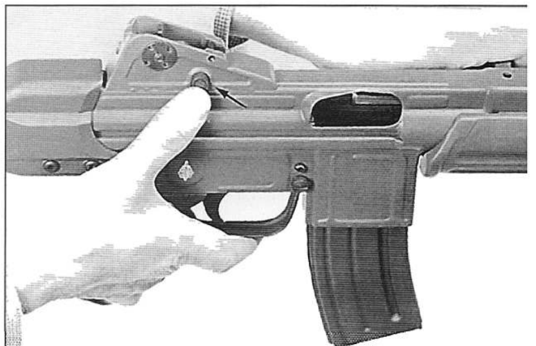
618 (right). Illustration from the CETME Model L manual, showing the method of engaging the bolt holdopen (arrow) while the bolt assembly is being held back by the charging handle.
