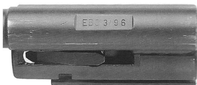
660. Left side closeup of the Sabre Defence XR41 bolt carrier, showing markings indicating manufacture by Hellenic Arms Industries of Athens in March, 1996.
