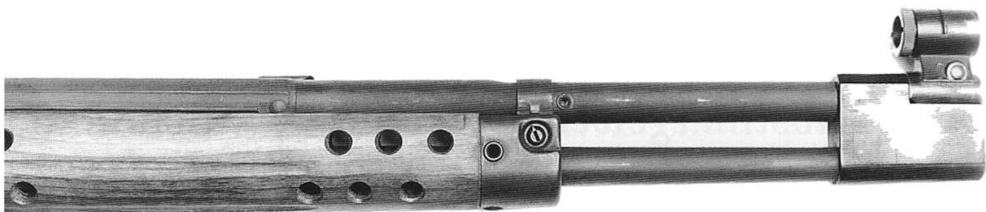
469. Right side closeup of the above Biathlon rifle, showing details of the Freischwinger handguard attachment and special front sight block. courtesy Walter Schmid
