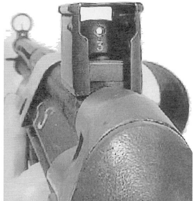
484. Rear closeup of a Danish G3 fitted with the expedient sunshade - an M1 Garand clip - over the diopter rear sight. During the 1980s some units were still issued with the M/50 (Garand), and it was common practice for users of the M/75 (G3) rifles to fit an M1 clip as shown to shade the rear sight in strong sunlight.
