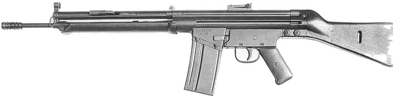
582. Left side view of a prototype of the CETME Model B, marked "F.A. CETME/A-312", fitted with the new flash hider, dimensioned for grenade launching, smooth black
