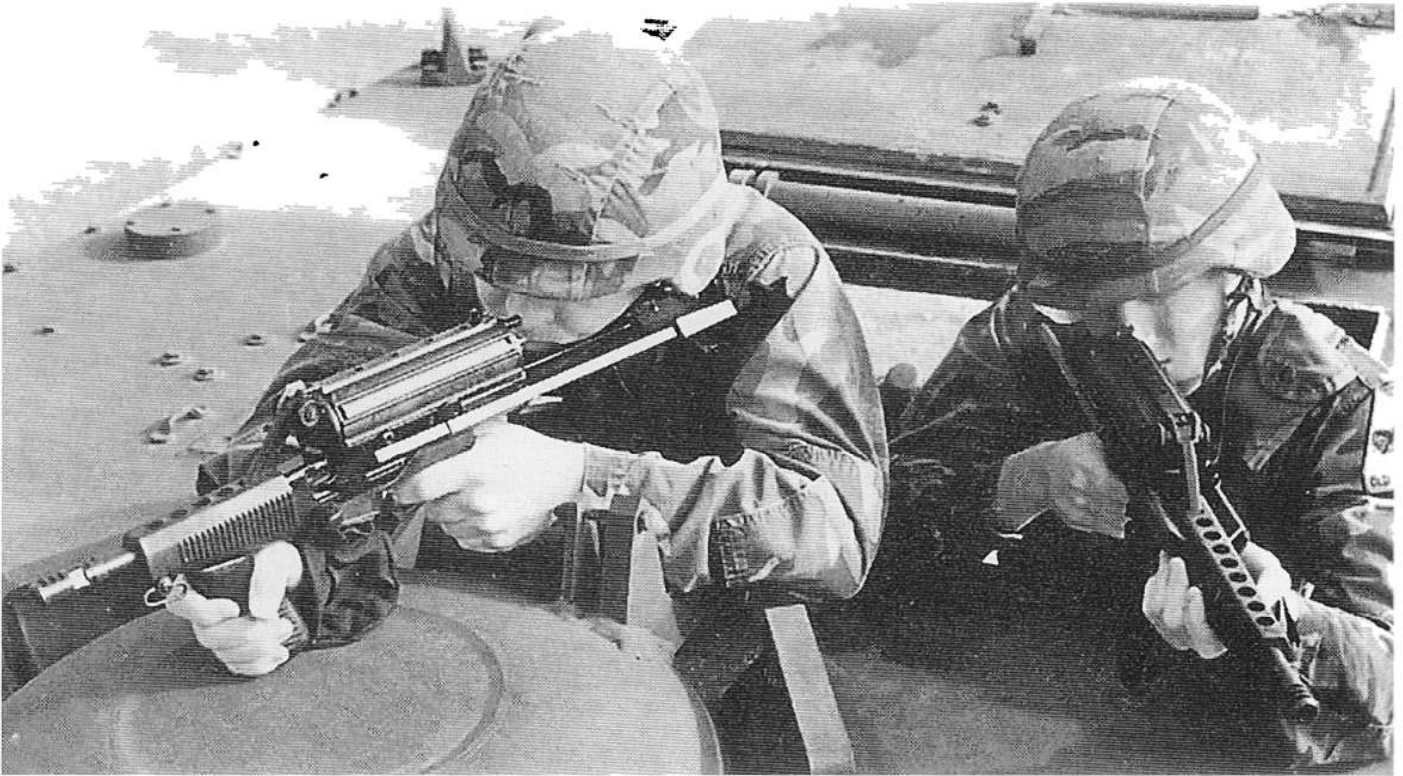
676. A photo from an advertisement headed "Maximum Firepower, Minimum Exposure", which appeared in Jane's Infantry Weapons , showing two selective-fire Calico weapons, the M-960A submachine gun, left, and the M-955A carbine, right. courtesy Mike Miller
