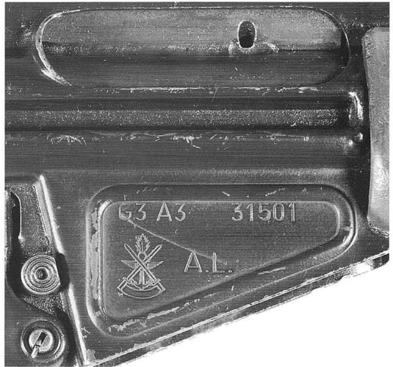
567. Right side closeup of a G3A3 rifle assembled at MAS, serial no 31501, marked with the crest and initials of the Lebanese Army (A.L.) courtesy Virginia Ezell
