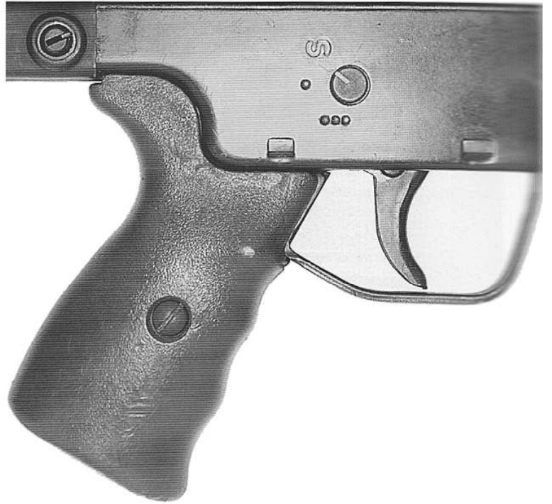
539 (right). Right side closeup of a Saudi Arabian G3A3 rifle, showing selector markings.
