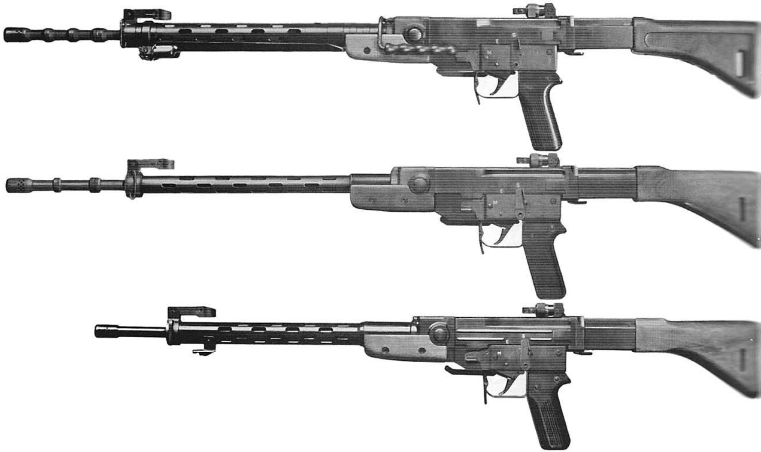
645. Left side view of three versions of the SIG 510 rifle, all featuring fold-down sights reminiscent of those used on the WWII German FG42 paratrooper rifle.
