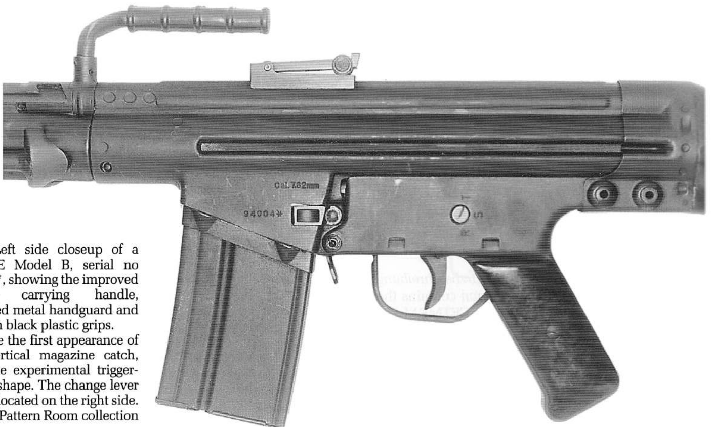
582. Left side view of a prototype of the CETME Model B, marked "F.A. CETME/A-312", fitted with the new flash hider, dimensioned for grenade launching, smooth black
