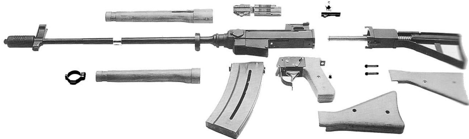
640. The above prototype stripped. The roller-locked bolt, above, shows its MG55 origins.
