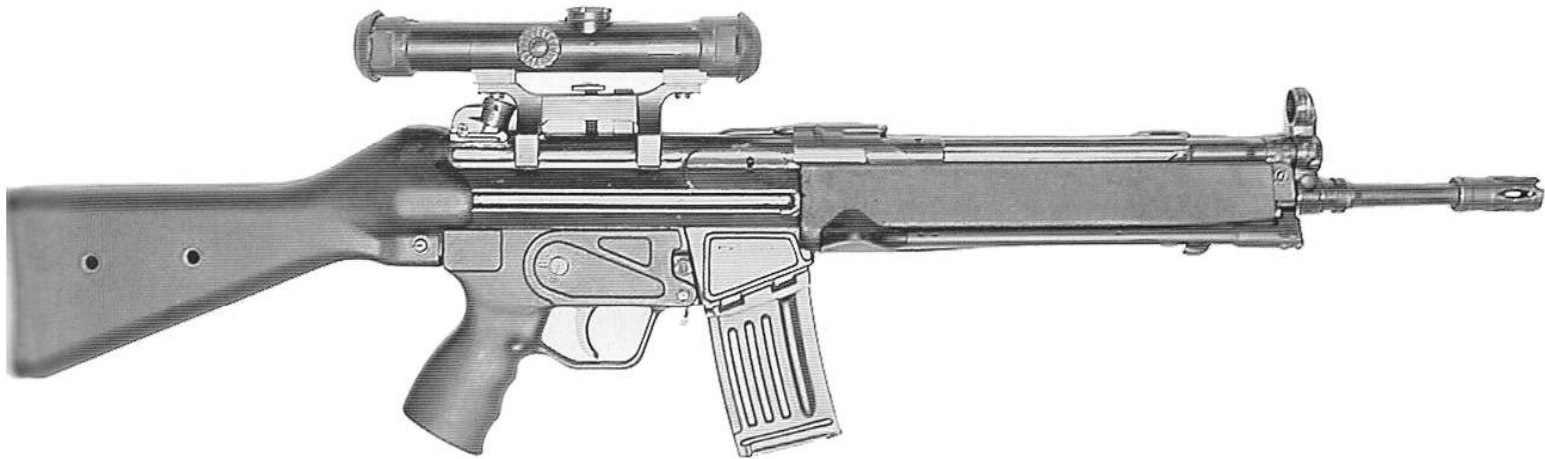
505. Right side view of a Malaysian-issue HK33, fitted with the one-piece black plastic stock and Export handguard with bipod.
