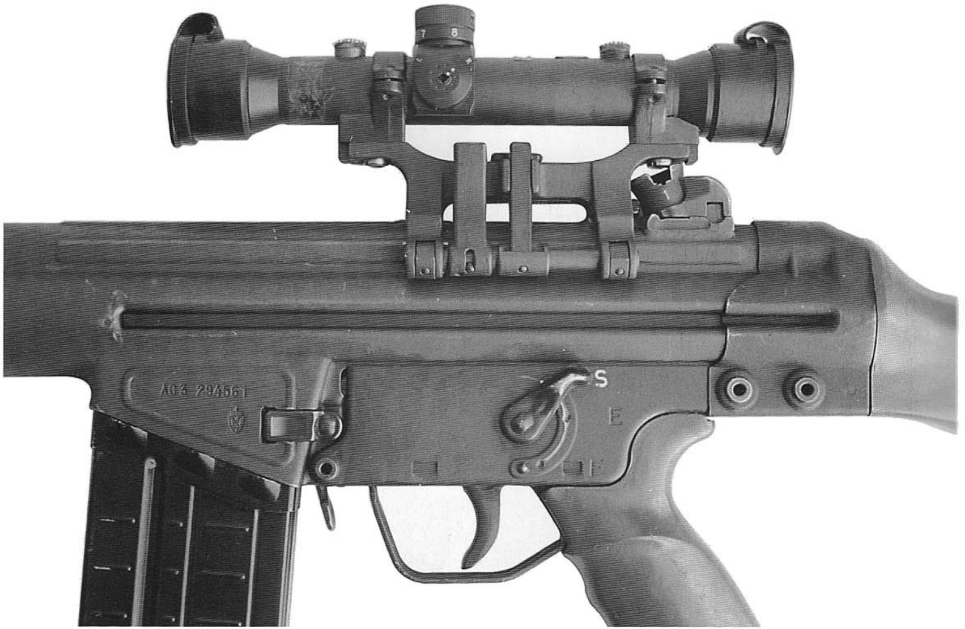
516. Left side closeup of a Norwegian AG3 sniper rifle, serial no 294561, with OIP scope shown fitted in H&K mount. courtesy Vidar Andresen
