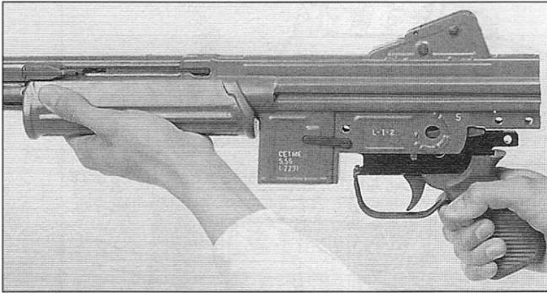
619. Manual illustration showing removal of the trigger group from the receiver of the CETME Model LC. courtesy the late Dr Edward C Ezell
