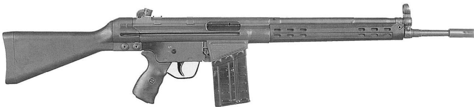
670. Right side view of an HK91 clone produced on the investment cast G3 receiver by Century Arms Inc.
