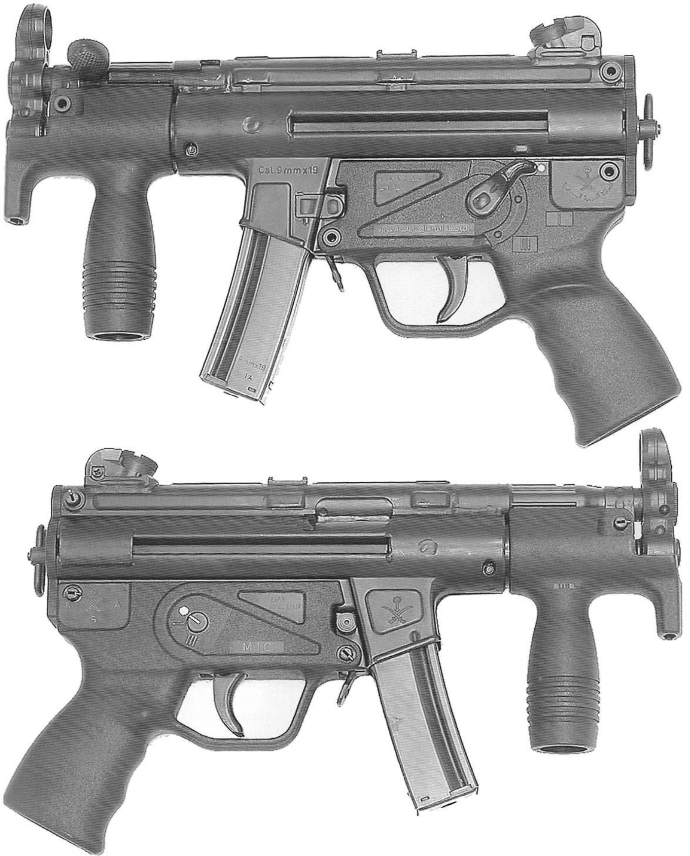
541. Left and right side views of a Saudi Arabian MP5K with curved 25-round magazine and flat end cap and swivel replacing any form of buttstock.
