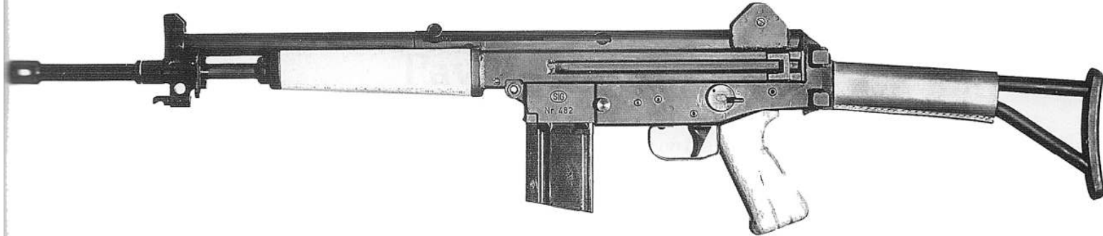
647. Left side view of the early folding-stock .223 calibre prototype for the SIG 530 series.
