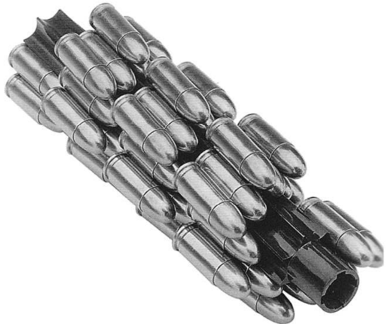
679. A right front three-quarter view of the central feed rotor, the “heart” of the ingenious Calico helical magazine, showing the way in which the 9mm cartridges are stacked in two helical layers. As noted in the text, “the cartridges roll on each other like ball bearings to minimize friction.” courtesy Mike Miller
