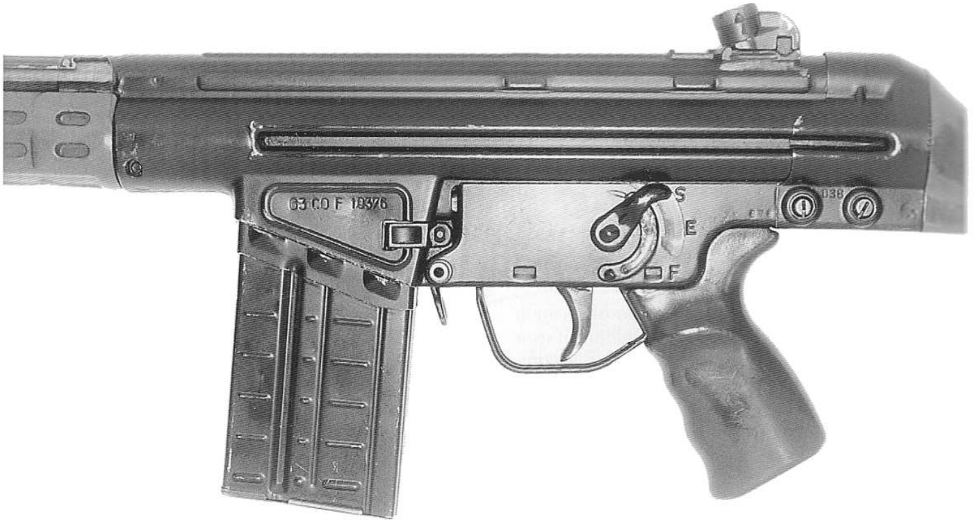
565. Left side closeup of G3 rifle marked "CO F", serial no 19376, fitted with plastic furniture and an aluminum magazine.
