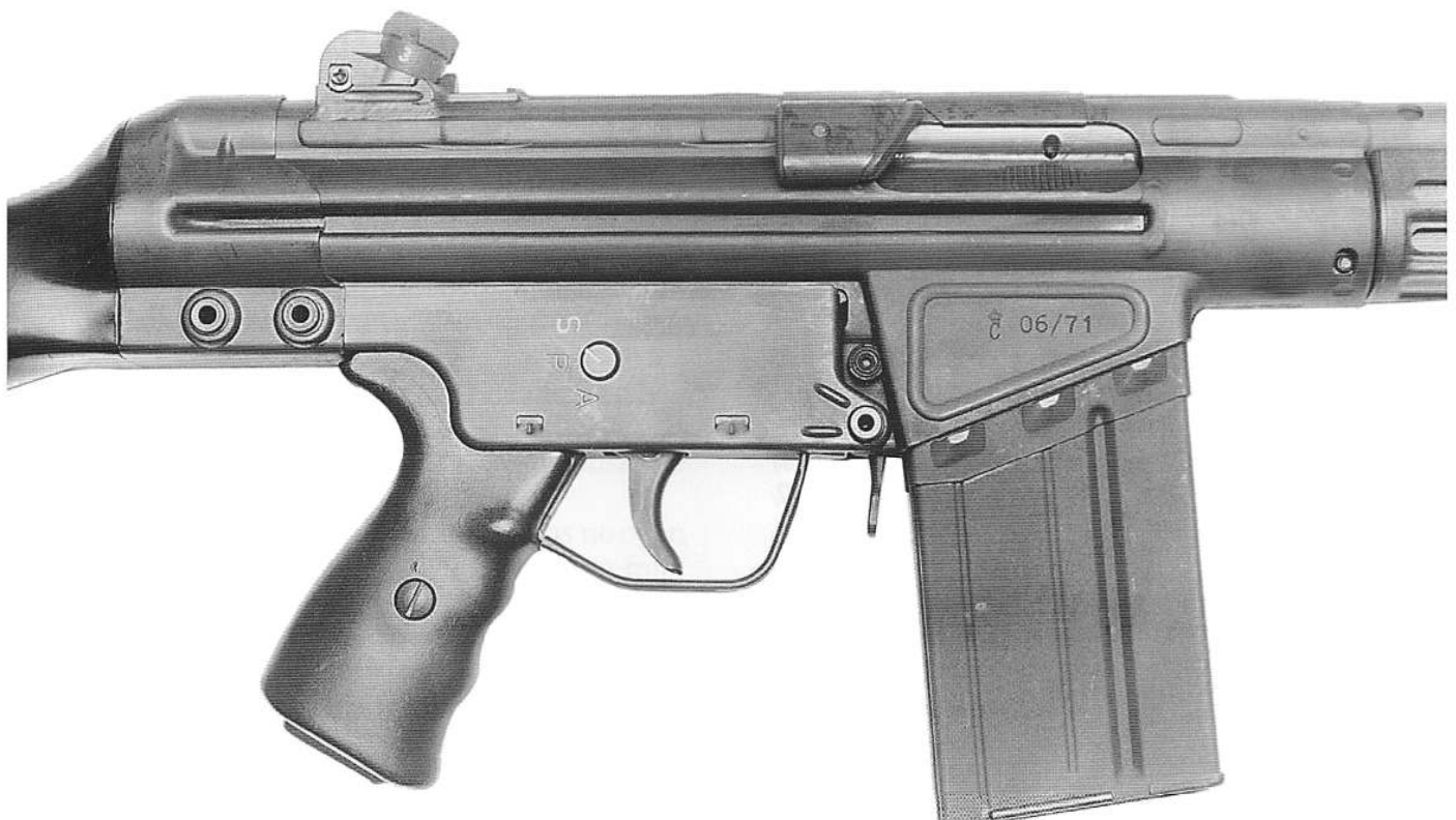
548 (below). Right side closeup of the above Ak 4, showing markings indicating manufacture by the Carl Gustafs Stads Gevärsfaktori in June, 1971.
