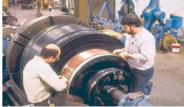
220 KW Exciter Armature for an Electric Utility generator
