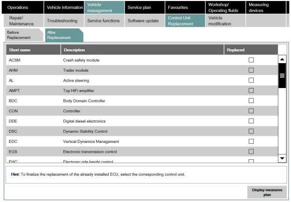
Then ISTA will automatically include the control unit validation in the measures plan.
