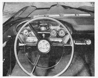
DRIVER'S EYE-VIEW of the instrument lay-out and "Teletouch" pushbutton transmission controls, mounted in the steering wheel "hub" on the new Edsel range. home should be completed in the British Resort Colony by race time, 1st-9th December.
