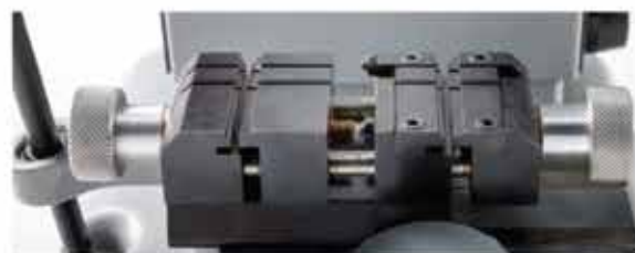
Replaceable jaws of the clamp on the cutter side
