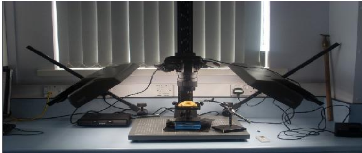
Figure 1 : The camera, computer, the stand and the source of illumination used in this study
