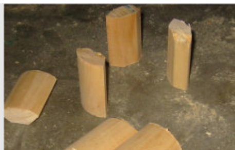
The central parts are glued together and the short pieces of moulding are test-fitted against the corners. They will need a little filler at the top because the moulding used has a flattened back. No trouble though – everything needs a bit of filling and sanding at some point!
