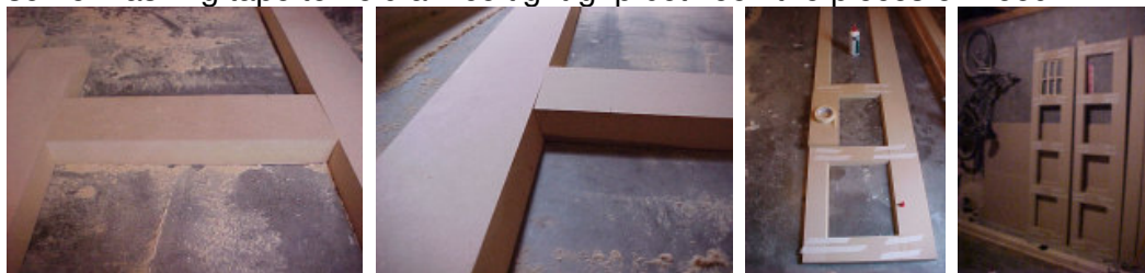
1) Test fit your pieces together 2) The long side rails should fit snugly 3) Masking tape is good for holding the pieces together tightly during gluing
