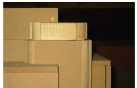
And a test fit of the cap in place. Note that it sits slightly inward of each edge of the actual corner post. It sits back from the front by the same amount, and in calculating it's depth you have to add the depth of the first "step" of the roof which it sits upon.
