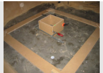
A piece of scrap wood is screwed underneath each corner of the platform which holds it all together since glue alone would flex and break quickly.
