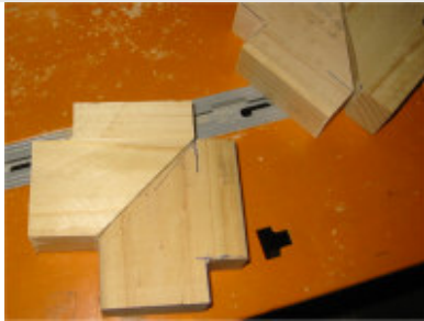
Here is a test-fit of one complete post-cap. Remember, these are not as wide as the actual corner post but are deeper so that they can sit on the first level of the roof.
