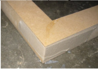
TIP: Masking tape can be a great aid at holding your wood in place whilst glue dries.
