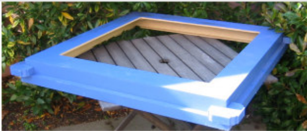
The corner post caps are attached to the top of the first step. As you can see the first step is the shortest and rises only as high as the top of the Corner Posts.
