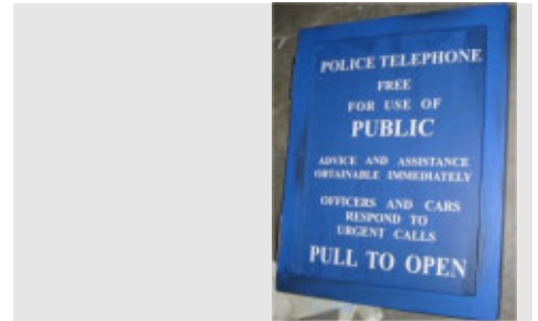
The Phone Panel could be printed as a solid image, but with individually laser-cut letters, you would still be able to read the sign when there are lights on the Box. Otherwise you would get a lot of reflection from the panel when using flash-photography.
