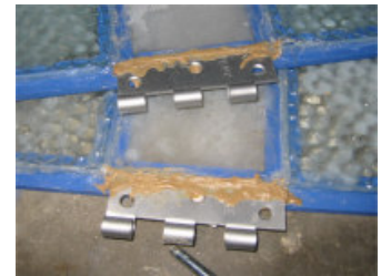
I cheated. I couldn't find the right gauge of screw and hinge in a hurry so I used No-More-Nails and simply stuck the hinges to the window frames. I should note that all of the glass and Perspex was sized to leave a 1cm rim around the back of the frame for attachment.
