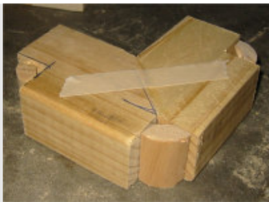
The central parts are glued together and the short pieces of moulding are test-fitted against the corners. They will need a little filler at the top because the moulding used has a flattened back. No trouble though – everything needs a bit of filling and sanding at some point!
