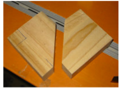
They are cut at a 45 degree angle so that they'll fit snugly. The joint will be hidden at the front by the quarter-round moulding
