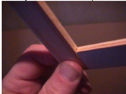
See how the recessed cuts help the two halves to fit together? Just remember to make all your cuts on the same side of the wood – trust me, stranger things have happened...
