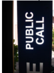
With a light source behind it, the opaque Perspex becomes white and glows. The surrounding blue film also illuminates
