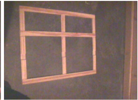
More Vertical rails are glued and pressed together
