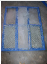
With the window flat down on the ground I left a mixture of paint and spirits to evaporate leaving random smudges and stains. Naturally you should test this process on scrap material first to get your mix right. Good ventilation is a must for this procedure as well.
