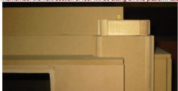
Internally, the first few steps were a very simple construction. Simply a square frame initially of the total height of the first 2 steps. After gluing and screwing together, this is surrounded on the outside by parts comprising the thinner first step which are glued to the outside lower edges. The top platform is almost a 2-D sheet made from 4 panels cut with 45 degree corners. These are slightly shorter than the total size of the step so that they will sit inside the frame. It is glued in place and then reinforced with corner supports and a few blocks along their length to add strength. Remember the next section of roof will be sitting on this platform later.
