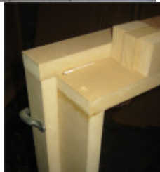
On this frame, build another layer – this will become the ‘first’ step. Scrap wood of known thickness becomes handy spacing blocks
