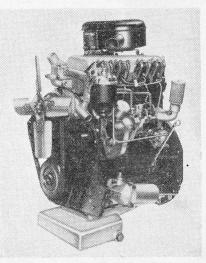
SMALL DIESEL: The compression ignition engine reigns supreme in the commercial world. This is the latest engine from Rootes: a 2.26-litre 4-cyl., with indirect injection and Ricardo Comet III patent combustion chambers. Power output is 50 b.h.p. at 3,000 r.p.m., and 4,200 r.p.m. can be attained.
