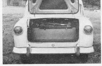
BOOT is capacious and incorporates a drop-down rack for the basic tool kit.
