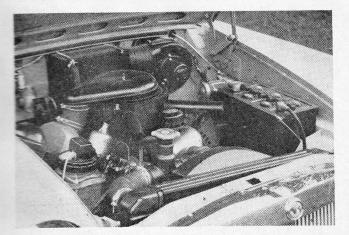
BONNET is well-filled and reveals twin SU carburetters on a TR3-type manifold.
