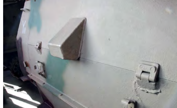
The armour on the rear of this Wespe was a lot thinner. It ranged from 8.7mm to 9.2mm
