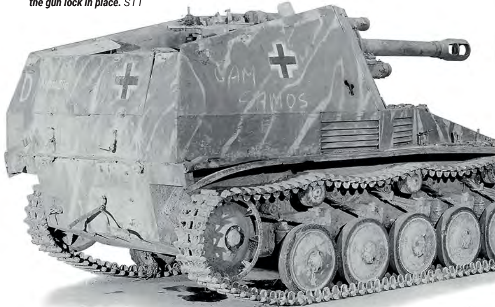
ABOVE & BELOW: Captured 10.5cm Wespe Artillery Self-propelled guns were examined by the British School of Tank Technology. This model is missing its rear exhaust silencer box below the rear hatch and has the gun lock in place. STT
