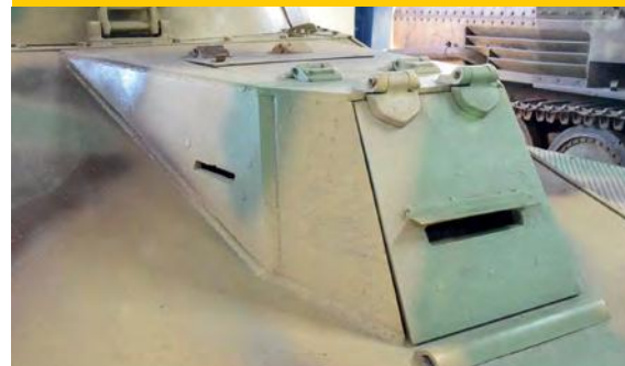
The driver was given an armoured compartment on the left side of the tank that protruded through the slopping front armour
