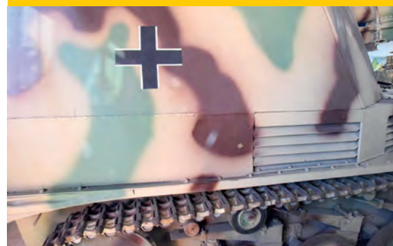
The thickness of the superstructure armour plate on the right side of this Wespe varied between 10cm to 10.4cm
