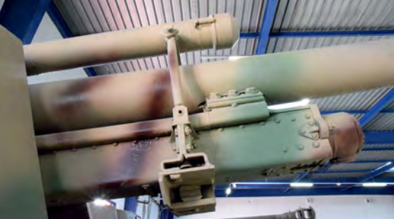
The tubes above and below the gun barrel helped reduce the recoil. The gun shield armour on this Wespe varied in thickness from 10.8mm to 11.6mm
