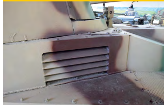
The armoured louvred grills around the Wespe varied in thickness from 8.7mm to 9.5mm
