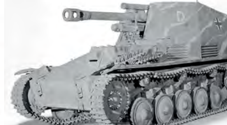
OPPOSITE: The Wespe Artillery SPG was built on a Panzer II tank chassis
