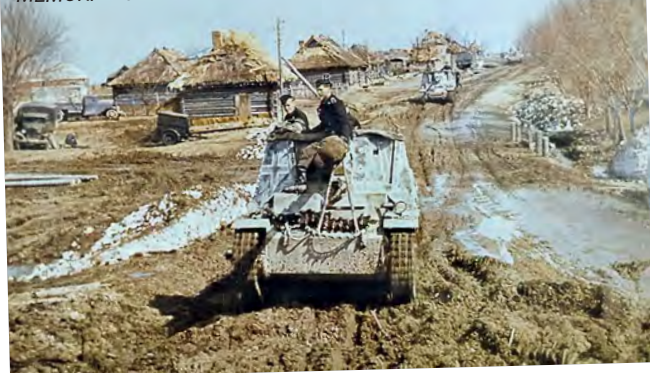
A column of German 10.5cm Wespe self-propelled guns covered in whitewash, passing through a Russian village. AUSTRALIAN WAR MEMORIAL 044595
