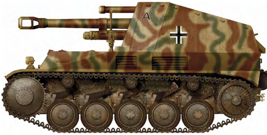
0.5cm leFH 18/2 (Sf) auf Fahrgestell Panzerkampfwagen II 'Wespe' (Sd.Kfz.124) artillery self-propelled gun from the 1st Abteilung, Panzerartillerie regiment, 8th Panzer-Division, Ukraine, summer 1944. DAVID BOCQUELET
