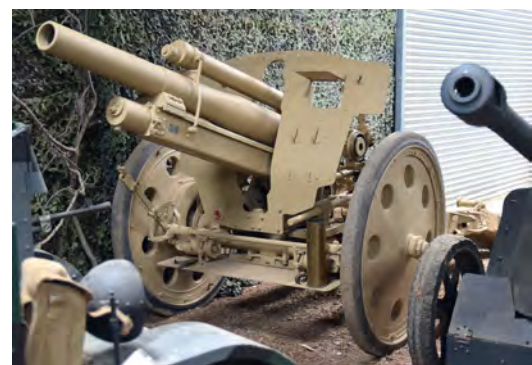
This 10.5cm leichte Feldhaubitze 18 (10.5cm leFH 18) light field howitzer is in the Armageddon Paint Ball Museum. It was this type of weapon that was mounted in the Wespe. STT
