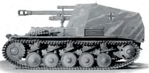
OPPOSITE: The Wespe Artillery SPG was built on a Panzer II tank chassis
