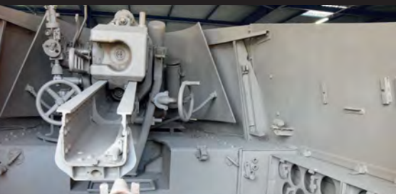
The 10.5cm leFH 18 gun used two-part ammunition. The high explosive HE projectile would be loaded first and then the cartridge propellant case. Depending on the range of the target different sized bags of propellant were inserted into the cartridge. More bags were used for longer range targets
