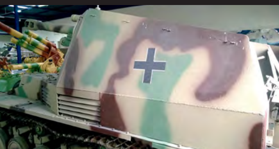
The upper superstructure that protected the crew from small arms fire and shrapnel was supposed to be constructed from 10mm thick armour plate, but the left side plate on this Wespe was found to vary from 11mm to 11.4mm thick
