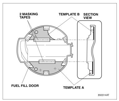
7. Using a pushpin, pierce the center of three marks on the templates A and B.
