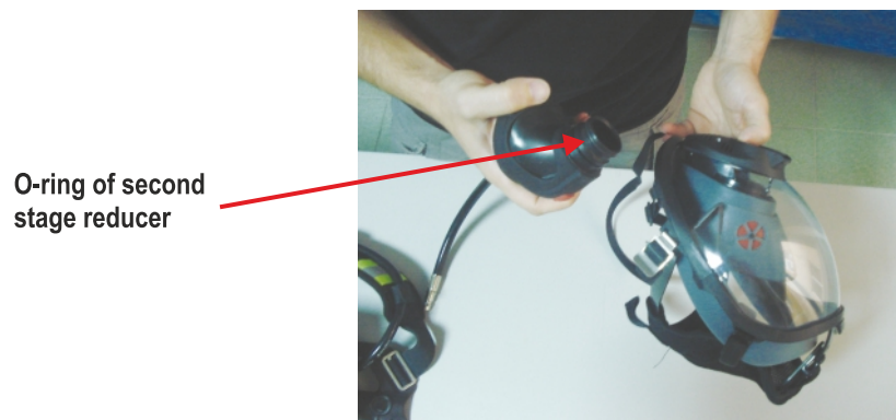
Figure 11 Visual checking of second stage reducer and face mask
