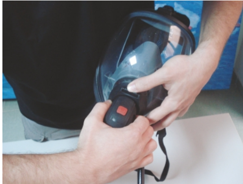
Figure 6 Detaching the Second Stage Regulator from the Face Piece
