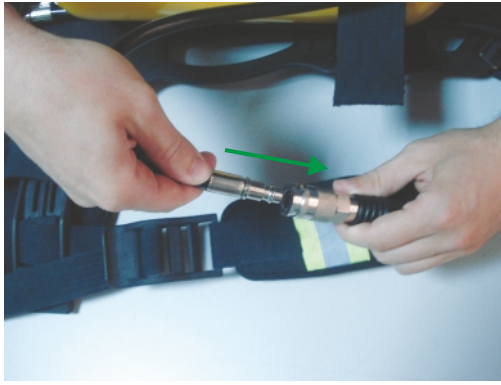
Figure 14 Assembling the Second Stage Regulator with the first stage regulator by the fast joint.
