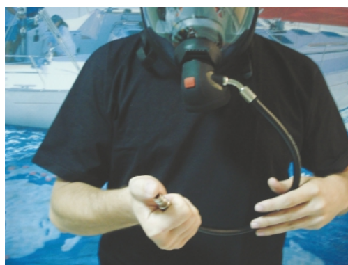
Figure 13 Face piece leak tightness test
