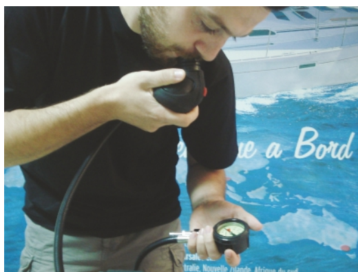
Figure 9 "ON DEMAND" valve operability check
