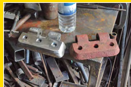
Above: Jon couldn't get the original cast steel hinges so made some himself.
