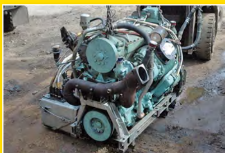
Above: Engine and various other running gear came from a donor FV432.
