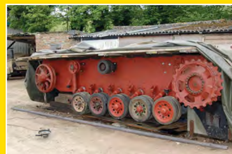
Above: Work started on the lower hull first, with Jon, aided by various friends and other enthusiasts, carrying out the repair work.
