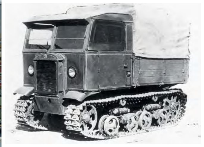
The STZ-3 was later adapted specifically as a forward control cab artillery tractor for military service. This is a prototype STZ-5 based on the STZ-3 chassis but with forward control cab, rear cargo area and 'road' tracks. MIKHAIL SVIRIN
