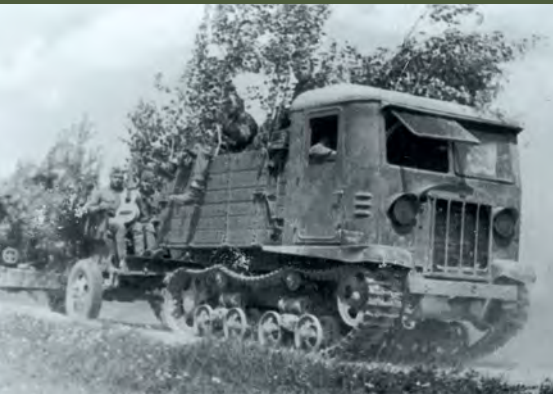
An STZ-5 in Red Army service, complete with guitar carrying gun crewman, August 1942
