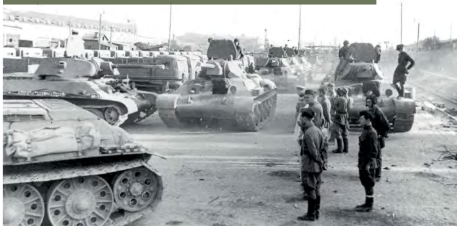
STZ produced T-34 tanks during delivery acceptance. Note the mix of cast and welded turrets, the latter with the distinctive STZ 'chisel' in the frontal turret armour, the sloped STZ gun mantlet shield and the all-steel road wheels
