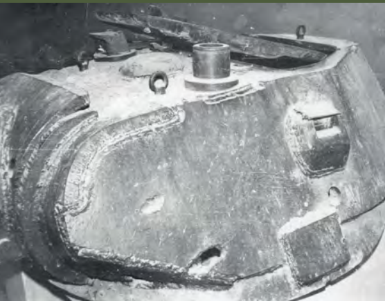
The distinctive features of the Stalingrad produced welded turret T-34 include the turret undercut and sight arrangements
