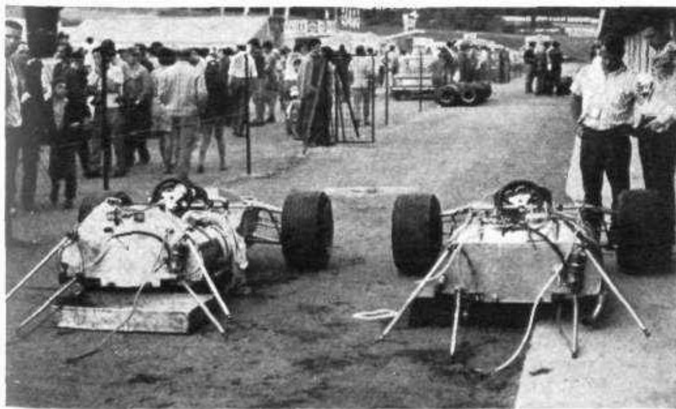
BT33s SHUFFLED.—When Cosworth engine trouble struck the Brabham team in practice there was a general switching of cars and engines between Brabham and Stommelen. This photograph illustrates some of the differences between the chassis of two cars, the newer one being on the right.
