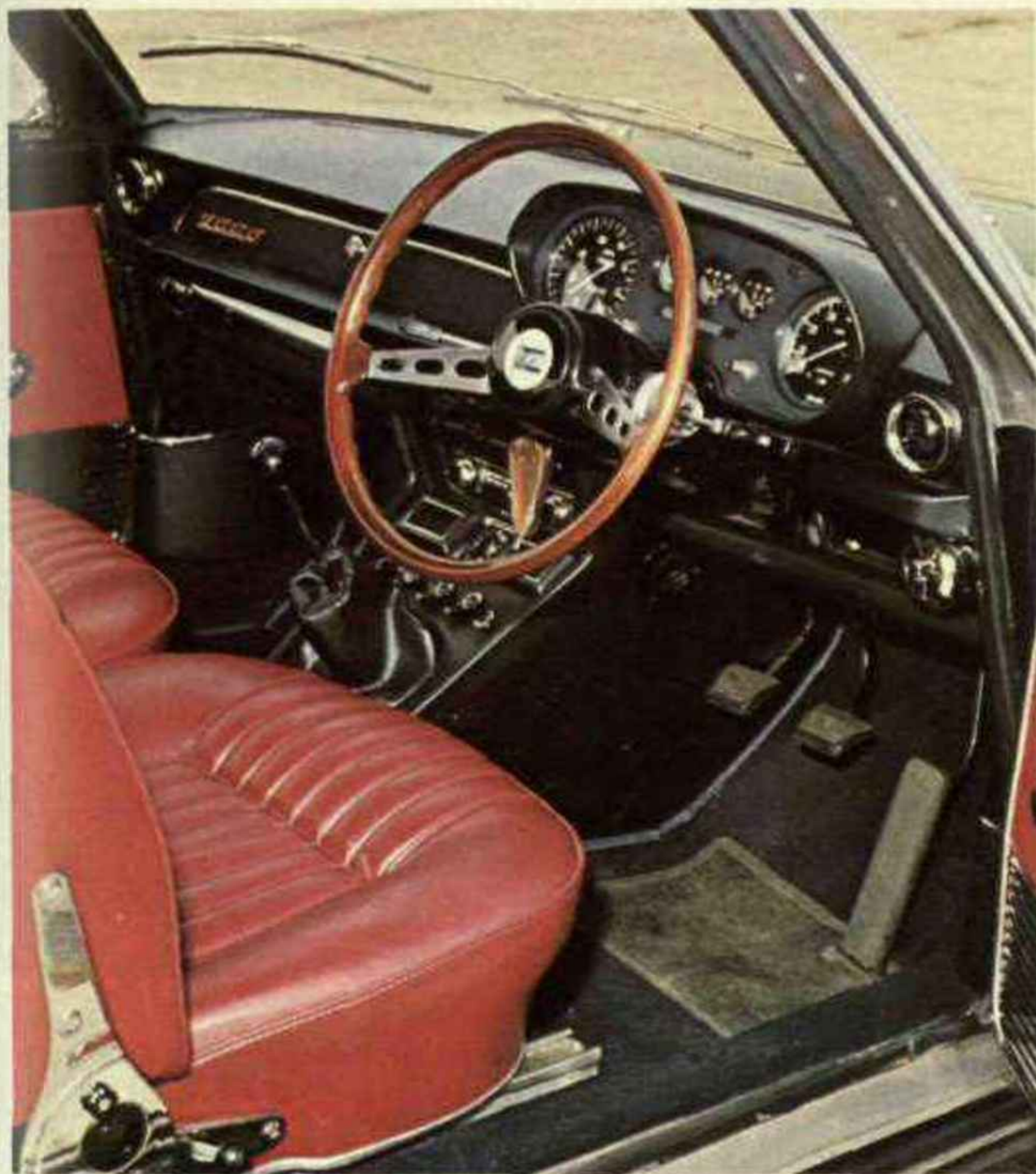
The driving compartment has a good driving position for the long-legged, with typical Lancia gear-lever, pendant clutch and brake pedals, treadle accelerator and hooded instruments.
