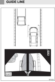
Check the positions and distance between the vehicle width guide line and a target object such as the obstacle or curb of the road.
