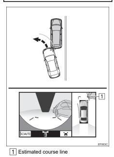
Three-dimensional objects (such as the overhang of a wall or loading platform of a truck) in high positions may not be projected on the screen. Check the safety of the surroundings directly.
