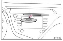
After insertion, the disc is automatically loaded.
