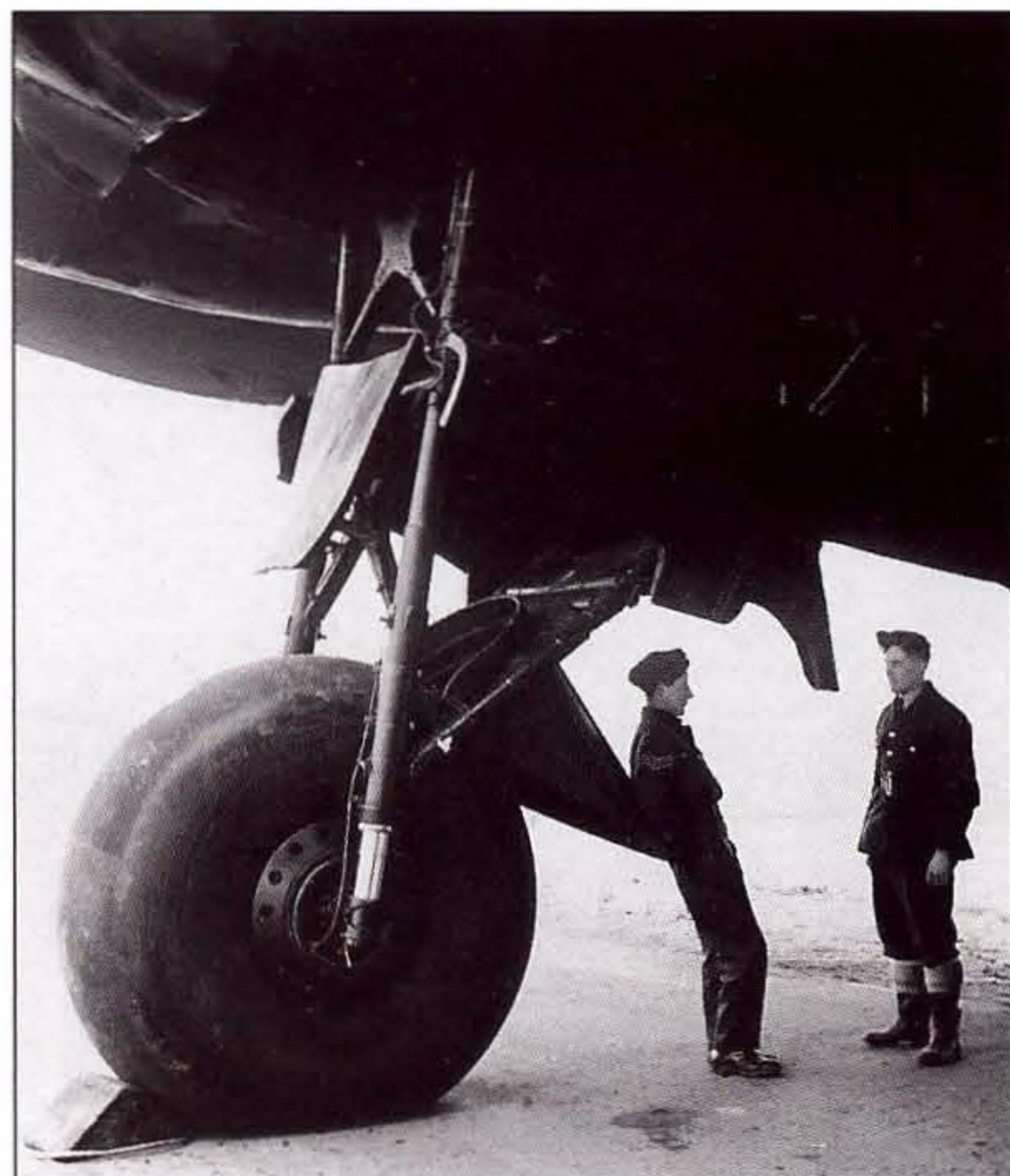
ABOVE Either the most accurate belly-landing of all time, or more likely the result of an undercarriage collapse while running the engines at Digby in 1942.
