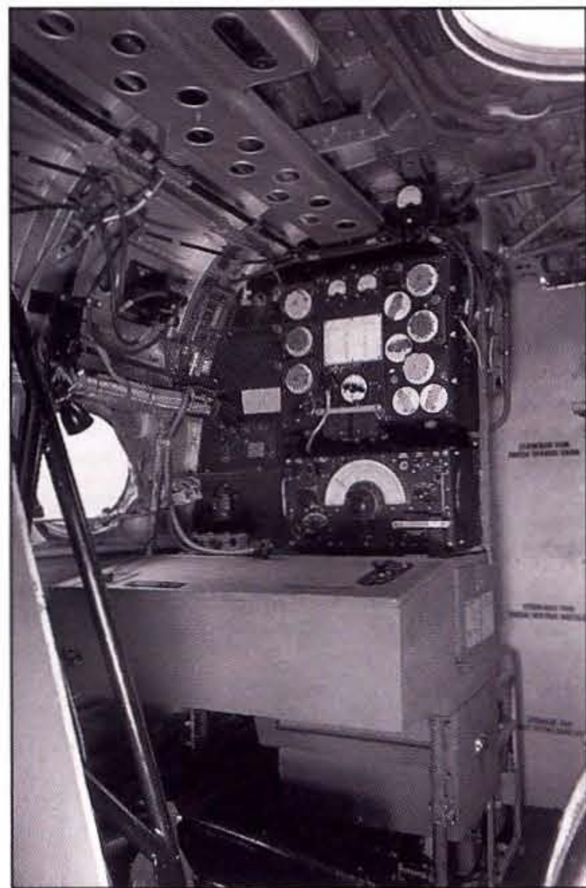
TOP The bomb-aimer's station was positioned directly below the nose turret, again providing plenty of room and a wide field of view. Note the selector switches to the right of the bomb-aimer's position.
