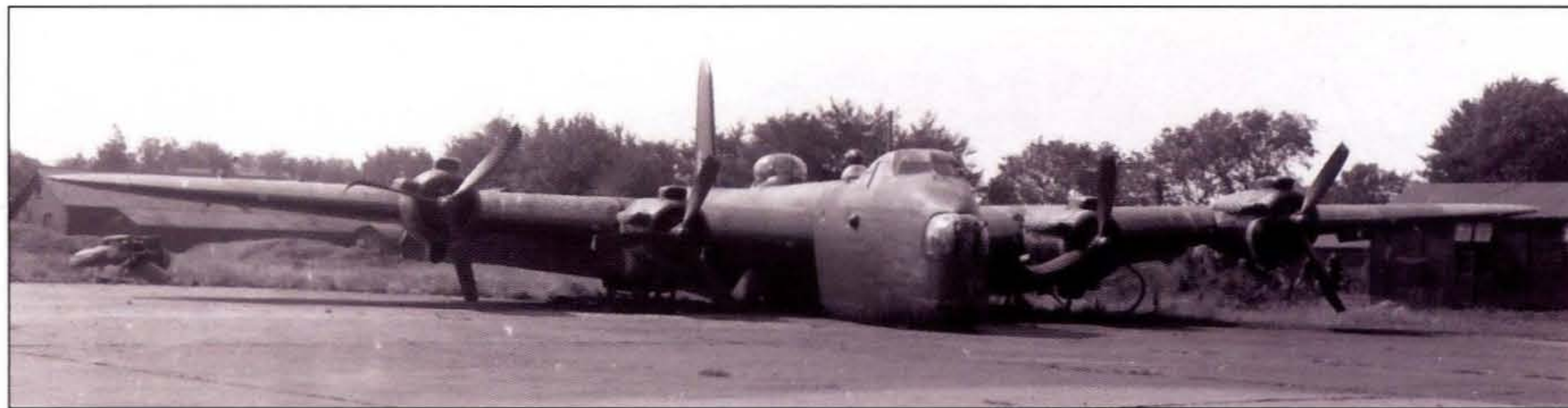
ABOVE Either the most accurate belly-landing of all time, or more likely the result of an undercarriage collapse while running the engines at Digby in 1942.
