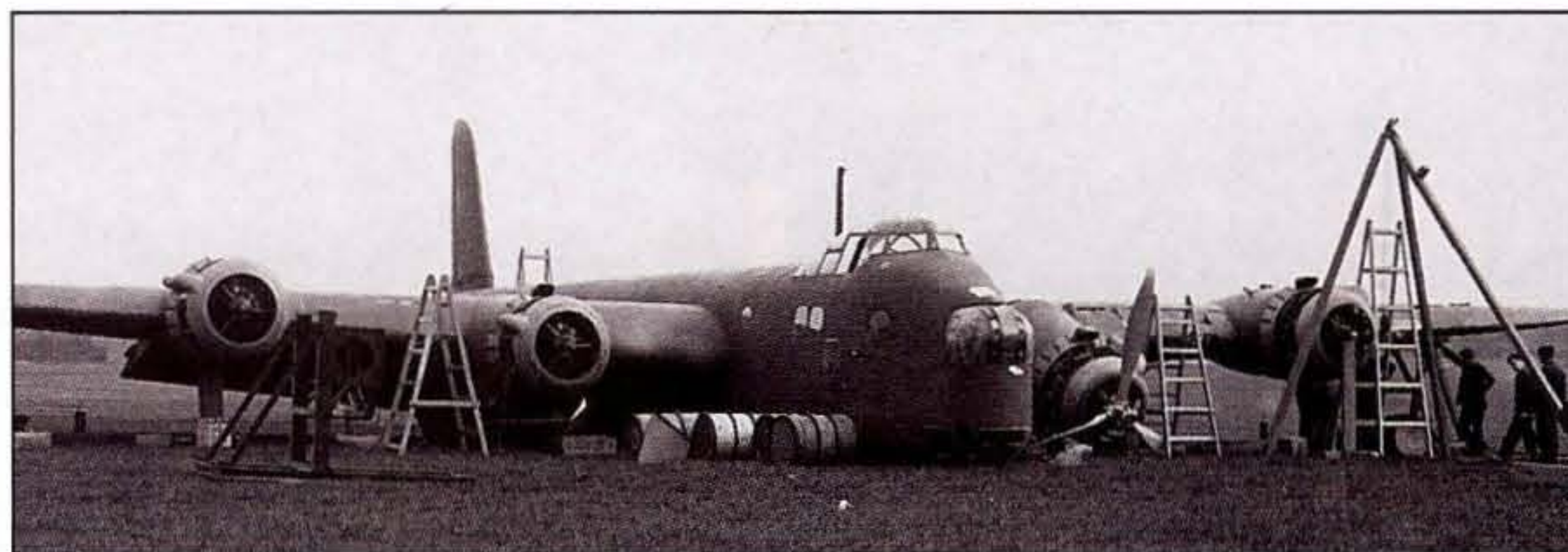
ABOVE The Stirling prototype, L7600, suffered an undercarriage collapse on its maiden flight on May 14, 1939, after a brake seizure on landing. The damage was extensive enough for the aircraft to be declared a write-off.
