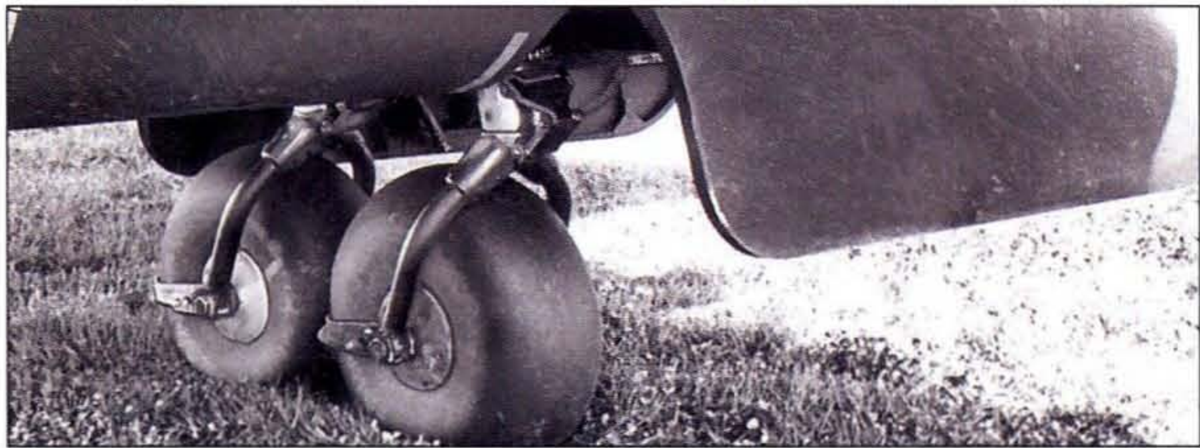
LEFT Twin tailwheels linked by chain and sprockets were used to avoid a large single wheel taking up space needed for the tail turret.
