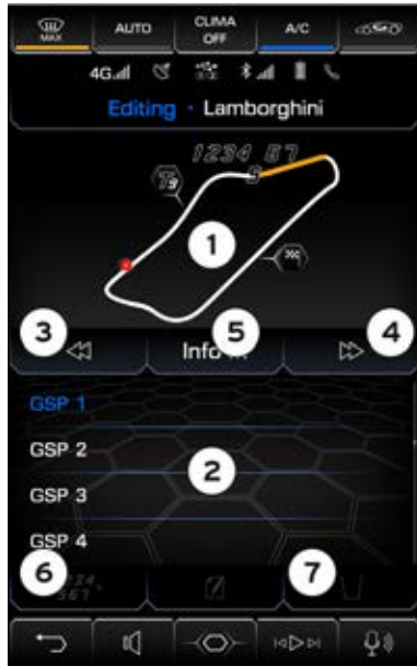
Fig. 91 Entering/deleting gear recommendations.
