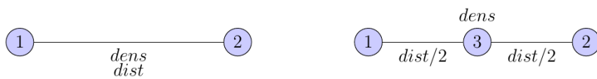
Figure 4.4: On the left, an edge of the original graph. On the right, the input graph to the heuristic.
