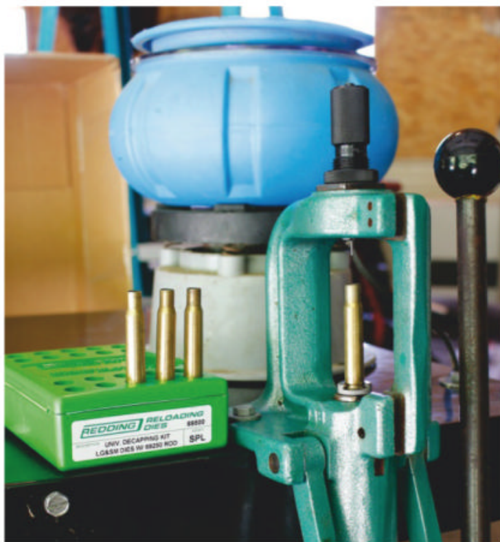
A Universal Decapping Die will remove spent primers from your cases before you resize them, allowing the primer pockets to be cleaned, keeping dirt and debris out of your resizing die.
