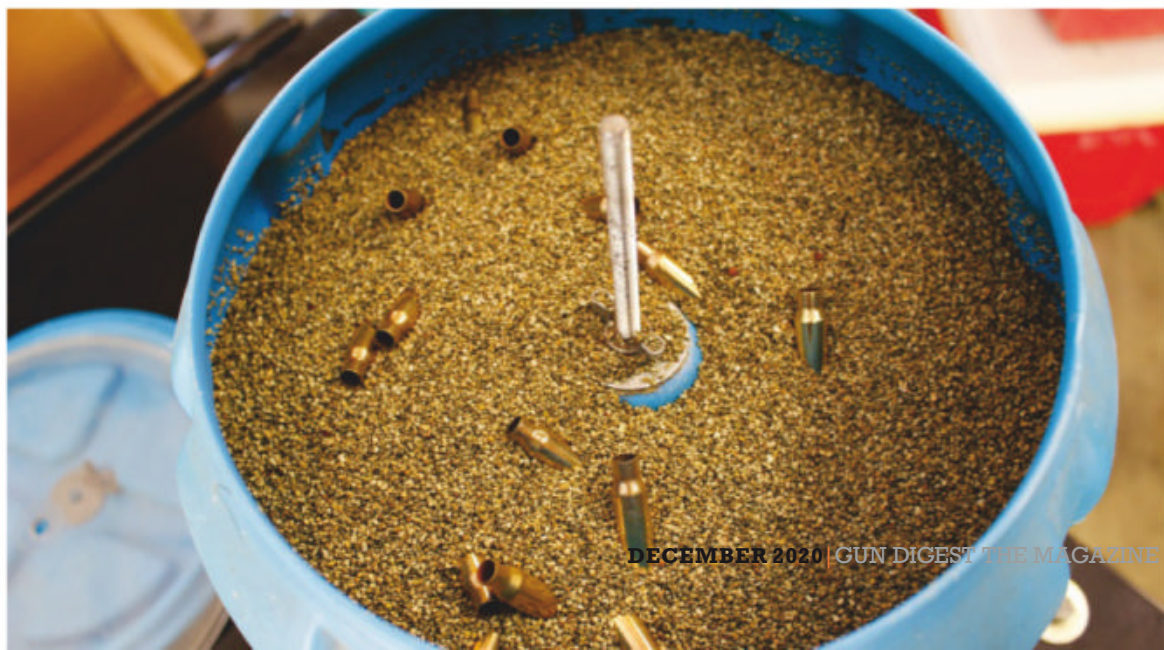
Ground walnut shells are just one type of abrasive media used to scour and polish brass cases.
