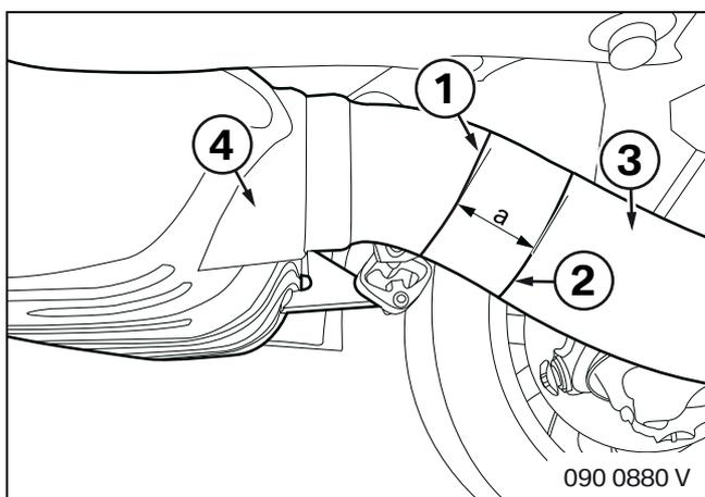
From the marking (1), draw a mark (2) at a distance of  $a = 40 \text{ mm}$  on the entrance pipe (3).
