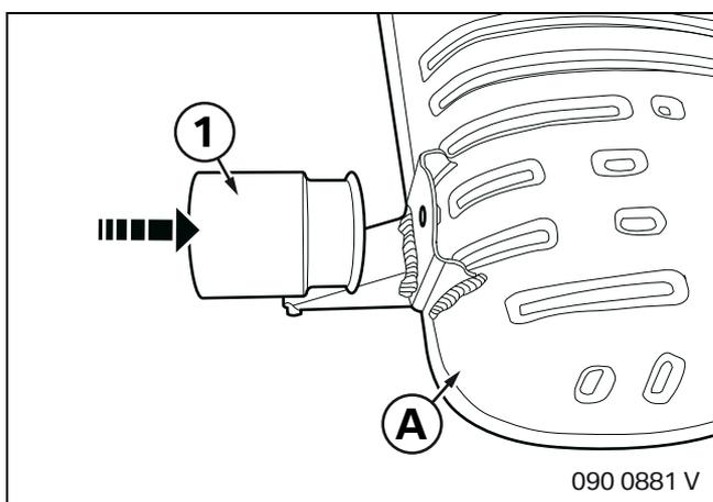
Uninstall acoustic distributor (1) on the standard silencer (not shown) and fit it to Performance silencer **A**.
