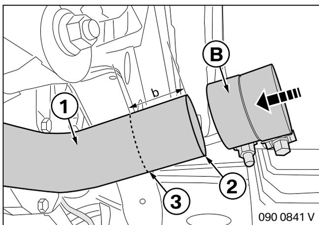
Mark the entrance pipe (1) from the cut end (2) with a distance of  $b = 35 \text{ mm}$  (3).
