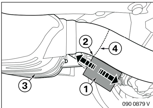
Using a suitable flat object (1), determine and mark (4) the start of the curve (2) of the entrance pipe into the rear silencer (3) by moving the flat object (1).
