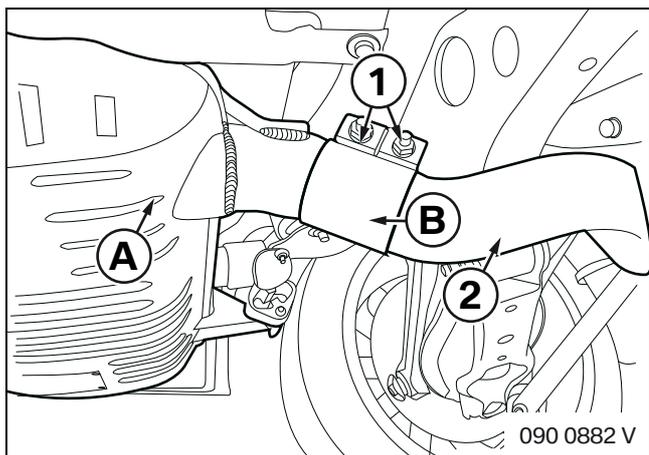
▶ In order to ensure adequate ground clearance, the screws (1) must not be below the pipe geometry and must be directed appropriately upwards, as shown in the figure. The screws (1) must have a distance of **20 mm** to all neighbouring components. ◀
