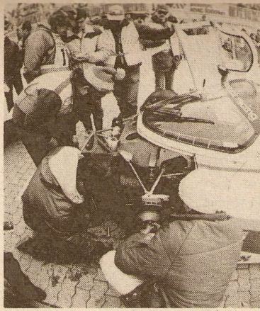
Rebuilding the Fitz 956's suspension.
