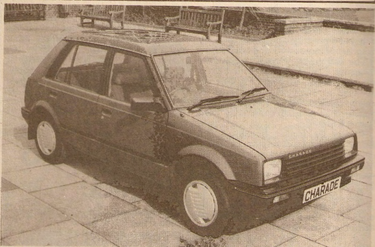
The restyled Charade has the in-vogue angular body shape with low Cd factor of 0.39.
