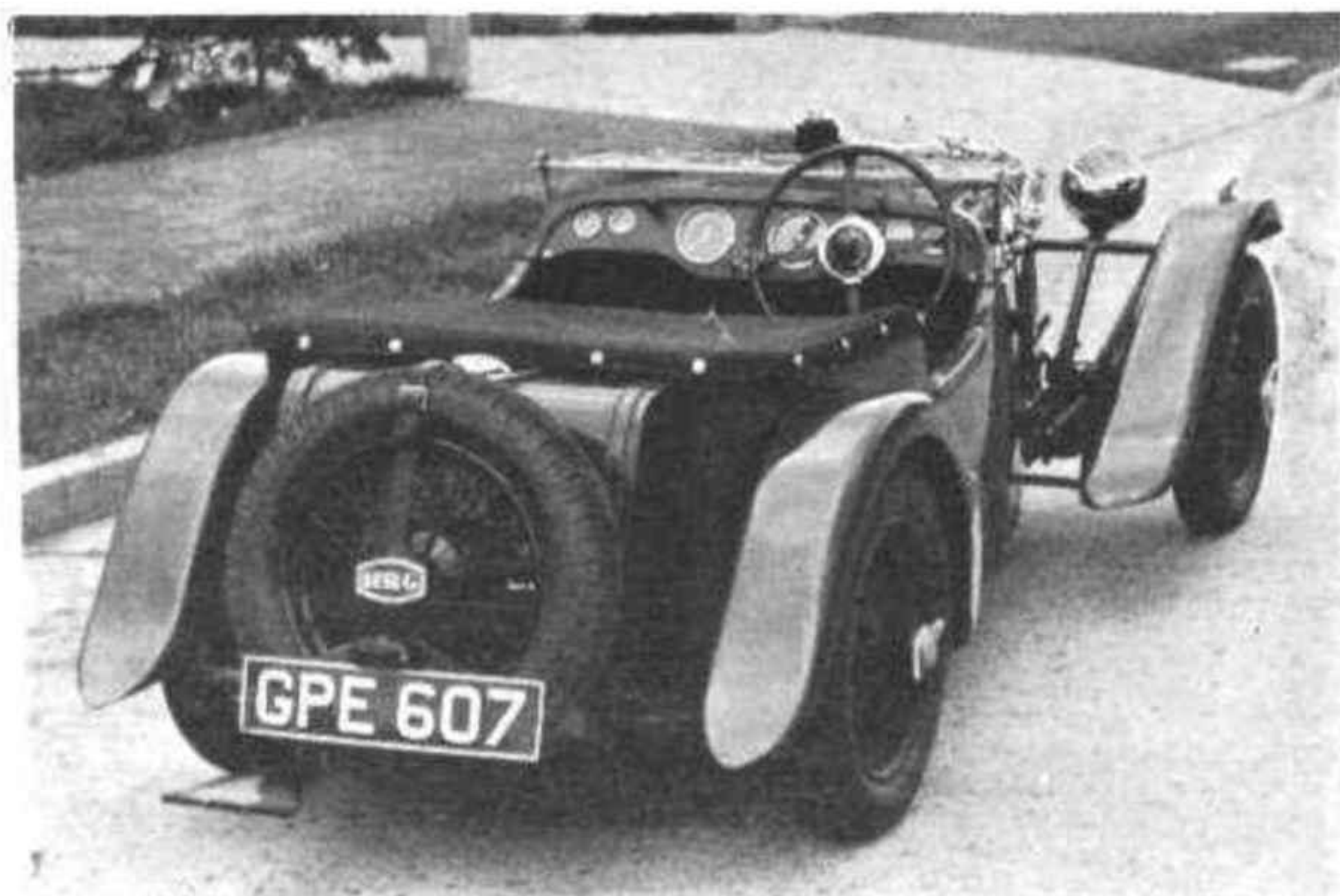
TYPICAL. —The pre-war H.R.G. was typical of the best type of small sports car. The first models had a 1½-litre push-rod Meadows engine and could do nearly 90 m.p.h.; later o.h.c. Singer engines were used and today, made only in 1½-litre form, it is by far the most costly of Britain's under-1½-litre sports models.
