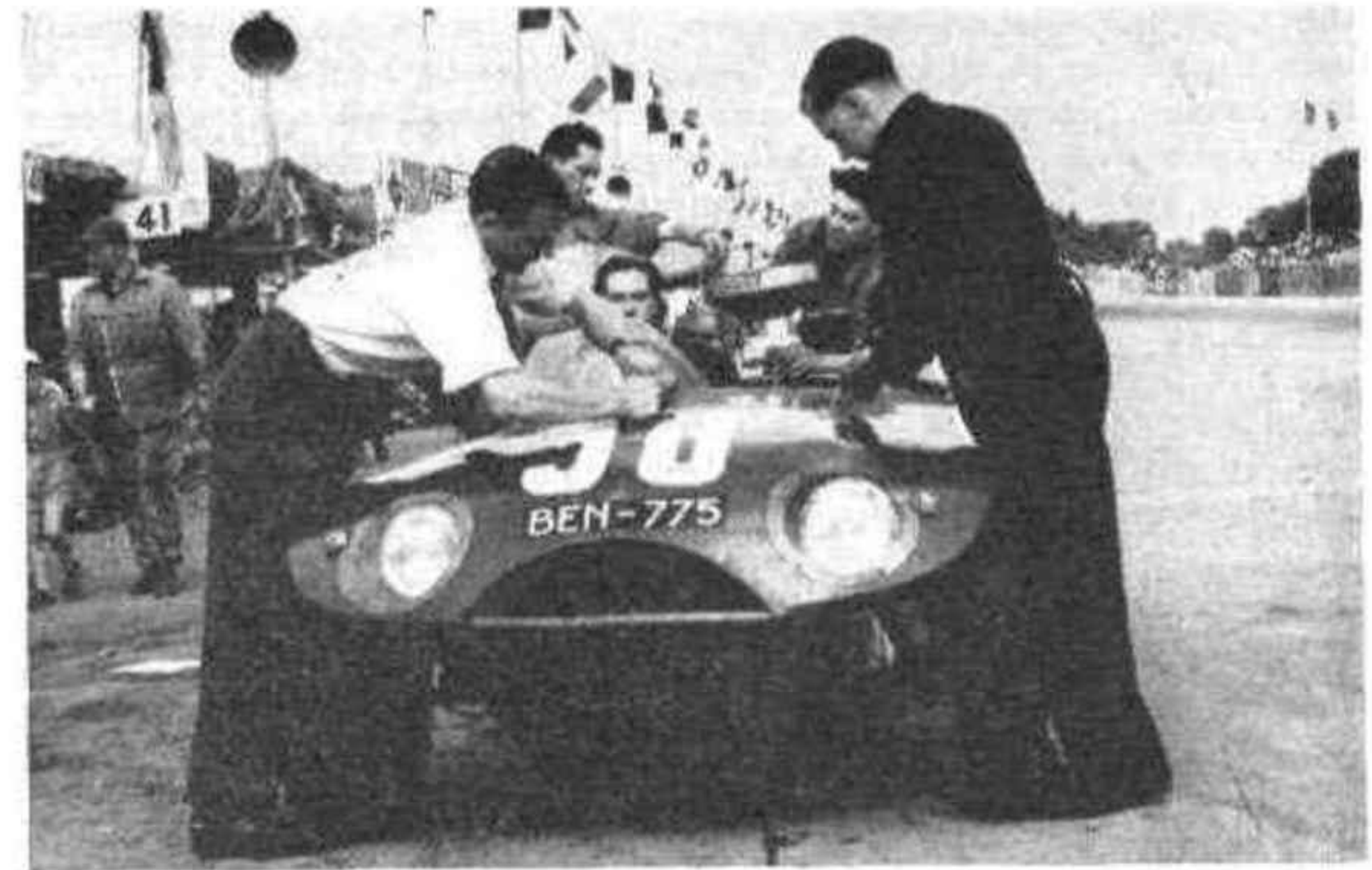
SUCCESSFUL HOME BUILD.—The strange-looking Horridge Special of J. Horridge and G. Trouis, comprising a Riley engine and a Wilson gearbox in a Jowett Jupiter chassis. It is being fuelled and oiled during a pit-stop during the Bol d'Or in which it finished a worthy second after a very regular run.
