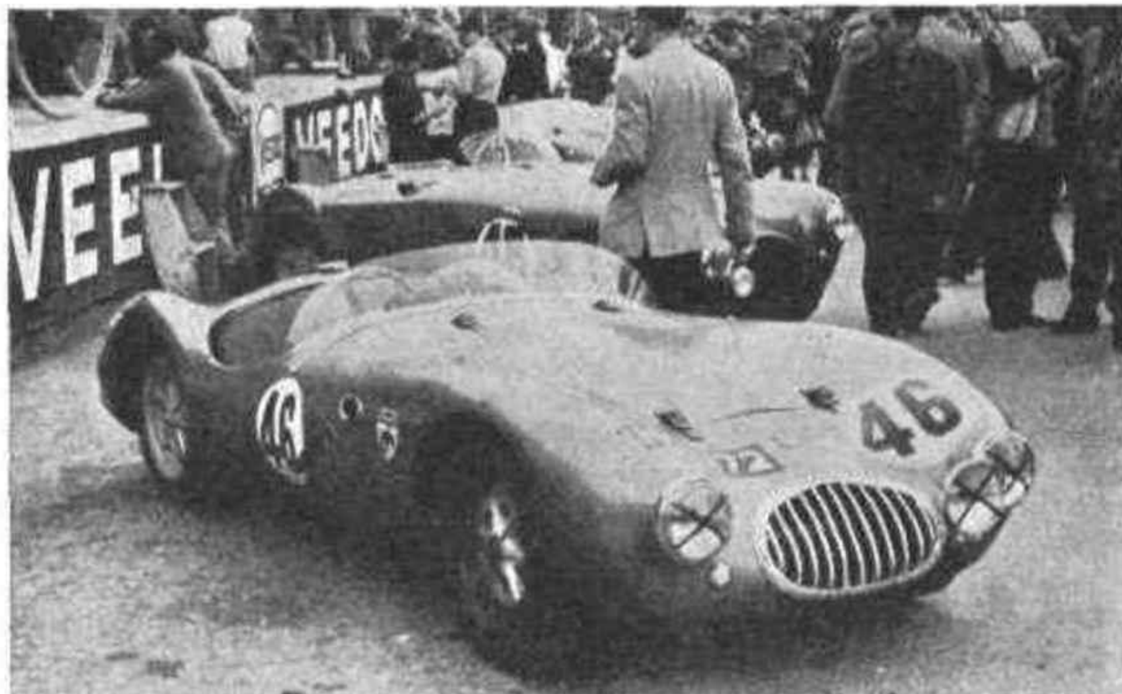
EXPERIMENTAL. —The new Kieft with plastic body aroused much enthusiasm for its neatness of line, but the 1,100-c.c. Climax engine was too new to last the 24 hours.
