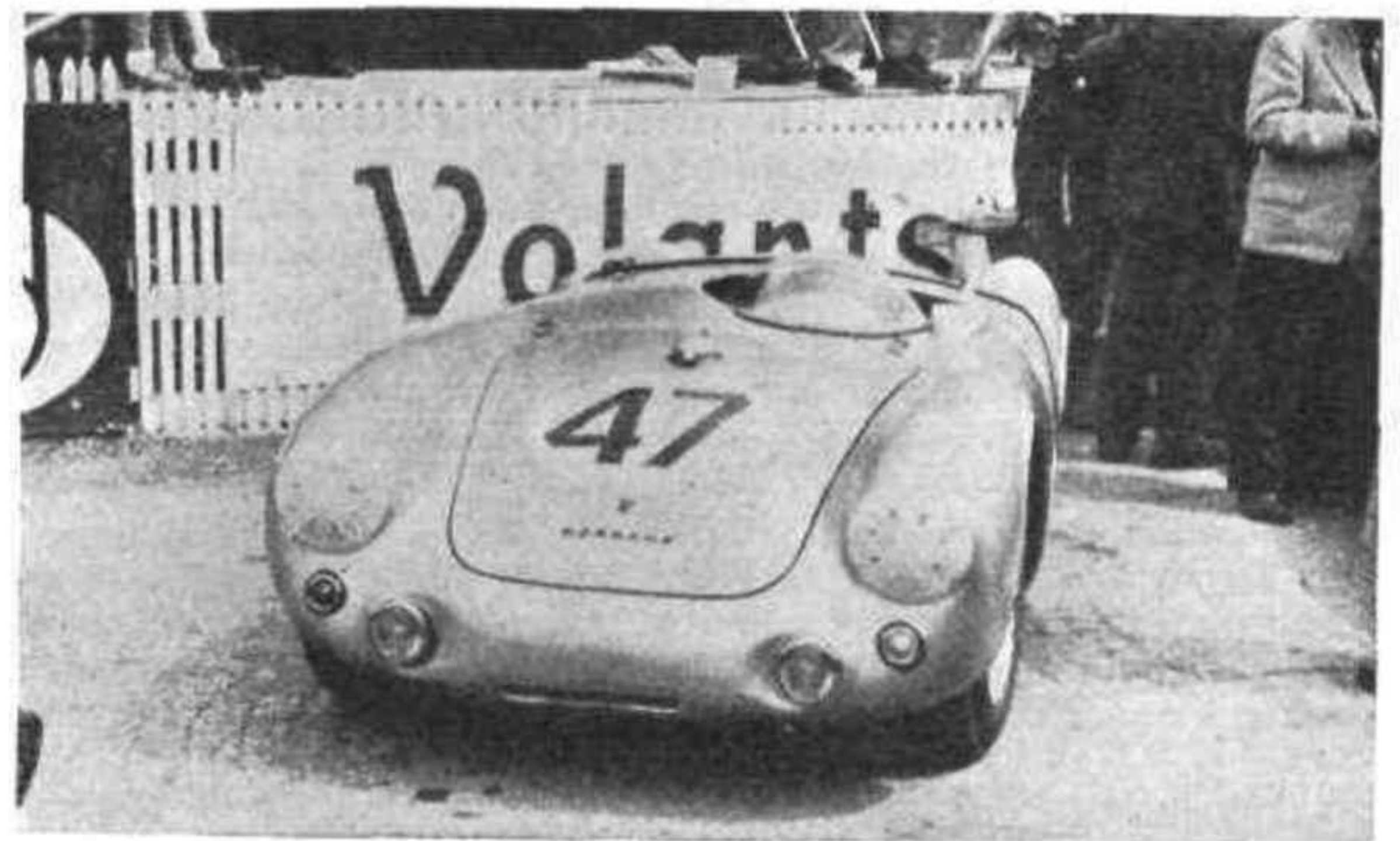
SMOOTH CONTOUR. —The 1,100-c.c. Porsche driven by Duntov/Olivier. Fitted with the four-o.h.c. engine it proved exceedingly fast, but suffered from gearbox trouble and only just managed to limp to the finish.
