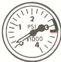
PC-1, PC-2 HYDRAULICS 3000 ± 200 NOMINAL PRESSURE
