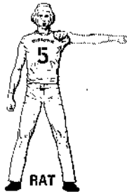
RAT RIGHT ARM STRAIGHT AHEAD, FIST CLENCHED; SWINGS ARM 90° TO SIDE. REVERSE THE PROCEDURE FOR RETRACT.
