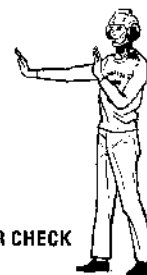
RUDDER CHECK RIGHT RUDDER IN RUDDER SWINGS RIGHT
