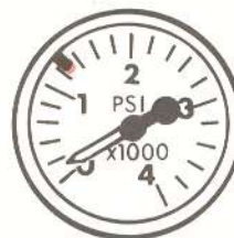
BRAKE ACCUMULATOR 1250 PSI MINIMUM PRESSURE
