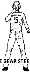
NOSE GEAR STEERING RIGHT INDEX FINGER POINTING TO RIGHT SIDE OF NOSE FOR RIGHT TURN AND VICE VERSA FOR LEFT TURN; OPPOSITE HAND POINTING TO NOSE GEAR.
