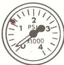
NOSEWHEEL STEERING 1100 PSI MINIMUM PRESSURE
