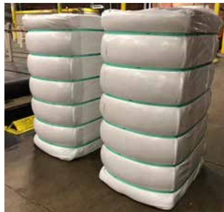
Figure 4.3 Bales of Nomex® staple with polypropylene wrapping
