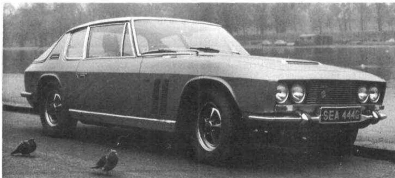
THE JENSEN FF of the late Sixties, early Seventies, not only had Ferguson four wheel drive but was the first road car with ABS. Like the Ferguson F1 car, the Jensen FF used the Dunlop Maxaret anti-skid system.
