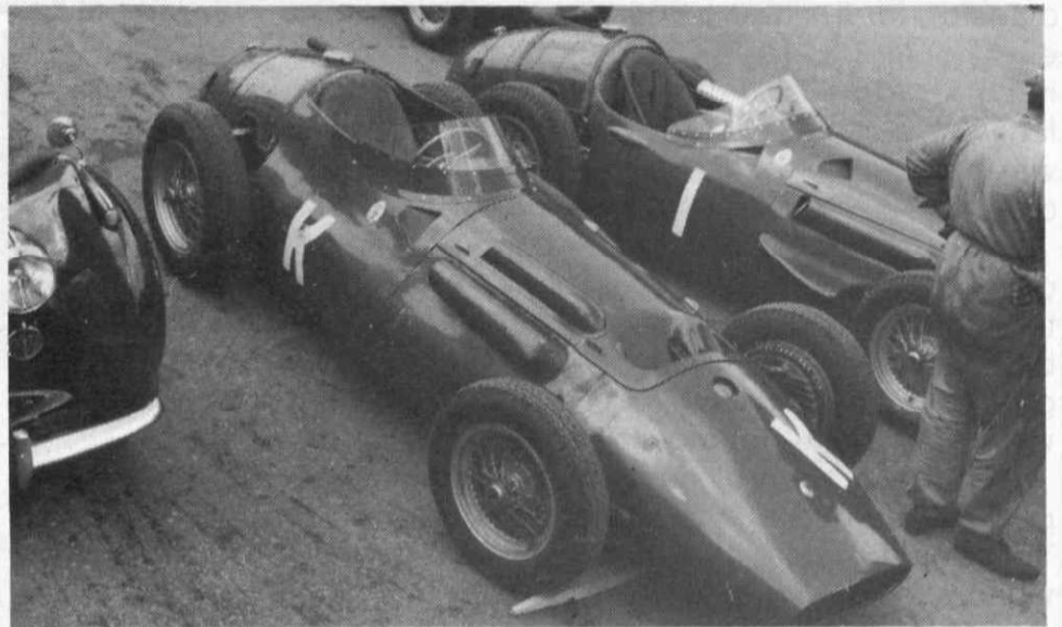
MASERATI 250F number 2501 in one of many experimental guises while it was in the factory team. In this 1956 photo it has a fuel injected engine, ducted radiator and high-sided cockpit. Behind is a more normal 250F.
