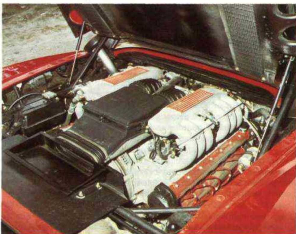
BIG as the block is, access is surprisingly good (above). Tubular chassis frame is visible in engine bay, but not in luggage compartment (below) whose misleadingly long cover reveals a rather irregularly-shaped space; room for two cases in the cabin, however.
