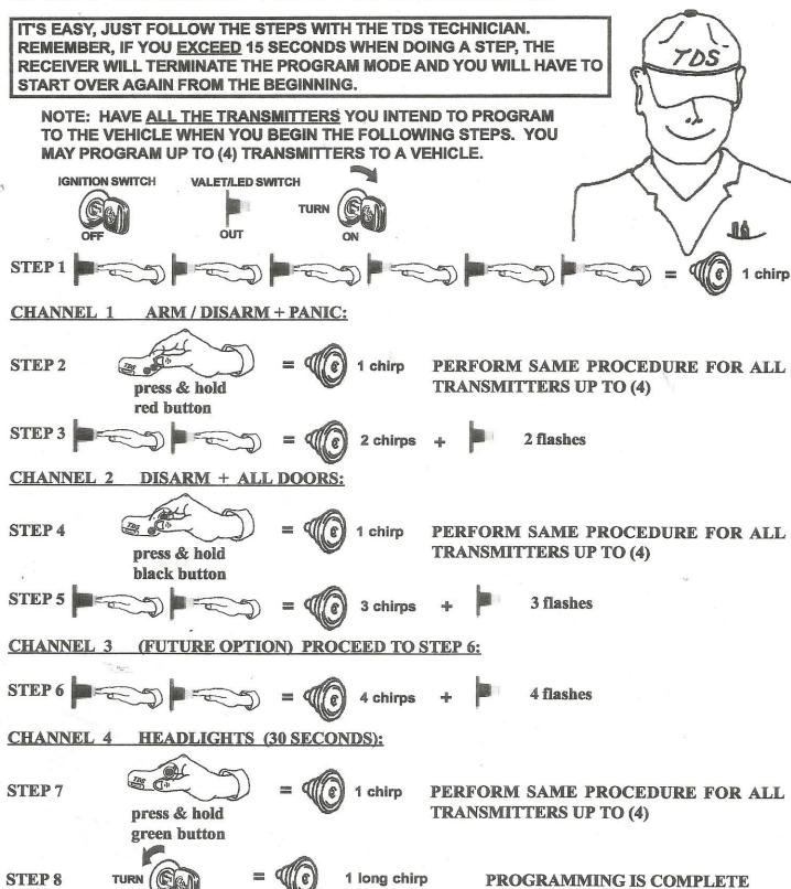
NOTE: SHOULD THE VEHICLE FAIL TO RESPOND TO A SINGLE BUTTON WHEN PRESSED, YOU MAY HAVE PRESSED THE WRONG BUTTON WHEN PROGRAMMING. IF THIS IS THE CASE, CLEAR THE TRANSMITTER CODES FROM MEMORY AND REPROGRAM THE TRANSMITTERS CORRECTLY.
