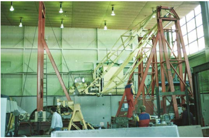
The 1985 trials on the Williams FW09 Formula 1 car. These early impact tests were between a mass swung on a pendulum and the solidly fixed nosebox structure
