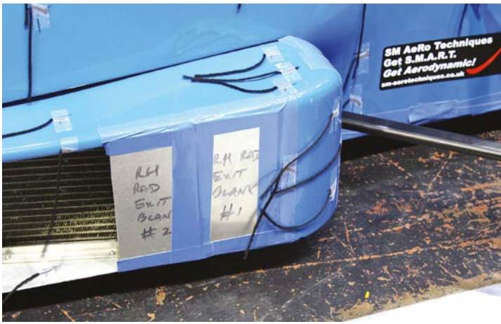
Blanking plates were fixed to radiator exit apertures to mask a quarter, then a half, of area
