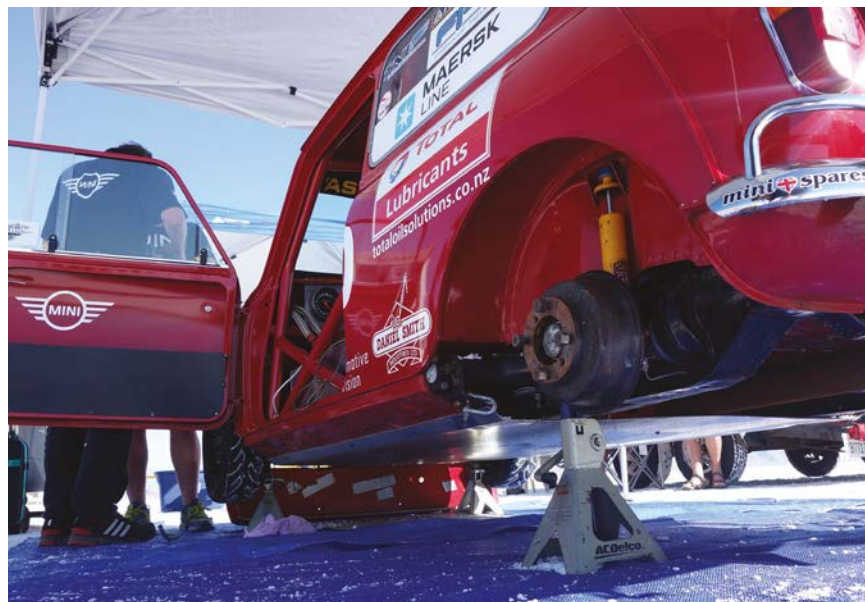
Suspension was the Hi-Lo adjustable rubber coned system that was used on all early Minis, but with new updated shock absorbers added. The body and chassis was near-standard, with a flat floor and undertray
