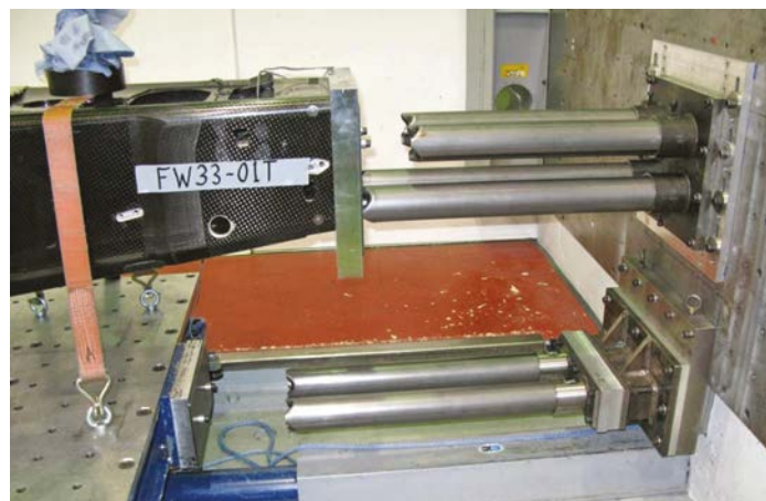
Chassis without nose is impacted into an FIA-specified tubular metallic energy absorber which provides a standardised 45g deceleration; no damage is tolerated.
