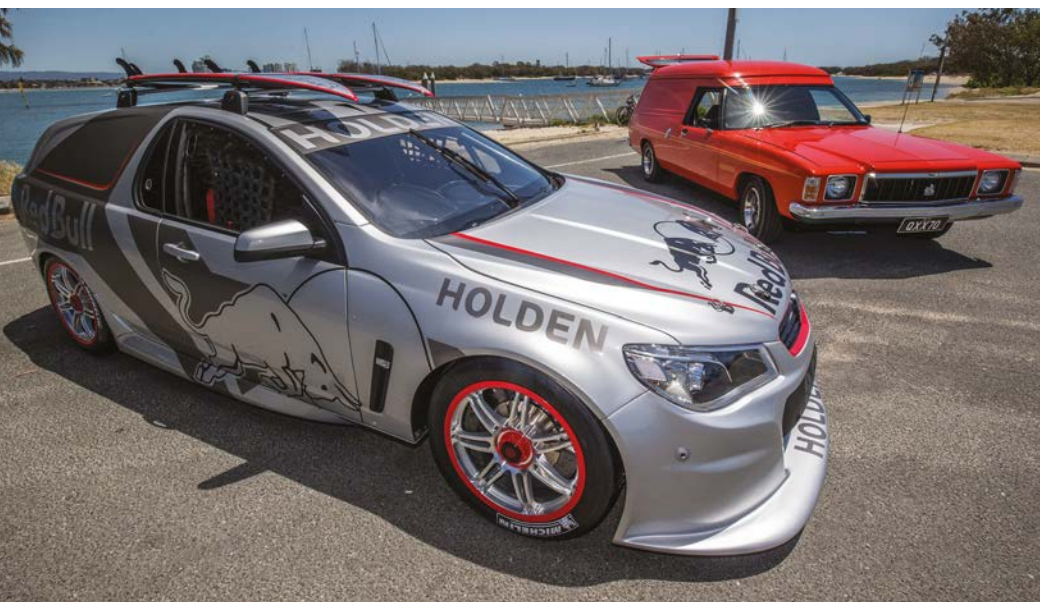
The Triple Eight passenger ride car is based on the 1974 Holden Sandman panel van, as seen in the rear of the picture. The modern version packs a 5.5-litre Holden V8 race engine, a paddleshift sequential gearbox, and two surfboards on its roof!
