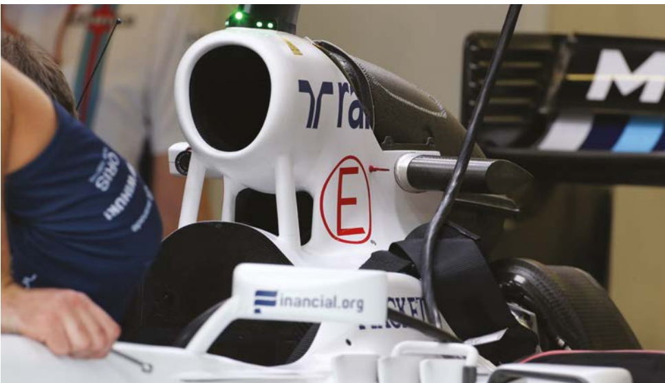
The roll hoop concept is a Williams trade mark and a continuation of that used on all of the team's designs since the FW35 of 2013, though it is highly likely that the design has been improved subtly since its introduction three years ago
