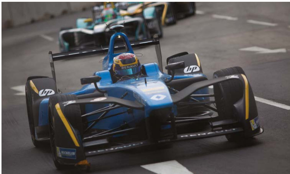
The Renault e.dams outfit is still the team to beat in FE. For season three it has switched to a direct drive transmission after previously using a two-speed gearbox, where first gear was only used for starts. It also has a very intricate cooling system
