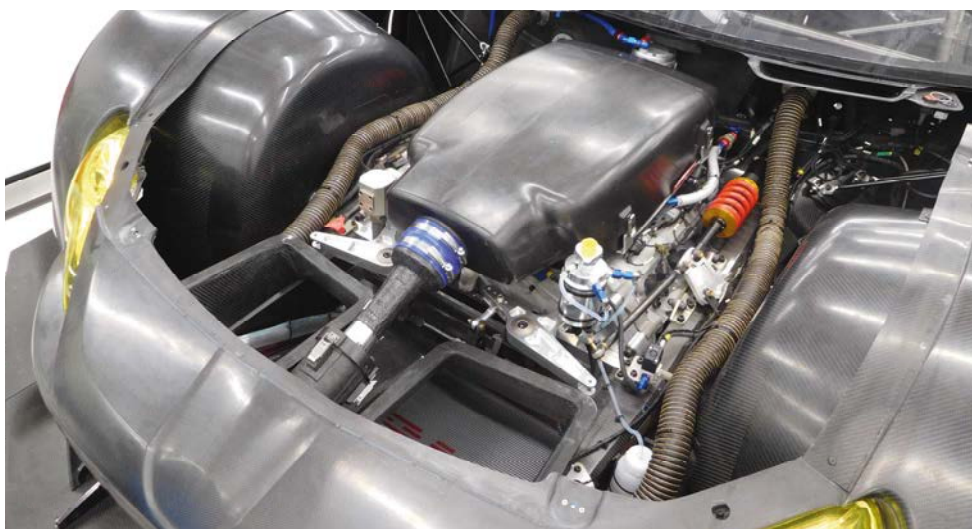
MC86B has its V8 engine mounted in the front yet in the Lotus Evora version of the MC the powerplant is mid-mounted, as it is in the production car. The Mother Chassis is designed to take all configurations, which gives the teams more car options
