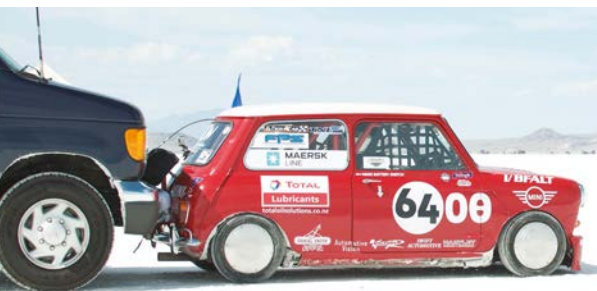
The Mini gets a nudge start, as wheelspin on the salt was a constant problem. To reach the high speeds attained with the standard gearbox some fairly long diff ratios had to be used
