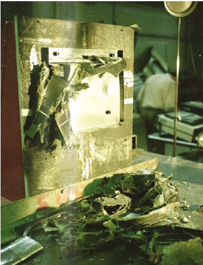
The pre-'85 nose test energy absorption requirement was 39kJ. This sample absorbed 50 per cent of that; 'meeting the requirement was not going to be easy,' O'Rourke said
