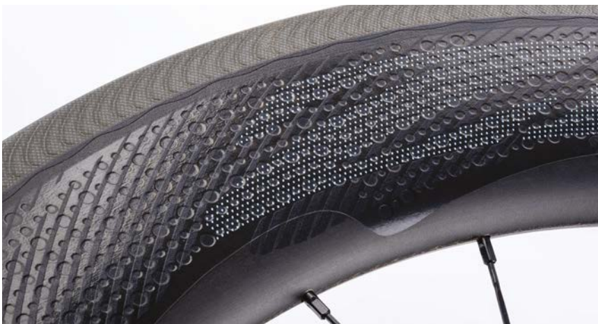
Dimpled surfaces are used widely in cycle racing having been pioneered by Zipp Speed Weaponry
