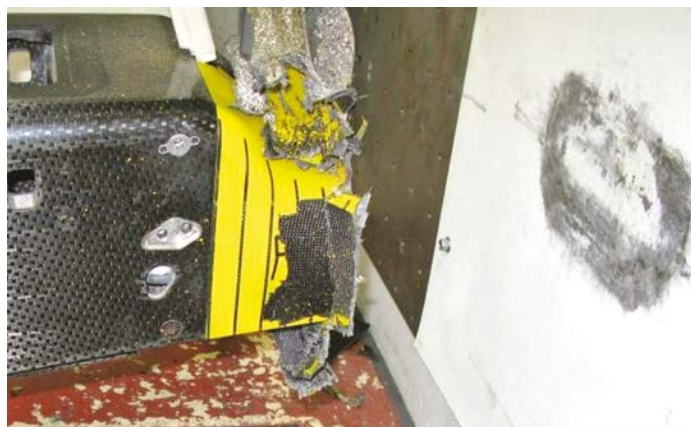
For the nose crush test the structure weighs 780kg and is impacted at 15m/s (88kJ). Six different deceleration parameters must be met, and no chassis damage is tolerated
