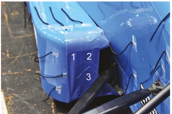
Strips of race tape were applied incrementally to the radiator inlet ducts of the Swift
