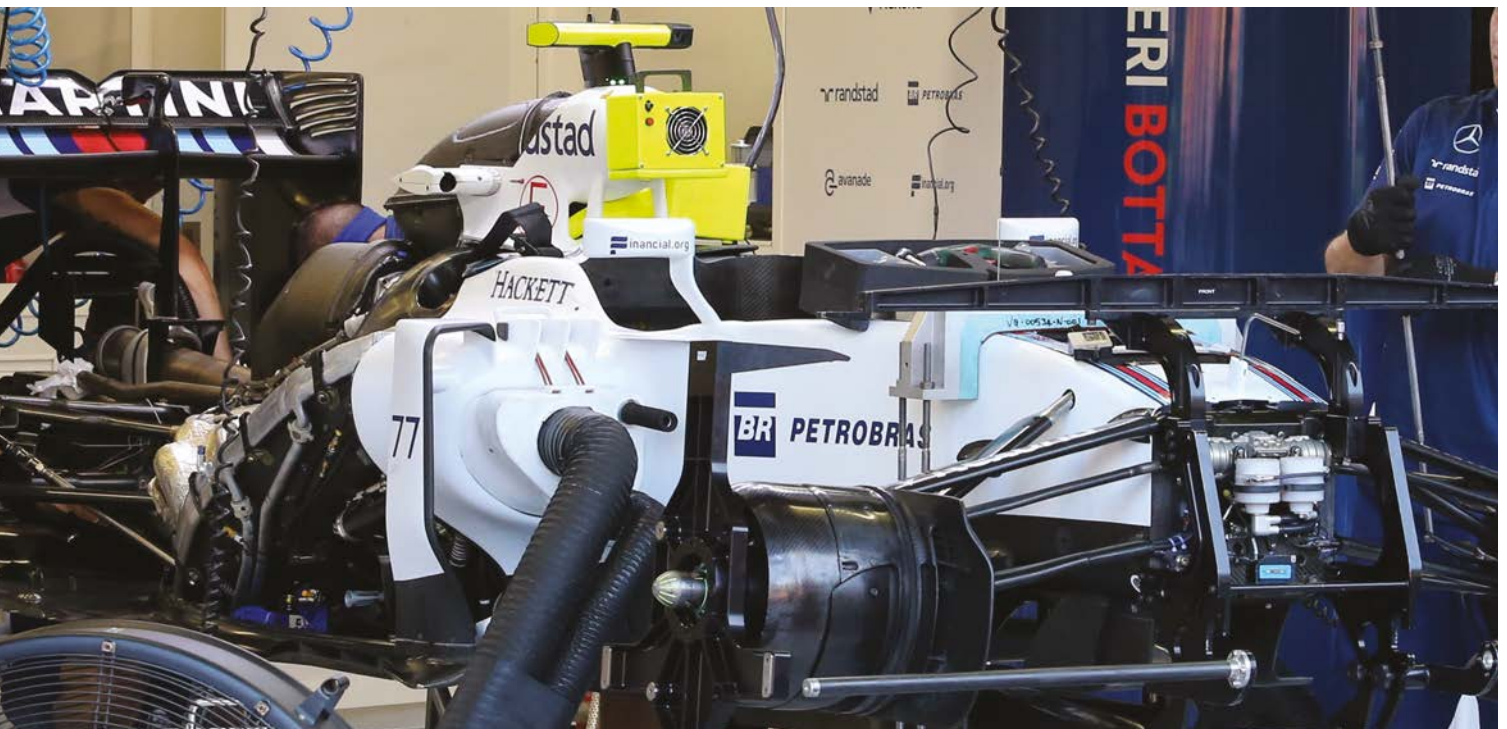
A half naked Williams FW38, showing pull rod rear suspension and the very neatly packaged cooling system. The car is in many ways an updated FW37, but with many refinements
