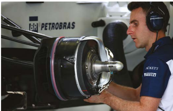
Williams has opted for the far less common AP Racing calipers on its FW38, using 6-piston calipers at the front end, 4-piston at the rear, and carbon discs and pads
