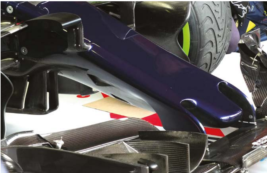
An inverted trailing edge blowing device as used on the Toro Rosso S duct sited in the nose of the 2015 car
