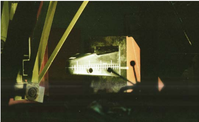
The time is up for this F1 part: the pendulum is about to impact the FW11 nose-box
