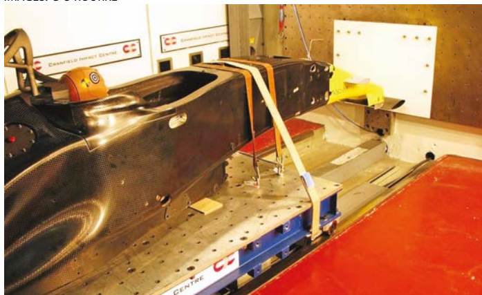
Here the Formula 1 chassis with nose attached is impacted into an immovable barrier
