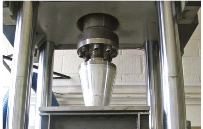
The panel penetration test rig with its solid metal cone, designed to act as a nose-box
