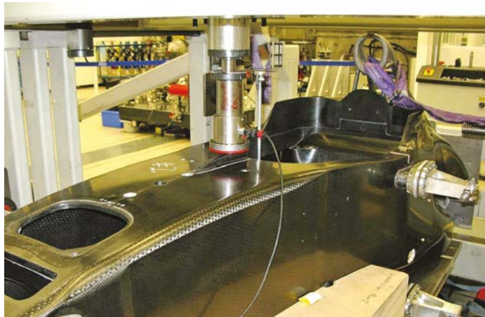
The front roll protection structure on the Williams chassis is subject to a 75kN push test
