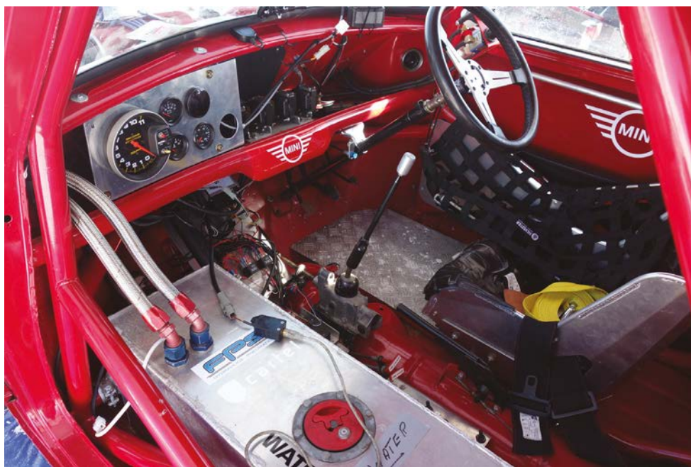
Cooling was a headache and the team fabricated this huge heat exchanger that sat within the car instead of relying on a conventional air to water radiator – it was filled with ice minutes before each run. Otherwise it's a classic race Mini interior
