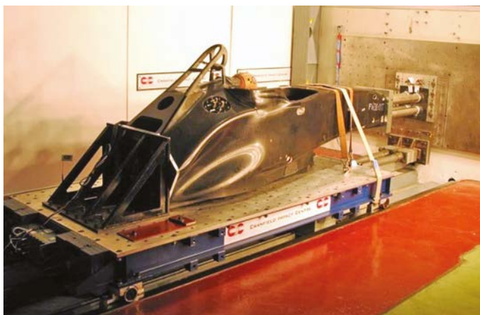
The 2016 test chassis is ballasted to 900kg, which includes the water-filled fuel tank, and is then propelled at the impact absorber on a trolley at 15m/s, which equates to 101kJ
