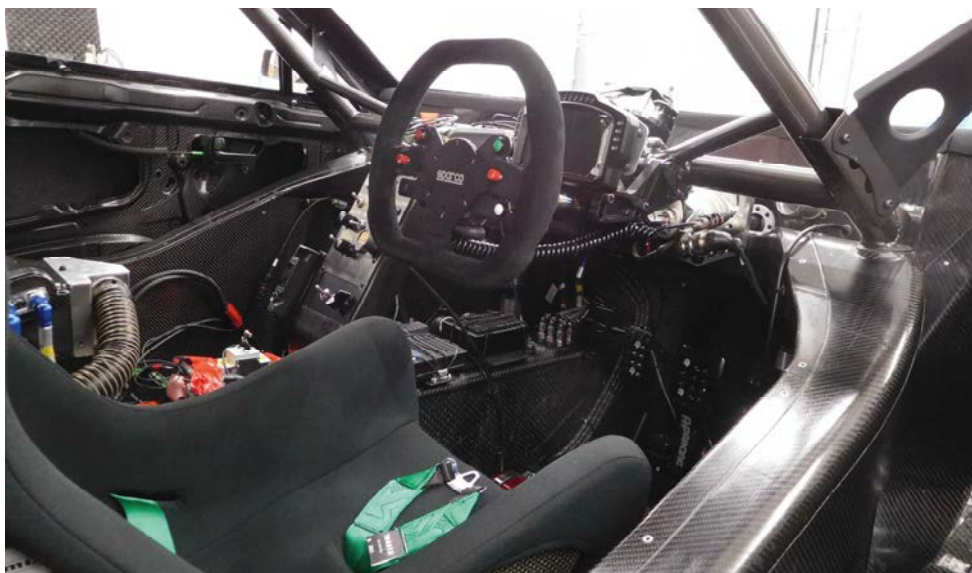
The carbon fibre tub is fitted with a very sturdy steel roll cage. Dome says that its torsional testing shows that the chassis of the MC86B is actually stiffer than its big-brother DTM-based GT500 cars. This is largely due to the thicker bulkheads used
