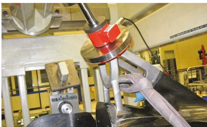
The additively-manufactured titanium main roll hoop undergoing its 120kN push test
