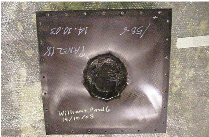
Aftermath of the panel penetration test; 500mm by 500mm panel was clamped down
