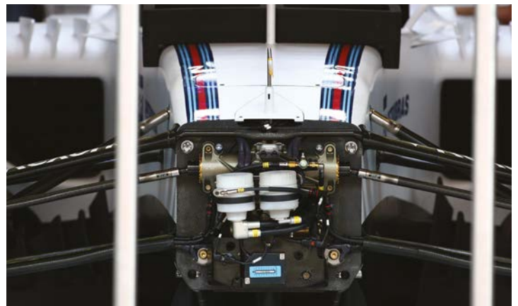
The front bulkhead and the steering rack. The suspension layout is essentially the same as the FW37, with pushrod actuated torsion bar at the front of the car and pull rod at the rear
