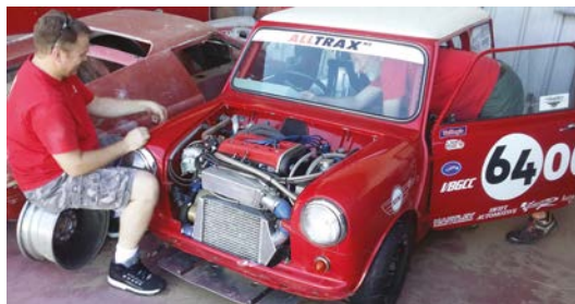
Much of the extra power was found through the use of the turbocharger, but it was a major challenge to eliminate the harmonics from the three-bearing crankshaft at over 10,000rpm
