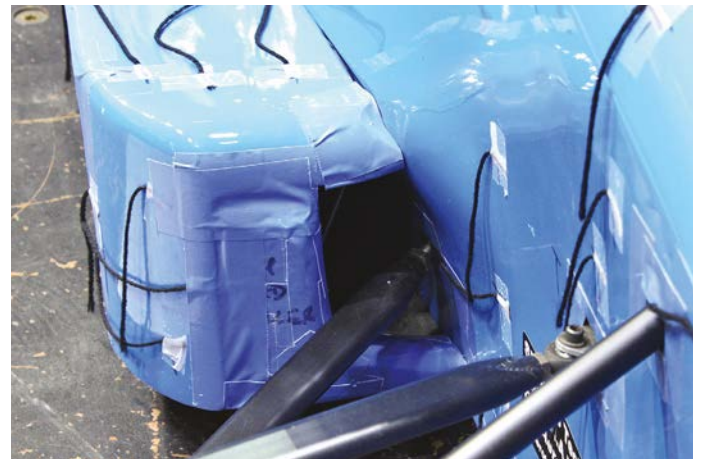
Would these shaped inlet reducers prove more efficient than the simple race tape?
