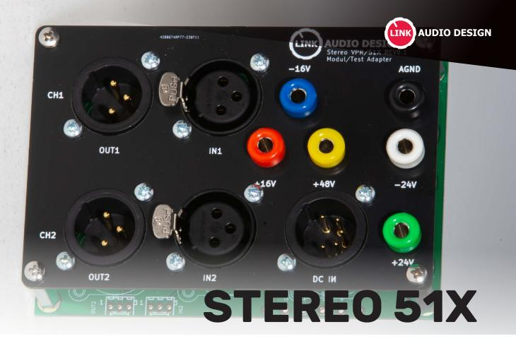
This updated STEREO 51X Extension is a complete set of PCB's, parts and components required to build an Extender for testing and calibrating 51X MONO and STEREO series modules. In addition you can use our STEREO 51X Stereo Modul Adapter to get your voltages directly out of the Rack via 4mm Hirschmann connections.
