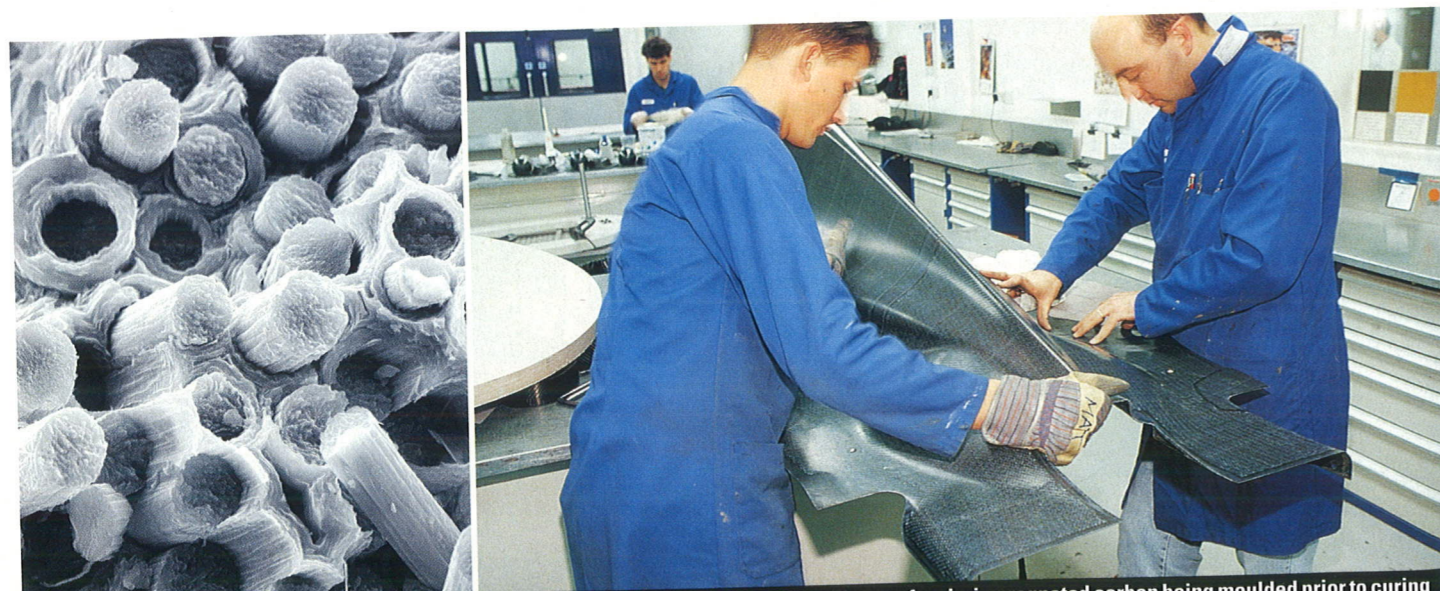
Above left Tight-packed carbon fibres seen under an electron microscope Above right Sheets of resin-impregnated carbon being moulded prior to curing
