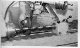
FIVE-BEARING camshaft ready for final grinding operation.
