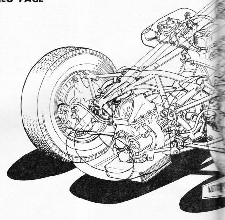
The car rides on wide-base magnesium wheels, with  $5\frac{1}{2}$  ins. rims, shod with  $4.50 \times 13$  ins. and  $5.50 \times 13$  ins. Dunlop tyres at the front and rear respectively. The disc brakes are outboard all round with
