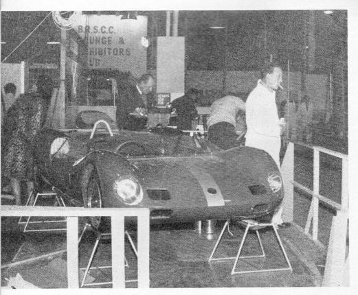
THE NEW Elva Mark VII sports car, with rear-mounted Coventry Climax engine.
