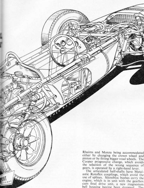
Lockheed twin master cylinder operation and Cooper-Mini type calipers. The steering is by a Cooper rack and pinion gear.
