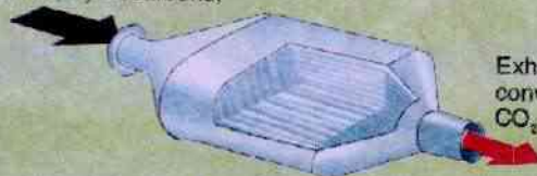
Fig. 14.5 Catalytic converter used in automobile vehicles.
