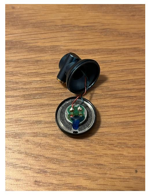
Twist the face cover to spiral wind (corkscrew) the wires (loosely). The wires will fit into the shell better and less risk of pinching them as well.
