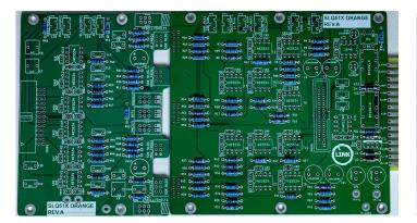
After Placing and Soldering all Resistors, we solder the next bigger parts like IC-Sockets and small Capacitors, like 37x100nF and 16x22pF
