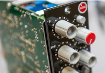
After finishing try to run an Audio Signal thru the Unit and try all switch modes, if everything works fine. If you have a bump when switching the Low or Highcut Filter, don't worry these filters need to be calibrated to have the right level. Try also if all Gains and Frequency Pots are working. You can do that either in the measure software or with Audio Signals. In the next step we will calibrate this wonderful Equalizer.
