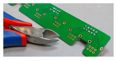
After we shortened all the pins we install all pots on this board at the same time. Get all pots on the PCB and solder just one pin in the middle and press the POT as much as possible on to the PCB. After Soldering one Pin make sure the alignement of the pot is flush and straight. You can check that with printed silkscreen on the PCB. Check also if the GAIN-Pots are center detent and the ,Q' is at the right place.
