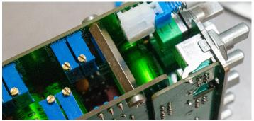
Now it's time to add the Frontpanel to complete the Equalizer. Use the spacers and the M3 Nuts to finish it. The Caps for the Knobs are sorted as following:
