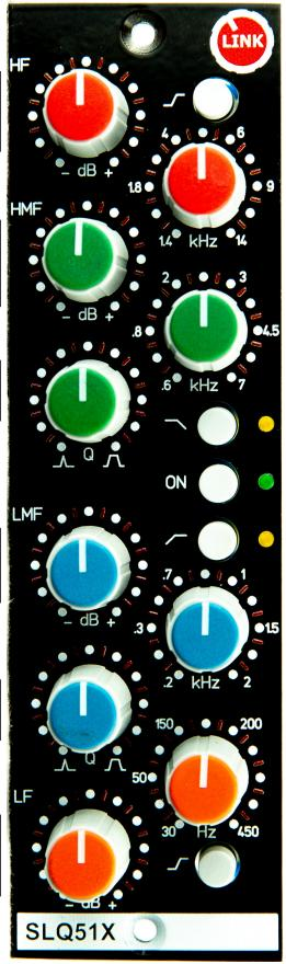
This Button switches from BELL-MODE into SHELF-MODE of the HF-Band
