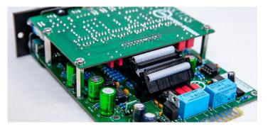
Now we install the upper subboard by holding it angled and connect the ribbon cables at the same time.
