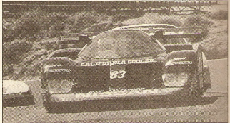
The rule changes favour the Electromotive team's Lola T-810, which is powered by a stockblock, 3-litre Nissan V6 engine turbo jointly developed by Nissan and Don Devendorf's organisation.
