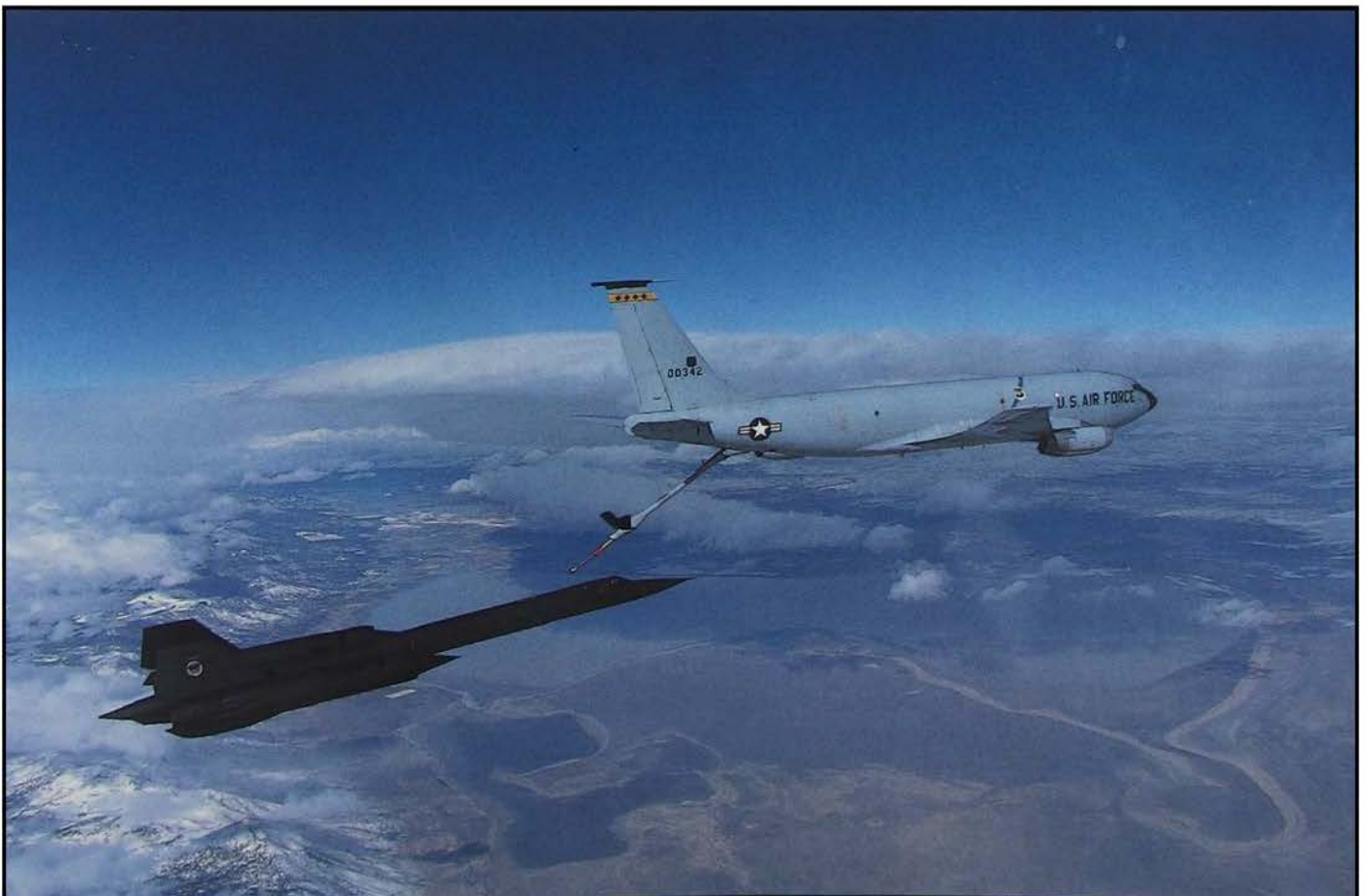
Sled pilot eases the jet forward for crucial contact. When the Blackbird is in position, the tanker's boom operator will place the refueling nozzle into the SR-71's receptacle.
