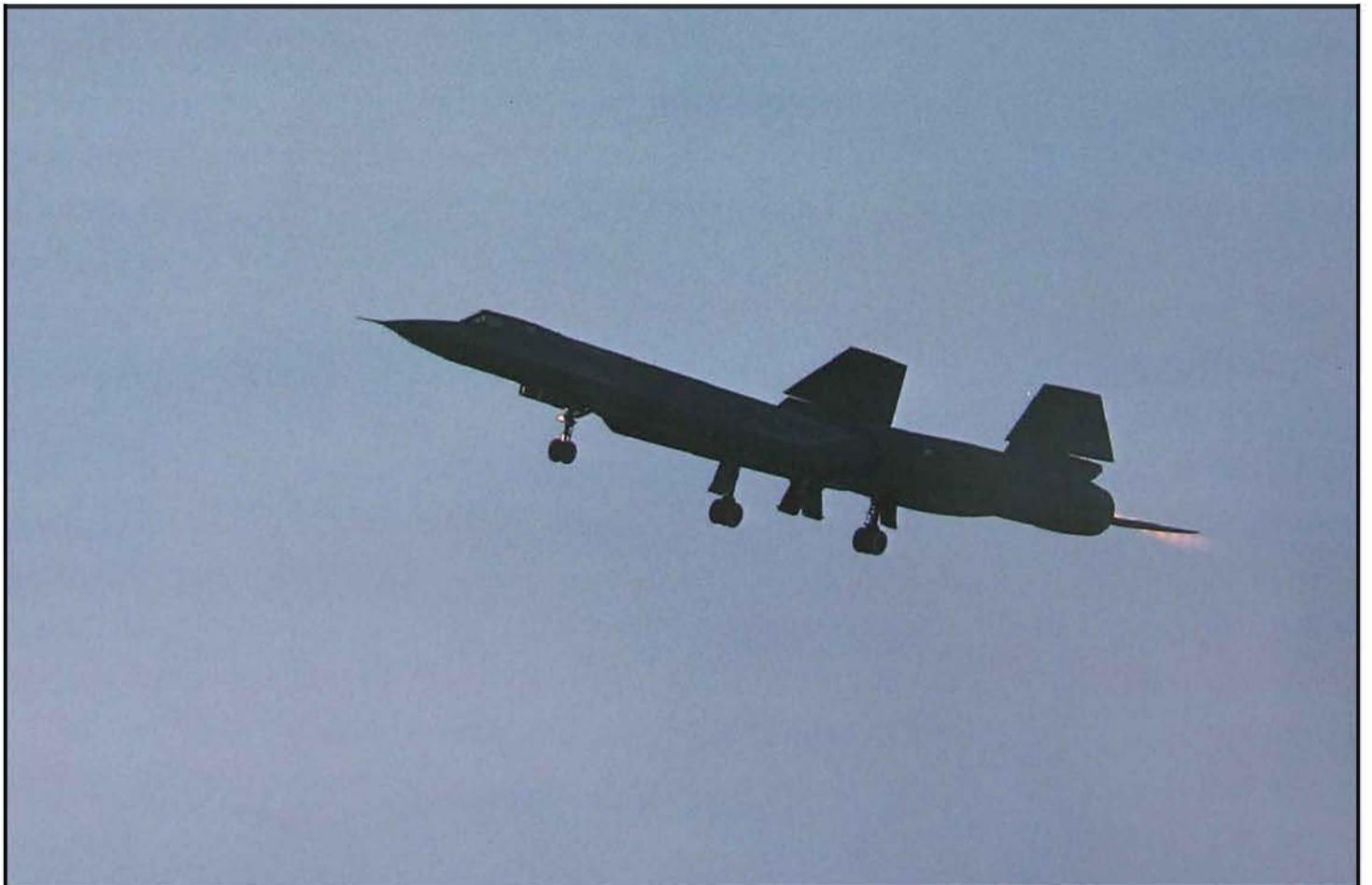
The simulated single engine pass, a crowd favorite at airshows. Large rudder deflection was necessary with one engine in idle and one in full afterburner.
