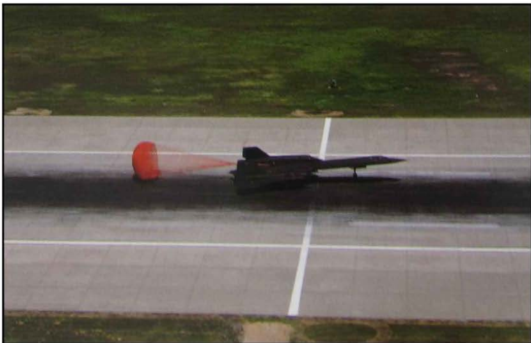
Large drag chute was deployed on every landing, greatly reducing the landing distance.
