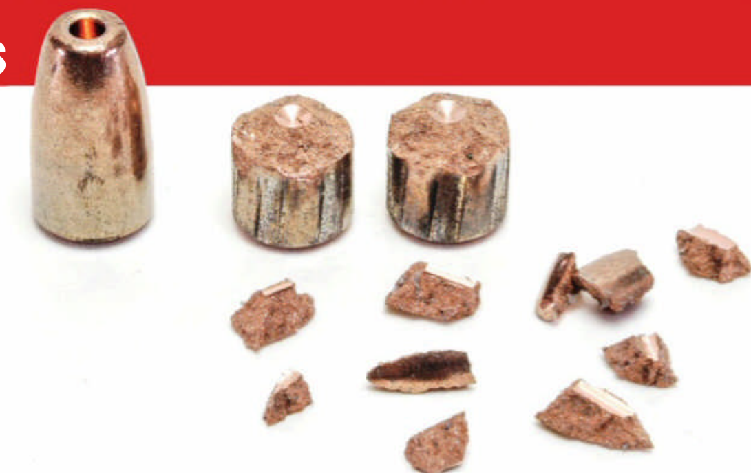
▲ When fired into bare synthetic gel blocks, the Reduced Ricochet bullets produced fragments that quickly veered off from the base while the base penetrated deeply.
