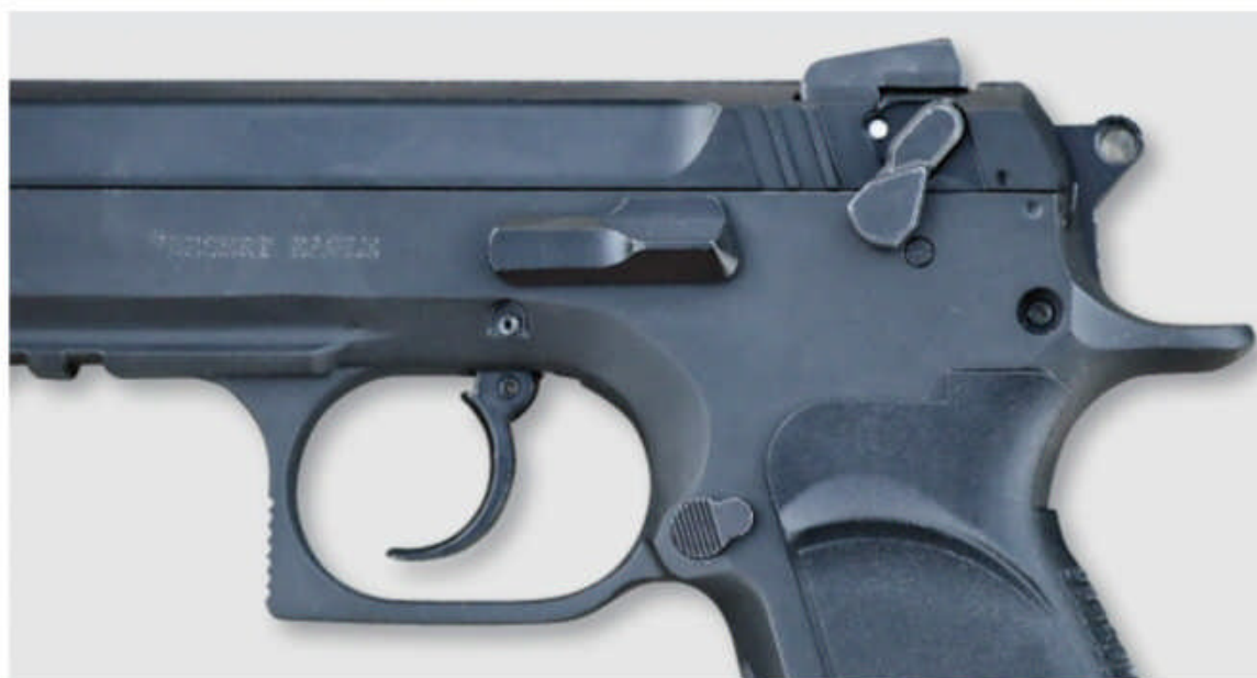
▲ The Baby Eagle III's control layout is quite simple. There's a large slide-lock lever, a decocker and a reversible magazine release button.
