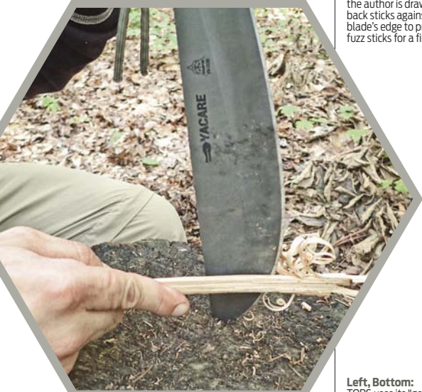
Left, Bottom: TOPS uses its "go-to" 1095 high-carbon steel with a very attractive Acid Rain finish on the entire Yacare blade.
