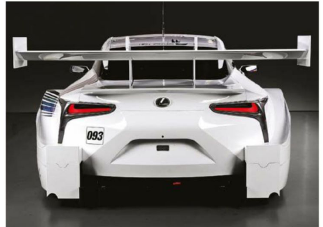
The big change for the LC500 is the 25 per cent cut in downforce which is the result of the new regulations. TRD believes it will claw some of this back in 2017
