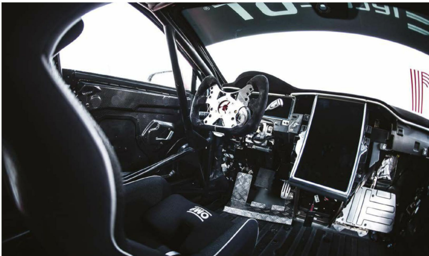
The Tesla is all FIA-spec racecar on the inside with a full rollcage and all the necessary gubbins. The steering wheel is the same as that used in the DTM. Electric GT is currently looking for drivers to take part in the series
