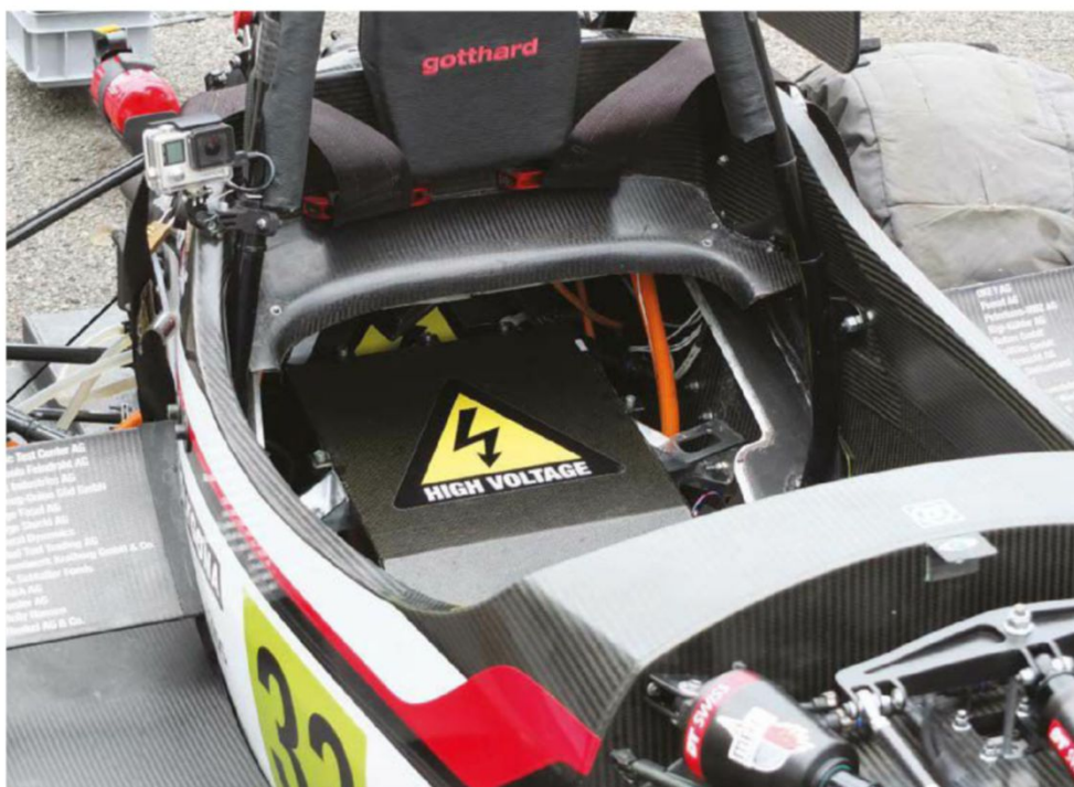
The ETH Zurich Formula Student car makes use of two lithium polymer cells with high energy and power density. The balance between power density and energy density is a matter of much debate in electric vehicle development circles
