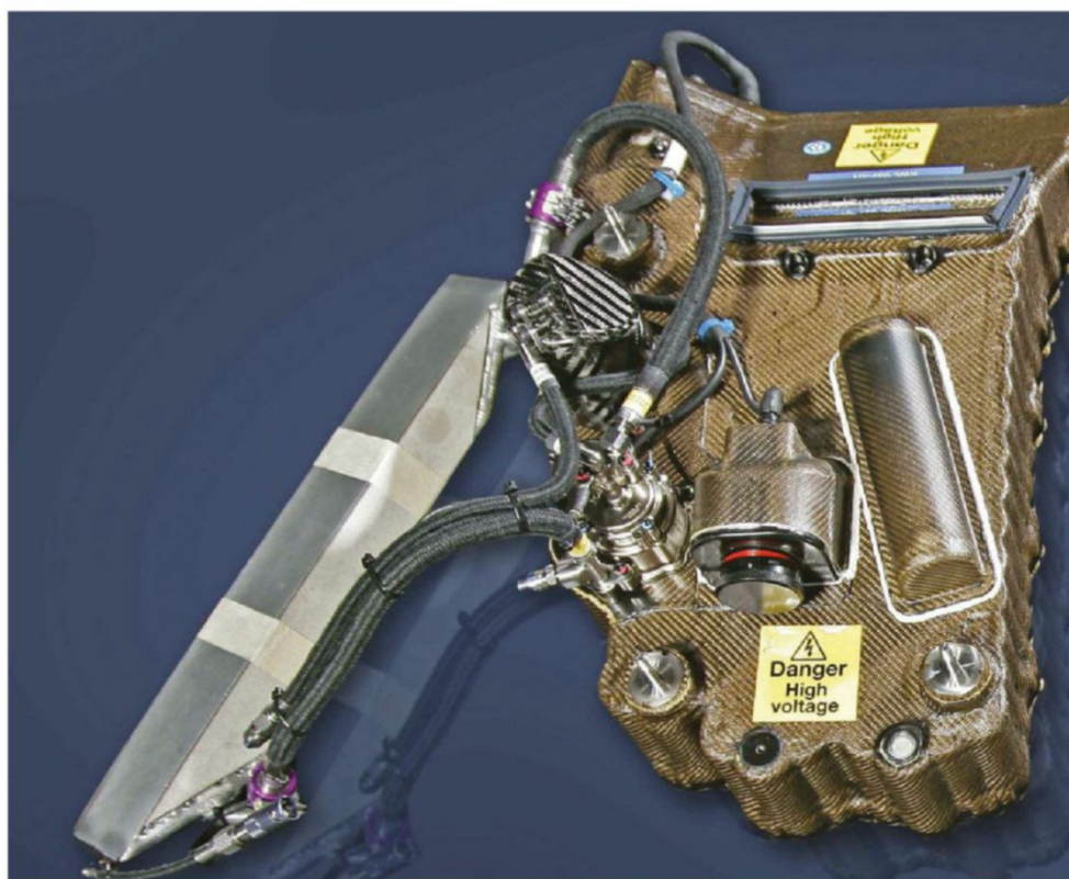
The 2009 Mercedes F1 battery pack used cylindrical cells derived from a production car. These cells are the most commonly available technology, but other packaging solutions, such as pouch and prismatic, are becoming more prominent in racing
