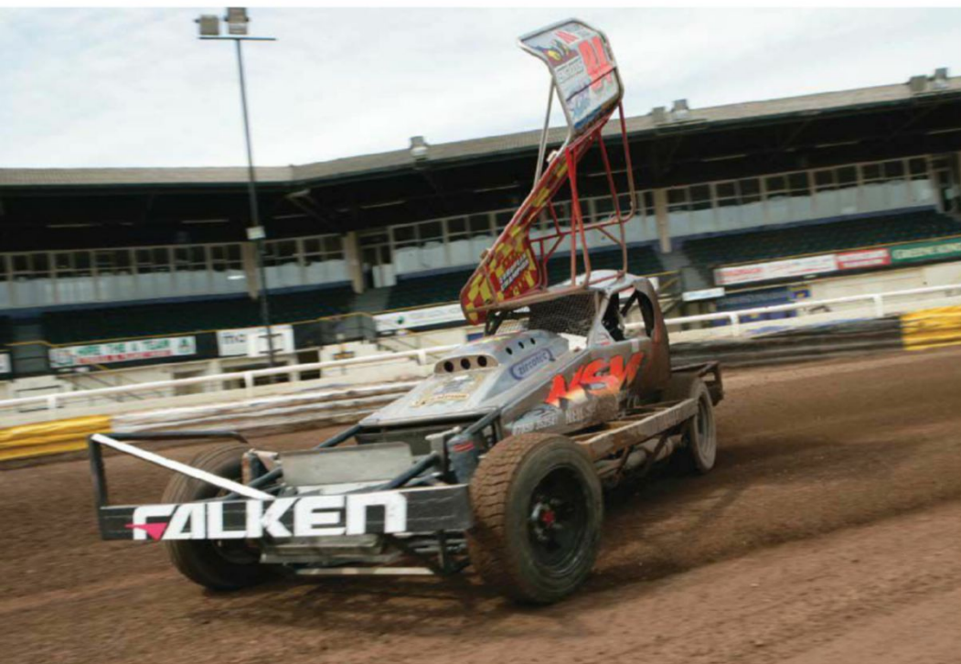
UK equivalent to a Sprint car is called a stock car. This one has an aerodynamic package optimised for racing on shale
