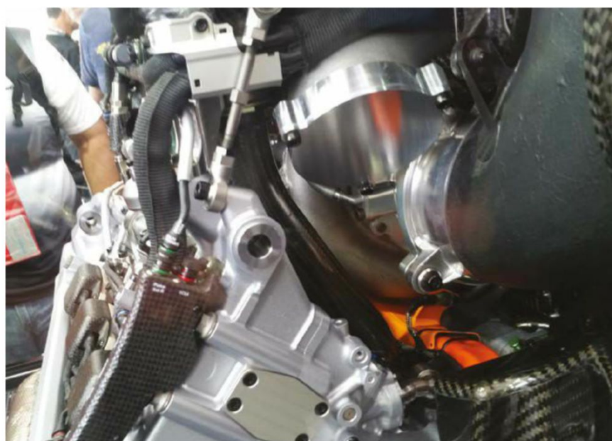
On the RA616H the turbine is mounted at the rear of the block, while the compressor is situated in the V of the engine about halfway along the ICE, right above the central pair of cylinders and underneath the plenum
