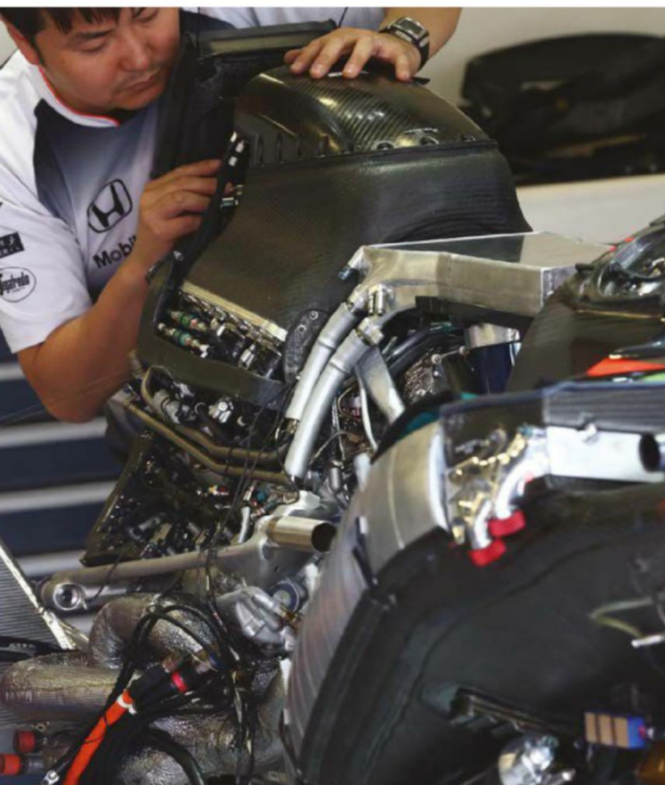
Left side of power unit from rear. The 2016 PU is in reality an update of the RA615H but Honda tells us almost every single aspect of it has been improved in some way
