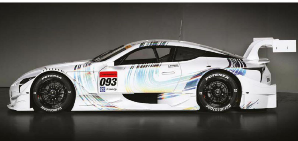
With the new for 2017 regulations the mechanical elements of the car remain largely unchanged, but the overall car length has been reduced from 4775mm to 4725mm, with all of this coming from a 50mm trimming of the car's front overhang
