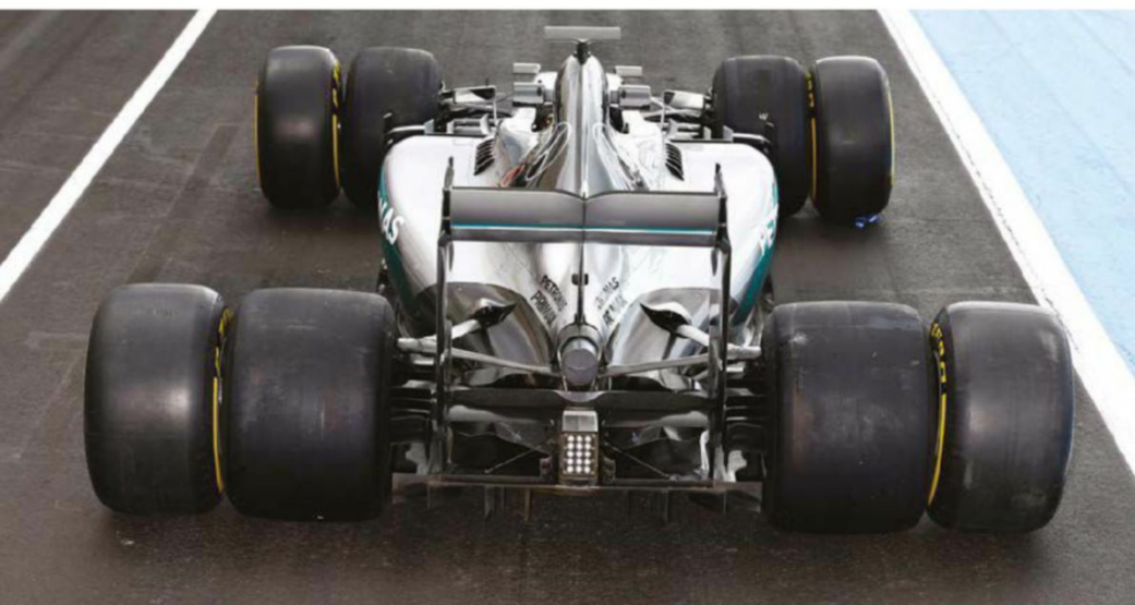
The new Mercedes eight-wheeler has been turning heads ... Okay, not quite. But this image does give a very good indication of the difference between the 2016 spec tyres (on the outside) and the new-for-2017 tyres, that are affixed to the racecar
