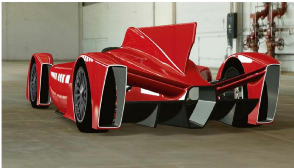
There is no conventional rear wing but there is a set of wing profiles between the rear impact structure and the rear wheel pods. Earlier versions of the design had a centreline downwash generating or CDG wing, similar to that once proposed for F1
