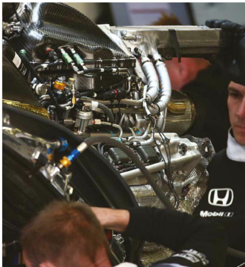
A view from the left side. The key to the success of the update is the new larger turbine which allows the MGU-H to function more effectively and also raises the deliverable power of the unit significantly
