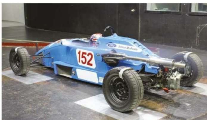
Wake from the mirrors was quite pronounced and these will certainly be causing drag
