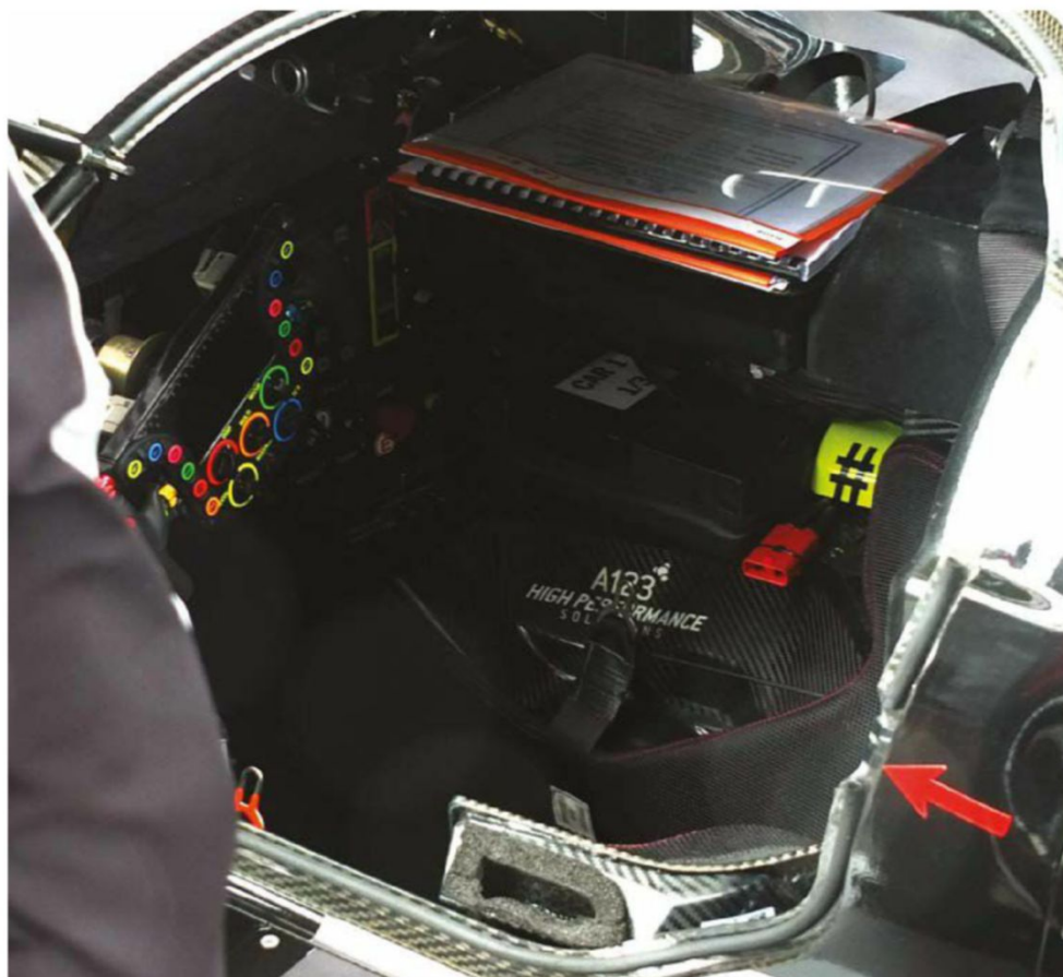
The Porsche 919 Hybrid LMP1 car packs bespoke A123 Systems cells located in the cockpit. With a need for better power density in sports prototypes, rather than energy density, some have questioned its relevance to developing road car EV tech
