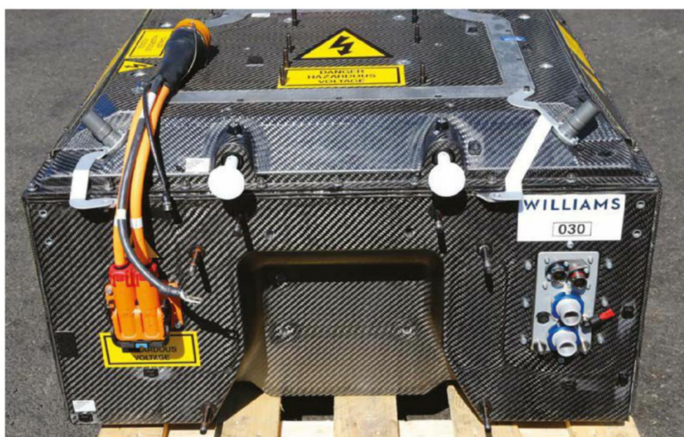
The current Formula E battery pack is made by Williams Advanced Engineering. Williams produces 44 batteries for FE each season. Each battery pack weighs some 320kg so it accounts for a fair portion of the overall weight of the Formula E racecar
