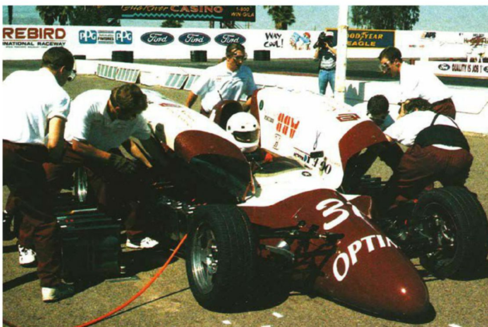
A Formula Lightning pit stop – for a planned battery replacement – back in 1997. This US-based series, which was ahead of its time in many ways, was all about managing the life in the battery pack so as to have enough juice to race to the finish
