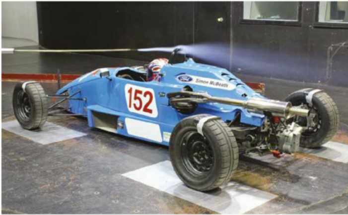
The roll hoop clearly has an effect on the airflow but as a safety device it cannot really be altered. But could changes to the bodywork around the hoop help with reducing the drag?
