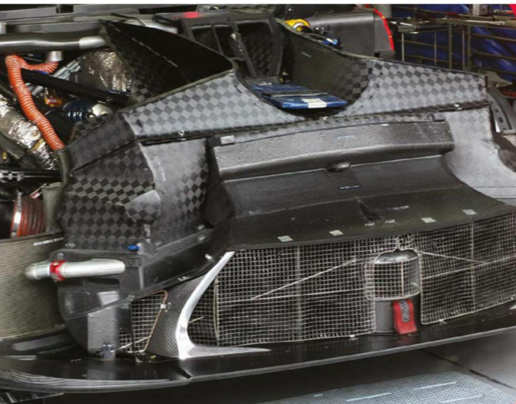
One of the weaker aspects of the RCF has been its cooling. While the internal ducting was not restricted in the regulations the positioning of the inlets and the heat exchangers were fixed. Improving cooling for the new LC500 has been a priority
