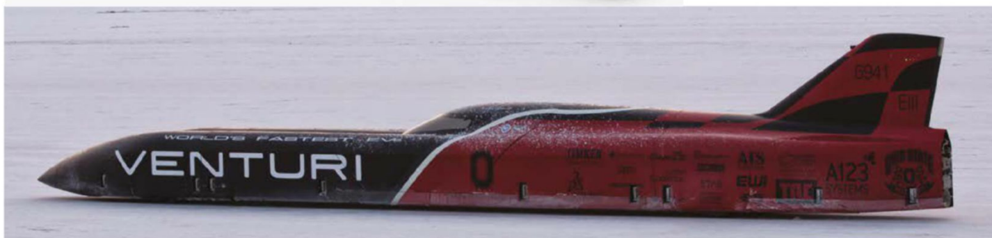
The Venturi Buckeye Bullet 3 (above and below) broke electric landspeed records in 2015. The all-electric record breaker ran on lithium-ion phosphate cells, due to their excellent behaviour under extreme temperatures
