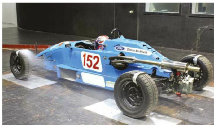
The smoke plume revealed that, usefully, the front wheel wakes partially impinged on the rear wheels, which would help reduce drag caused by the rear wheels and tyres
