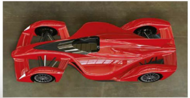
Under the skin the Dome is conventional, the racecar utilising double wishbone suspension all round with pushrod actuated dampers at the front and the rear
