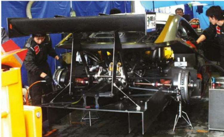
The 2015 RCF from the rear. The suspension is a relatively free area for modification, but all cars must use common uprights. Geometry is changed to suit tyre developments in-season
