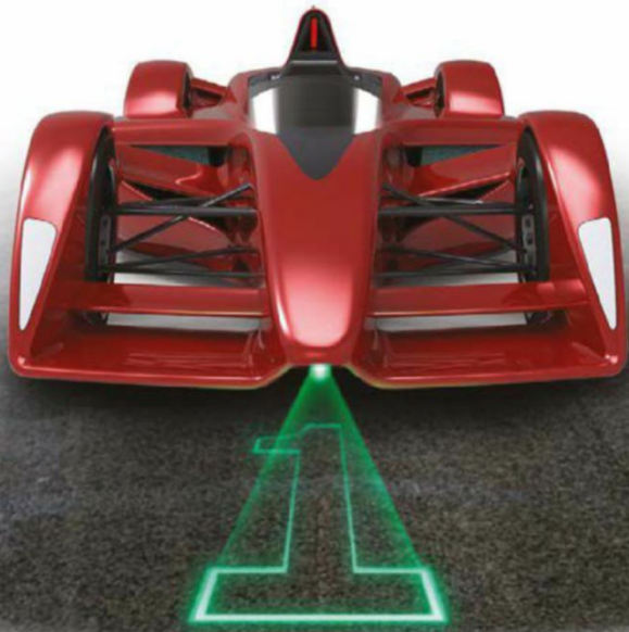
One of the more quirky ideas Dome had for its Formula E was the car number, or a car's position in the race, being projected on to the race track in front of it as it competed. This was to be done with a laser projector
