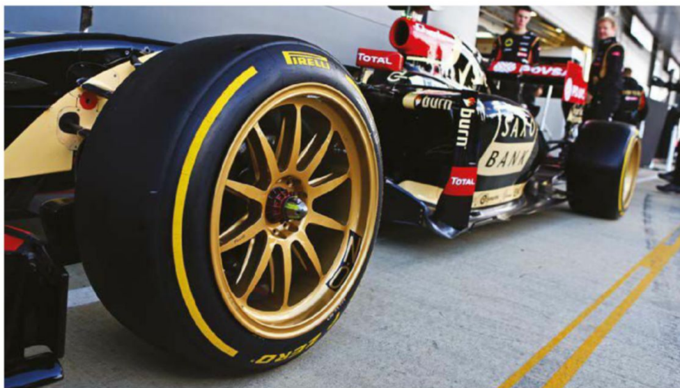
There had been talk of a switch to 18in rims and low profile rubber for 2017, driven in part by Michelin which had been considering entering F1 once again. This has now been shelved, although Pirelli did produce some tyres to this spec (above)
