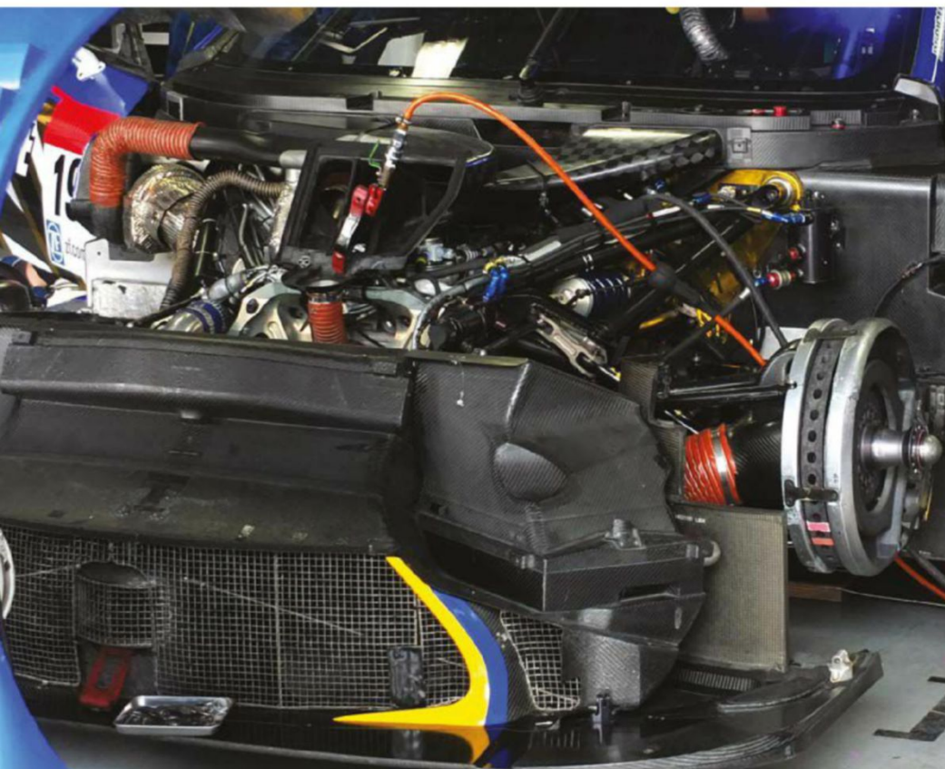
Engines in GT500 are relatively free and unlike its DTM cousin it has a modern engine formula with an extremely advanced 2-litre turbo in-line 4-cylinder unit featuring direct injection. Toyota also develops a version of its engine for Super Formula
