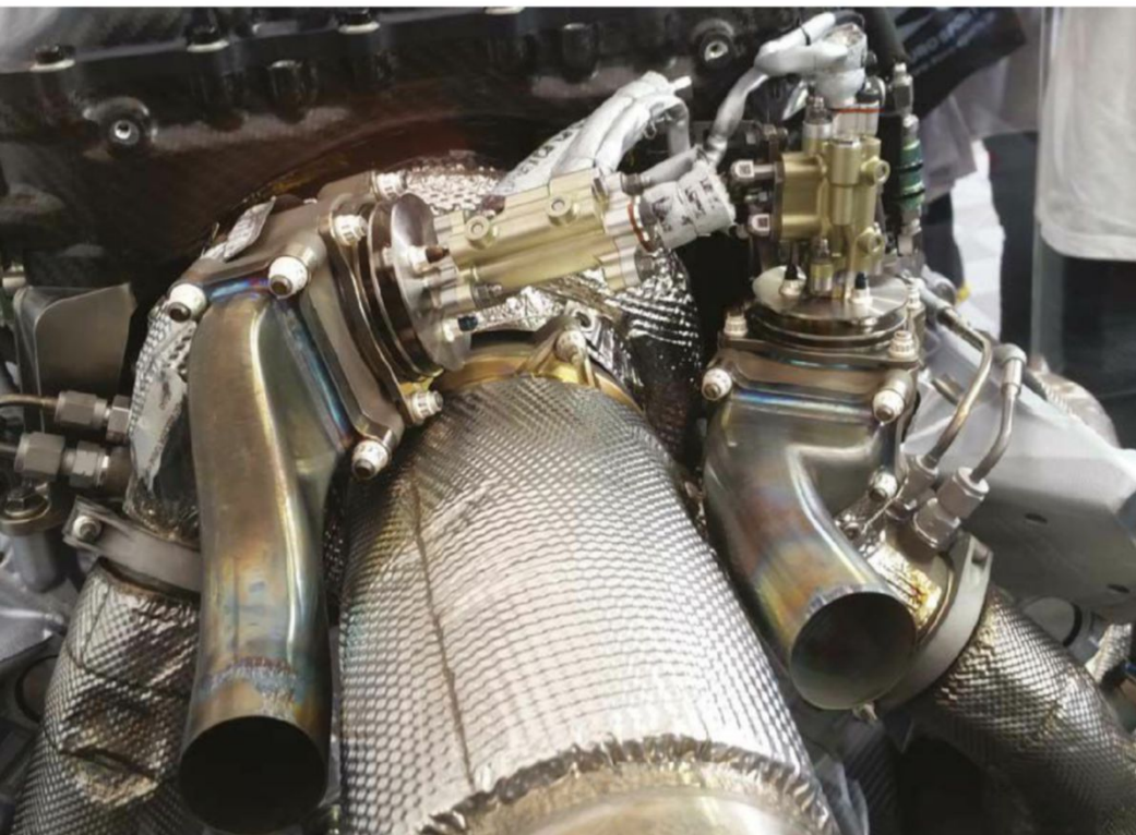
The turbine housing on the RA615H featured an integral wastegate, aimed at reducing PU size. This year a new rule was introduced in an attempt to make F1 engines louder, which forced Honda to change this layout on the RA616H (pictured)
