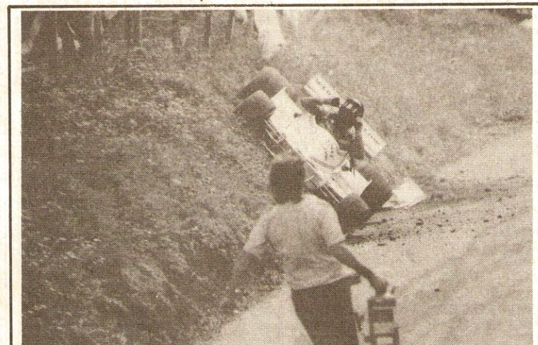
Subtle modifications to Alistair Douglas-Osborn's Waring & Gillow Pilbeam MP47 at Shelsley Walsh on July 11, endowed the machine with better balance than before so the team was able to crank off some rear wing in their quest for greater speed. On the first Top 10 run the car felt so good that ADO decided to approach the bottom Ess faster than before, only for the tail to slide wide onto the bank. The DFV-powered Pilbeam scaled the gradient, coming to rest at a 45 degree angle but, amazingly, repairs in the paddock allowed Alistair to make his second championship climb.
