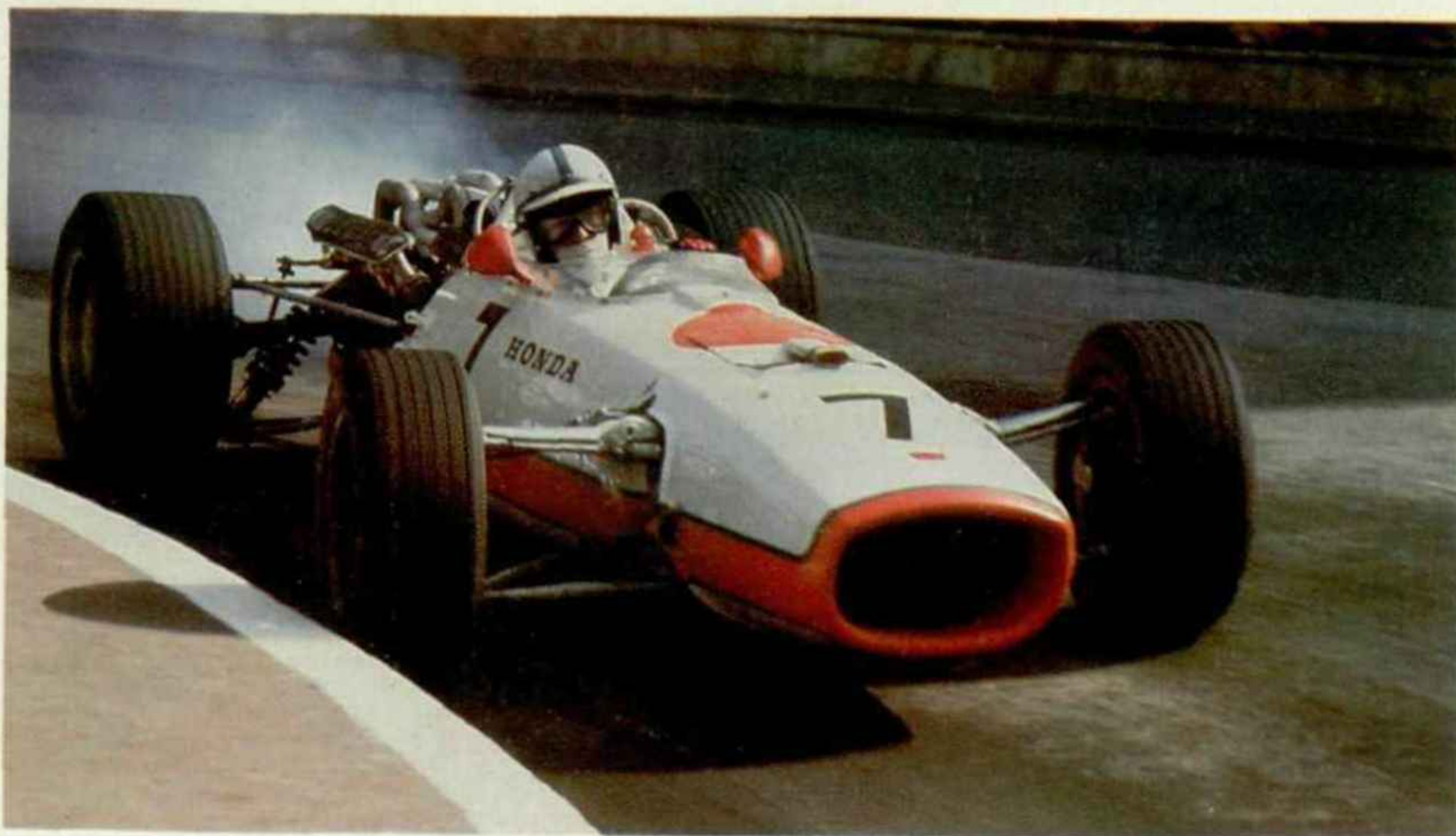
The V12 Honda engine campaigned in 1967 was too large and heavy to be competitive.
