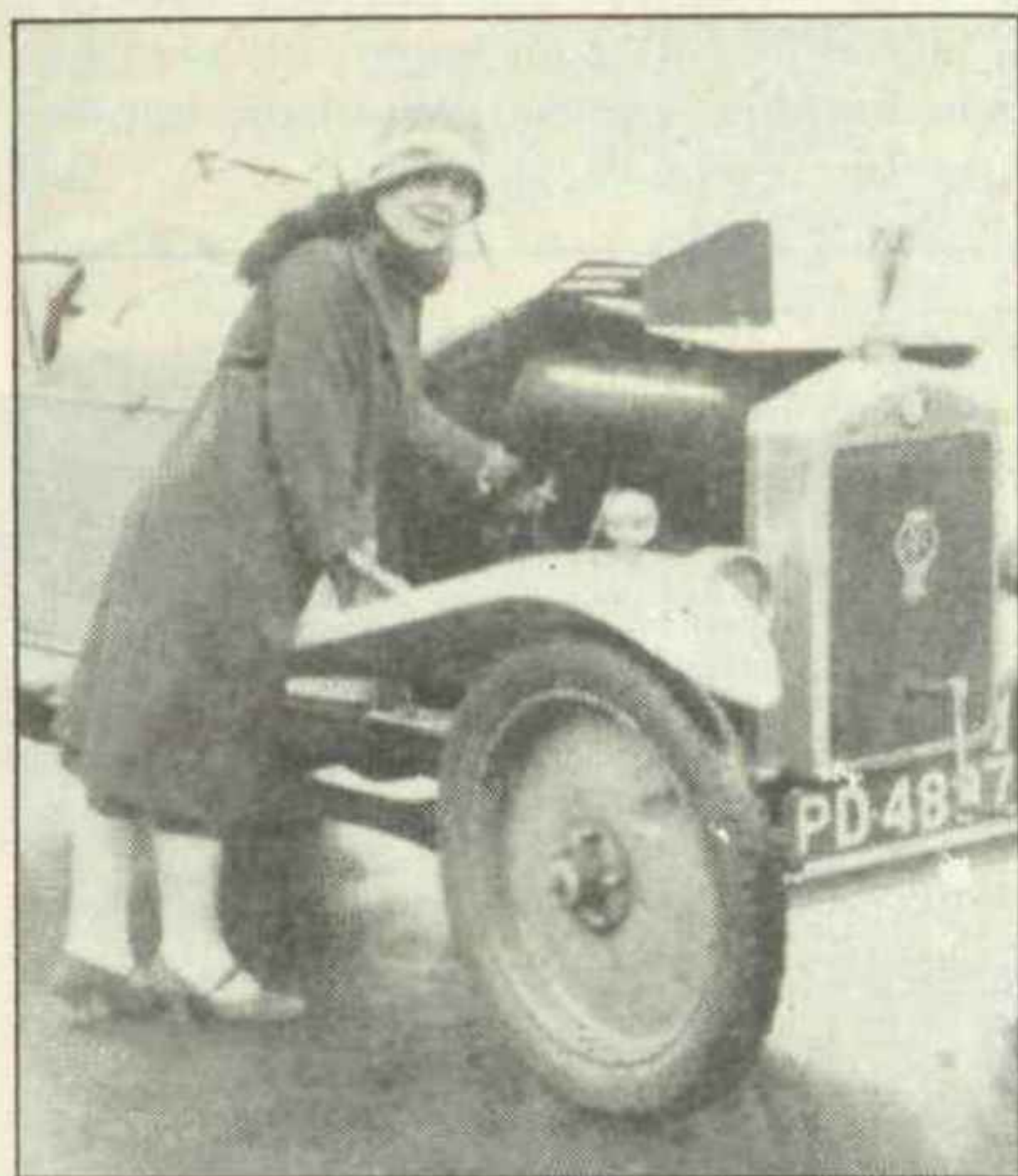
An ABC with the bonnet up, showing the seven gallon petrol tank that had to be filled through the radiator cap!
