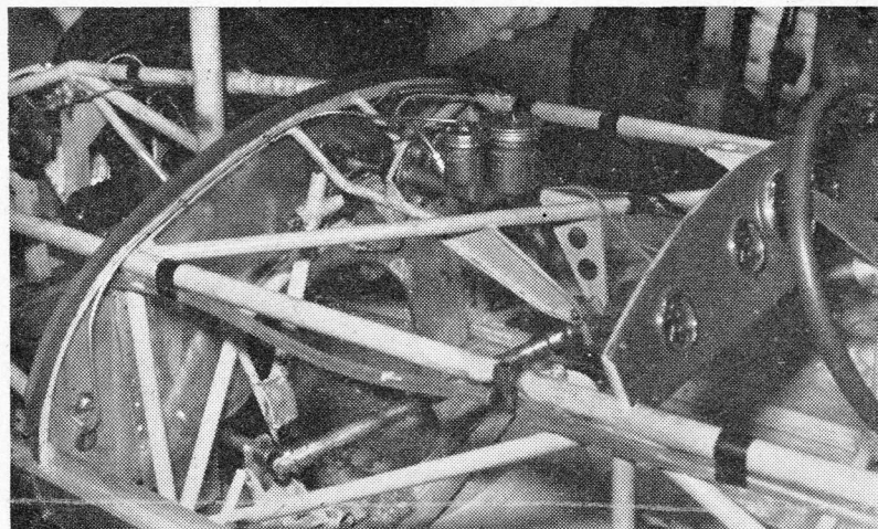
DETAIL of the space-frame chassis, showing how the steering column is cranked through two universal joints to bring it to the left of the cylinder block.
