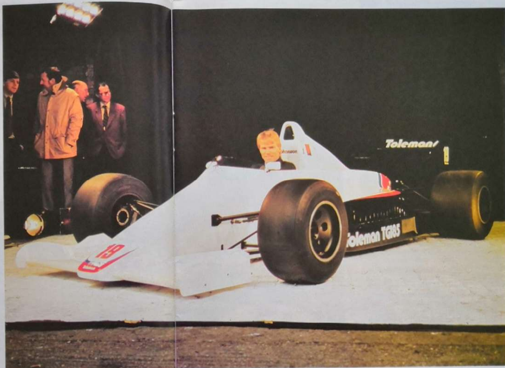
The TG185 is a thoroughly revised version of its predecessor, featuring an original rear wing and rear bodywork designed to cut turbulence caused by the rear wheels.
