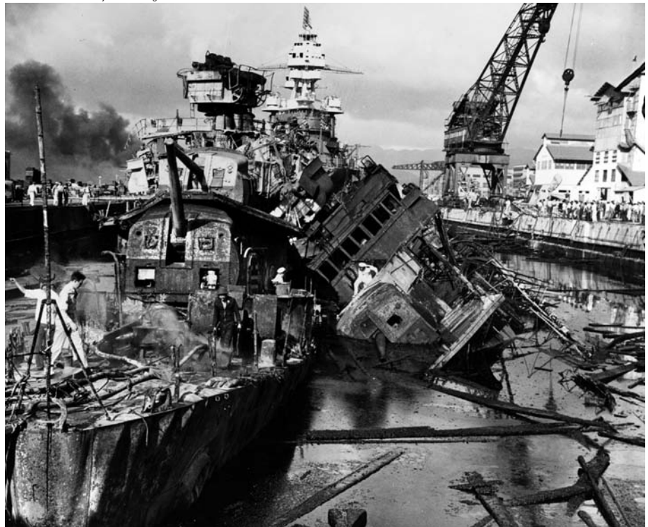
ABOVE: In this view of Drydock No. 1 following the attack, the destroyer Cassin has rolled over against the superstructure of the destroyer Downes . Japanese bomb hits and the resulting fires seriously damaged both ships. Looming behind the stricken destroyers, the USS Pennsylvania emerged from the attack with slight damage, the walls of the drydock having provided some protection. BELOW: The USS Pennsylvania sailed to Mare Island, California, where this photo was taken, and eventually reached Bremerton, Washington, to undergo repairs to damage sustained at Pearl Harbor and upgrades to some equipment.
