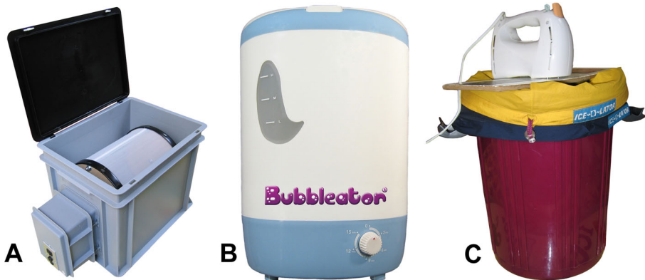
Fig. 22 Recent commercially available extraction systems for preparation of purified, high-THC concentrates of secretory glands starting with herbal material (leaves and flowers). a The “Pollinator ® ” is a dry sifting machine. Herbal material is placed in the revolving drum, which is perforated with 150 micron holes. Resin glands are expelled through the holes and collect in the box containing the drum. b The “Bubbleator ® ” is constructed like a small washing machine. Frozen herbal material is placed, along with ice-water, in a series of bags that are perforated with holes of decreasing size that permit the resin glands to be expelled. These in turn are placed in the device, which agitates the bags for a period, and then the separated resin glands are purified by additional sieving, and dried. This device takes advantage of the insolubility of the resin in water, and the brittleness of the glands when frozen. c The “Ice-O-Lator ® ” at right is a similar but simpler apparatus, in which an agitating device is placed on top of a bucket. Detailed operating instructions are available at various websites. These devices may be considered to be illegal drug paraphernalia in some countries. Photographs courtesy of Mila and Chimed Jansen of the Pollinator Company (note Jansen & Teris, 2002)
