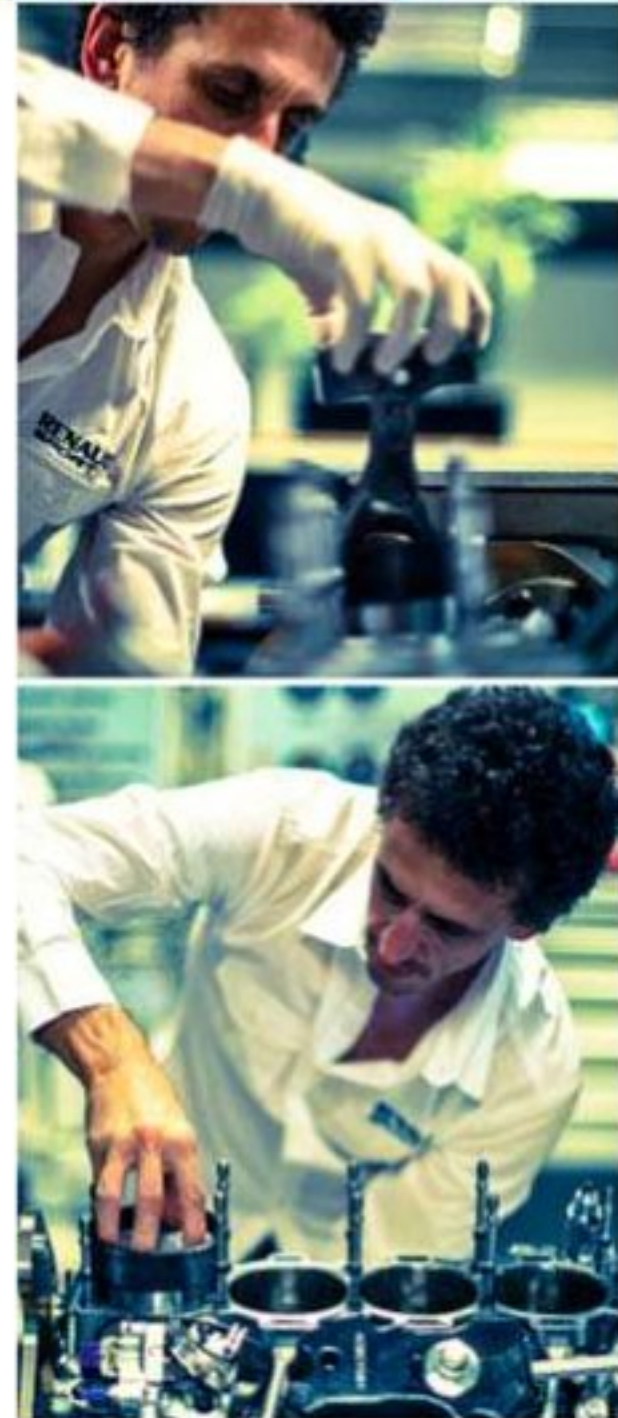
F1 Racing tries to fit the fiddly pistons into cylinder sleeves... and promptly cracks a ring
