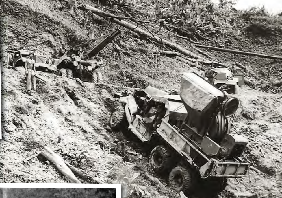
Above: A Diamond T 972 that slid off the road is being recovered by a Ward LaFrance or Kenworth M1 and a Diamond T 969 wrecker (US NARA).
