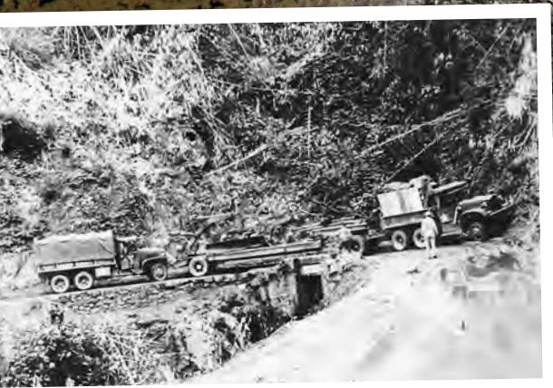
Above: A Diamond T 972 tipper and a GMC CCKW 353 combine their power to manoeuvre a trailer loaded with a grader near Bhamo, an often exhausting skill imposed on the drivers (US NARA).
