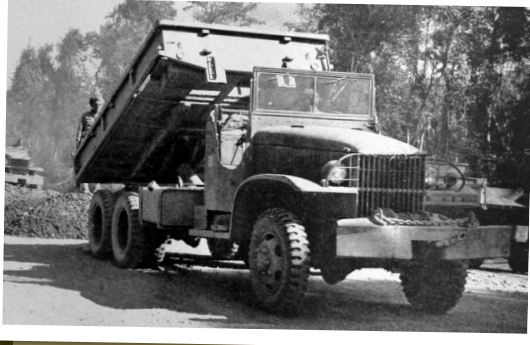
Above: Gravel laid down by a GMC CCKW 353 dump truck (1880th Aviation Engineer Battalion). Top: Shooting the Ledo airstrip with asphalt was a sordid task under the boiling rays of the sun (1880th Aviation Engineer Battalion). Top right: One of the advertisements published by Caterpillar during the war to pay homage to the Ledo Road builders, referring to its HQ in Peoria, Illinois (1880th Aviation Engineer Battalion).
