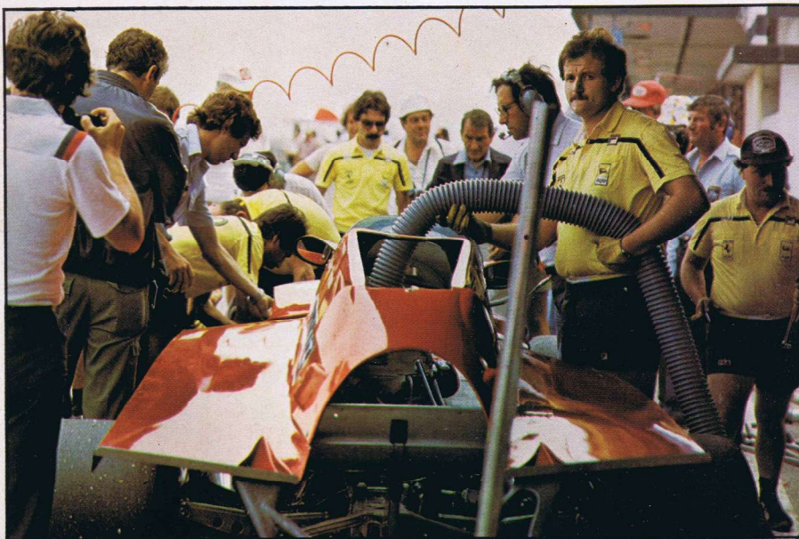
Ferrari's turbo gets a blast of cold air to cool it.
